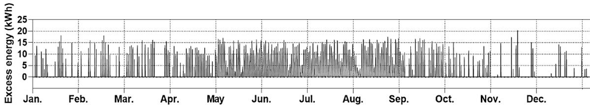
**Figure 6.** Yearly excess energy produced from cucumber-tomato greenhouse to provide energy for pepper greenhouse
