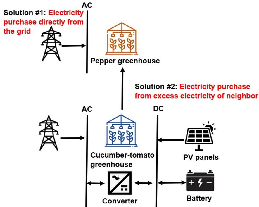
**Figure 3.** Schematic diagram of energy trading generation configuration
