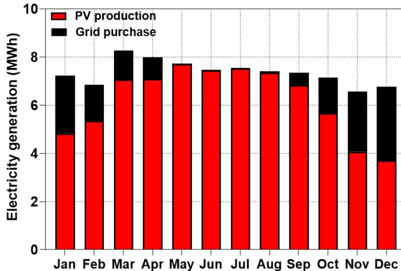
**Figure 5.** Energy generation profile of the optimal solution for cucumber-tomato greenhouse
