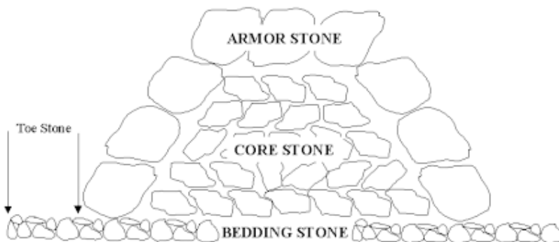
Figure 7 Typical cross-section of a rubble mound breakwater.
