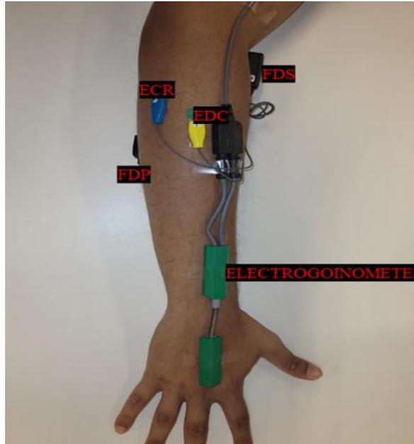
*Figure 8: Insertion Area for Extensor and Flexor Muscles of the Forearm*
