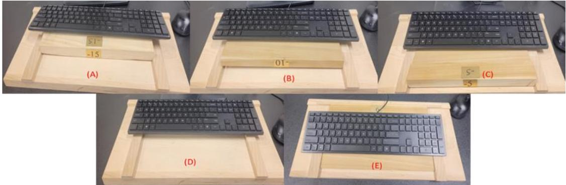
Figure 3: Portable Wooden Stand for (A)  $-15^\circ$ , (B)  $-10^\circ$ , (C)  $-5^\circ$ , (D)  $0^\circ$  and (E)  $6^\circ$  respectively
