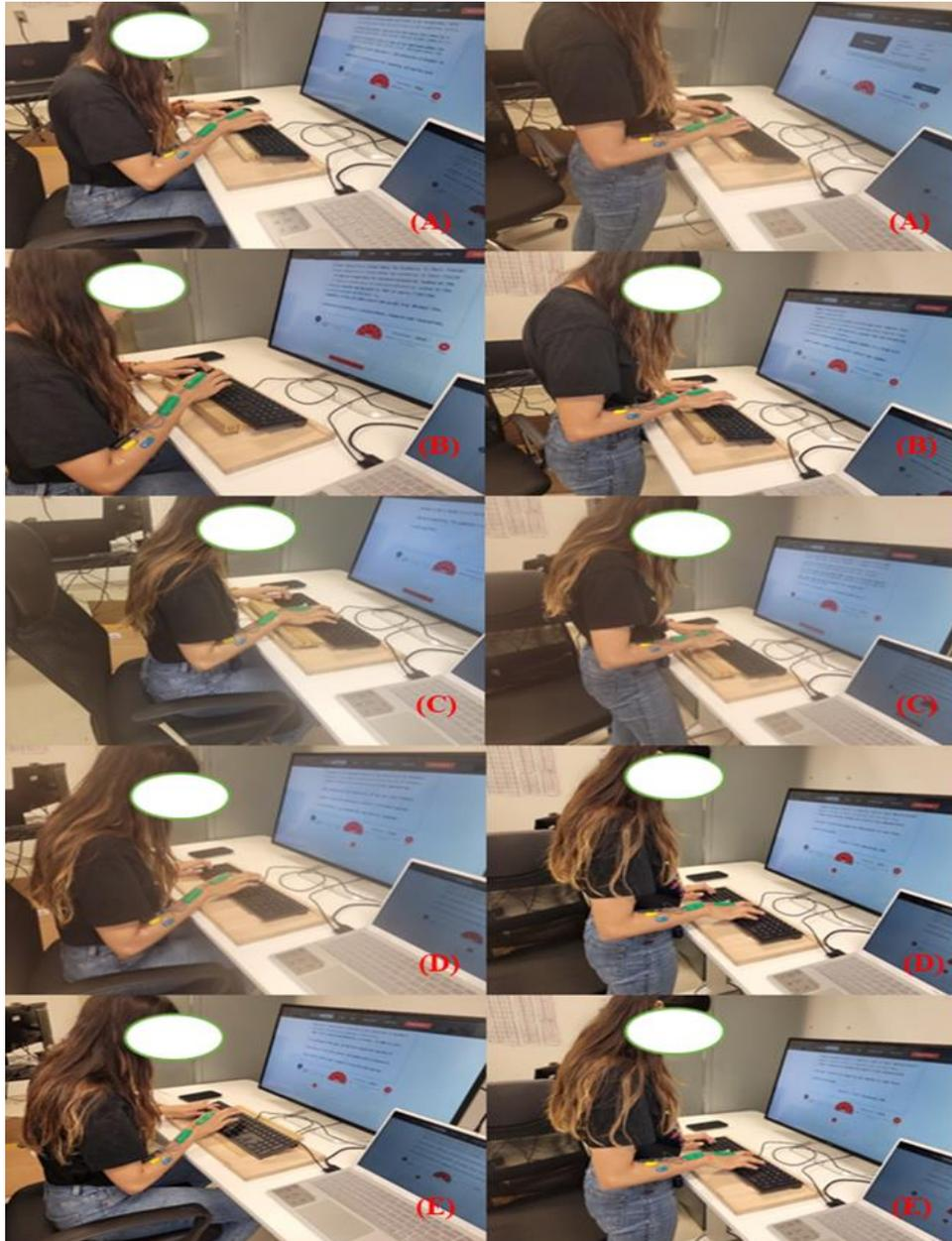
*Figure 7: Participant Typing on (A)  $-15^\circ$ , (B)  $-10^\circ$ , (C)  $-5^\circ$ , (D)  $0^\circ$  and (E)  $6^\circ$  for the sitting and standing positions respectively.*
