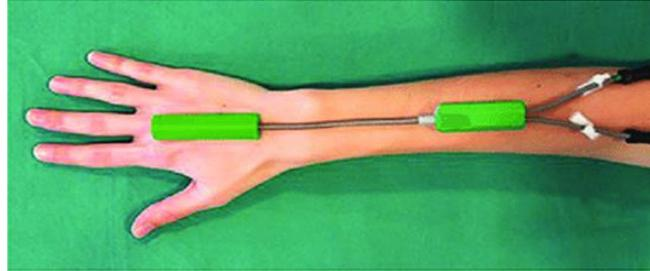
*Figure 6: Placement of goniometer (Image source: (PDF) Ergonomics in Laparoscopic Surgery (researchgate.net))*
