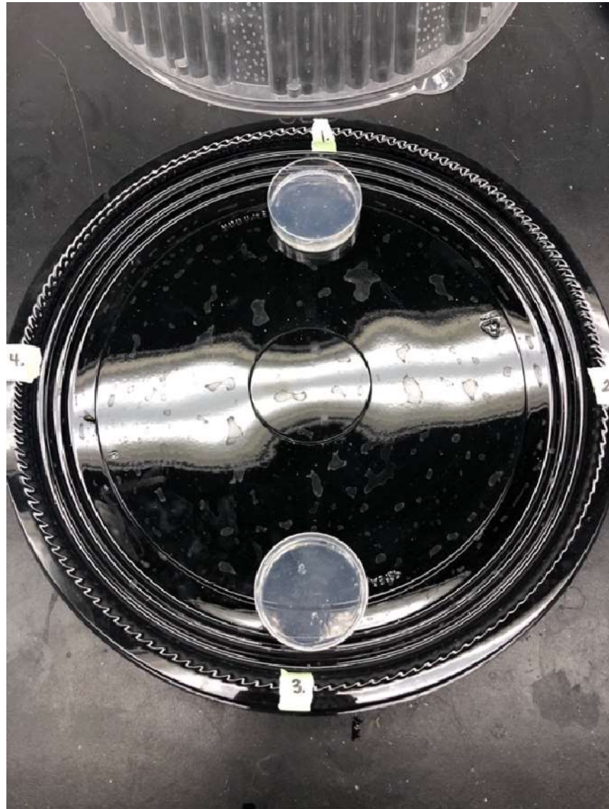
Figure 3.2. Open Experimental Arena. An image taken of the arena with two petri dishes containing agar, placed in randomly assigned sections. Quadrants are labeled with numbers assigned 1-4 according to their position. The lid to this arena is removed but visible at the top of this image.
