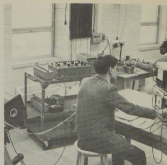
Facilities are available for precision measurement of magnetic and electrical properties, Heat treatment and Metallography. In the foreground of the picture is the coercimeter, in the background the measurement of permeability is being carried out.
