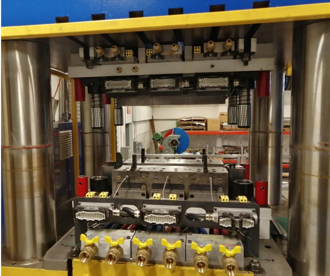
Figure 39 - Hot stamping channel die (front view).
