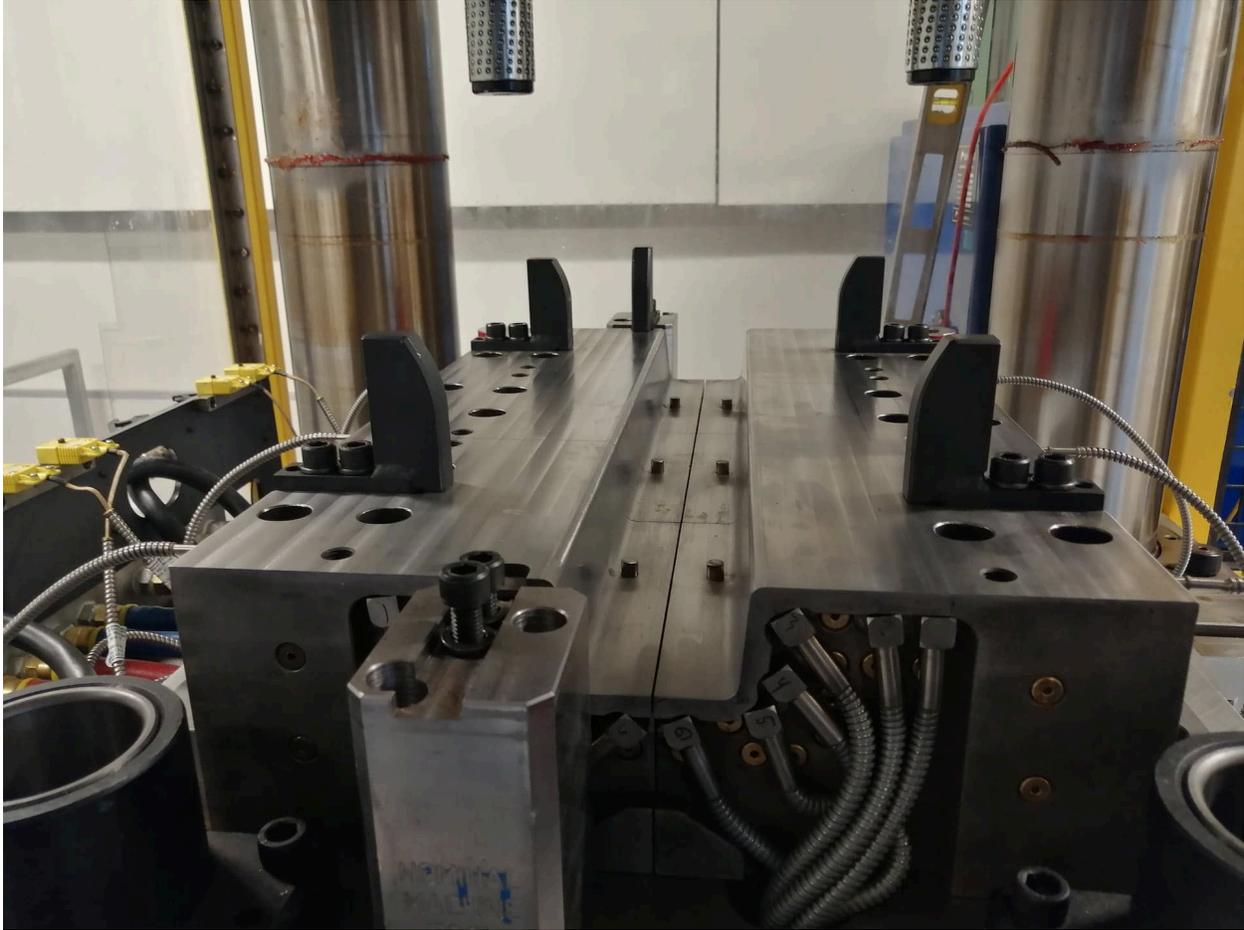
Figure 40 - Hot stamping channel die (side view).
