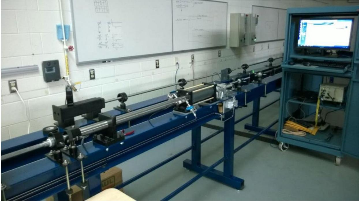
Figure 33 - Split Hopkinson pressure bar testing setup.
