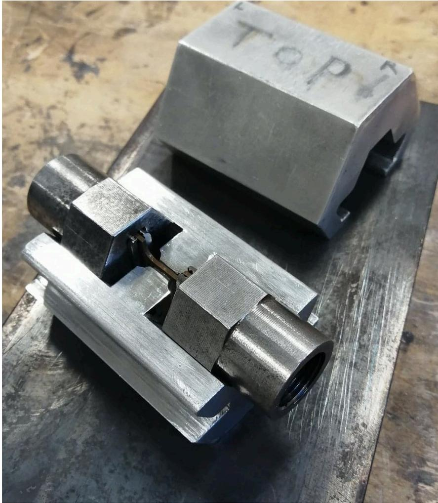
Figure 36 - Split Hopkinson specimen mounting fixture.
