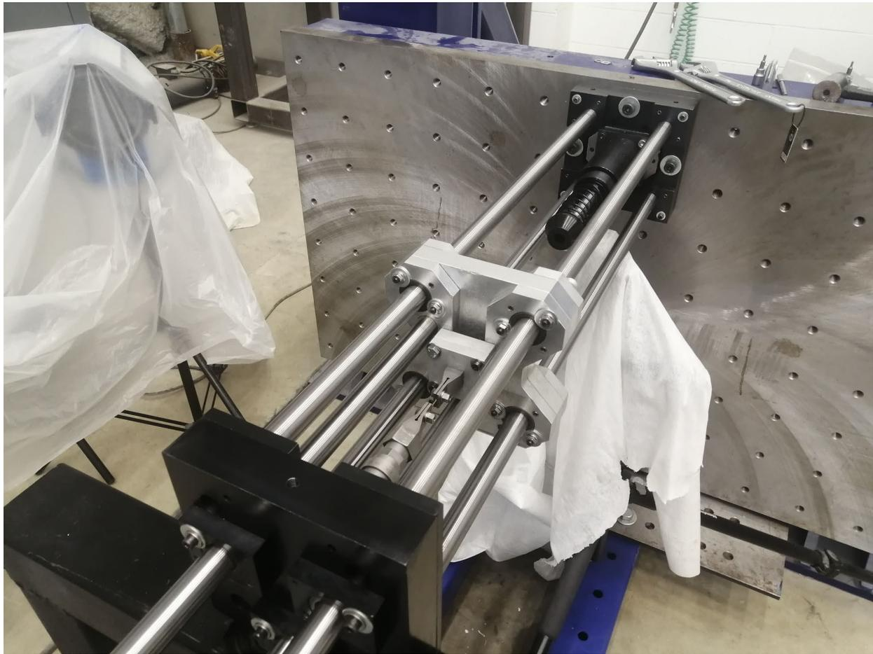
Figure 29 - Intermediate rate tensile testing apparatus with mini dogbone specimen.
