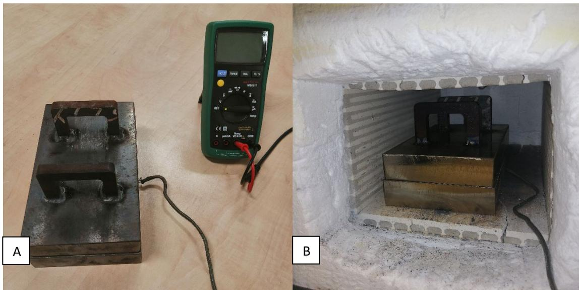
Figure 23 - a) H13 quenching dies with K-type thermocouple. b) Quenching furnace.
