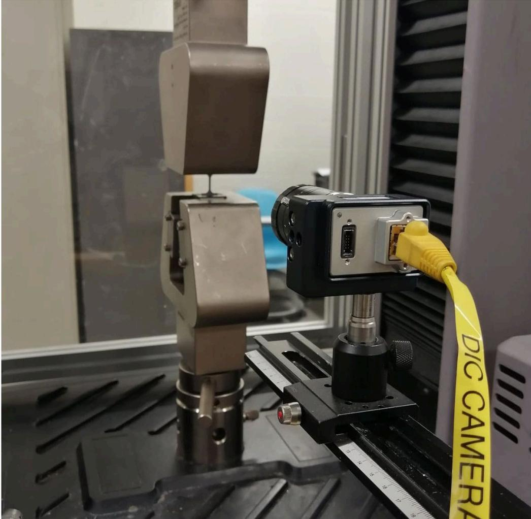
Figure 28 - Quasi-static tensile testing with DIC camera.
