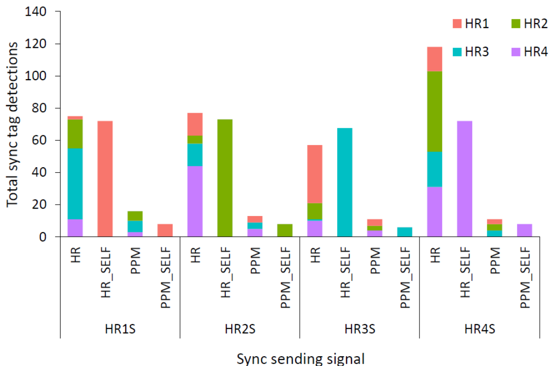
Figure 4.7 Total number of detections of internal sync tags (HR transmission rate = 25-45 s, PPM transmission rate = 270-330 s; 147 dB) aggregated across the 36 min study period. Number of detections displayed as a stacked bar for each signal type. Detections of surrounding sync tags are logged as either “HR” or “PPM” detections, and detections of internal sync tags are logged as either “HR_SELF” or “PPM_SELF”. Reflections are included in this visualization and are identified according to listening receiver (e.g., HR4) decoding its own sync tag (e.g., HR4S) as a “HR” rather than “HR_SELF” detection. Expected number of sync detections: 7 (range 6 - 8) PPM detections per sync tag, and 61 (range 48 - 86) HR PPM detections per sync tag.
