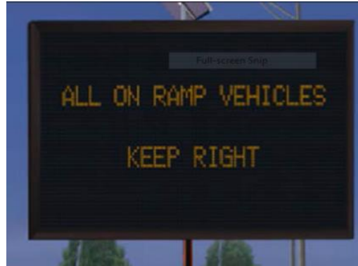
FIGURE 2-4. VARIABLE MESSAGE SIGN FOR RAMP VEHICLES AT TOLL PLAZA (SOURCE: SAAD ET AL., 2019)
