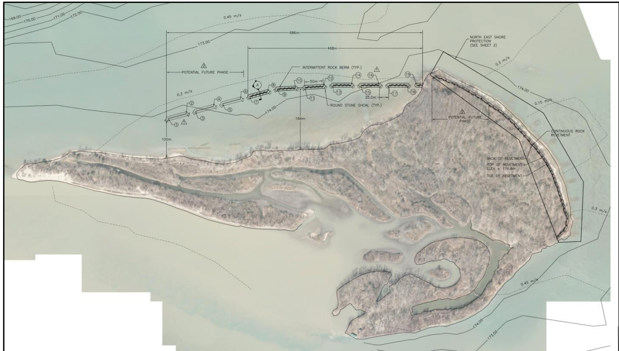
Figure 9: Engineering plans showing location and spacing of offshore berms (DRCC Annual Report, 2021-2022).
