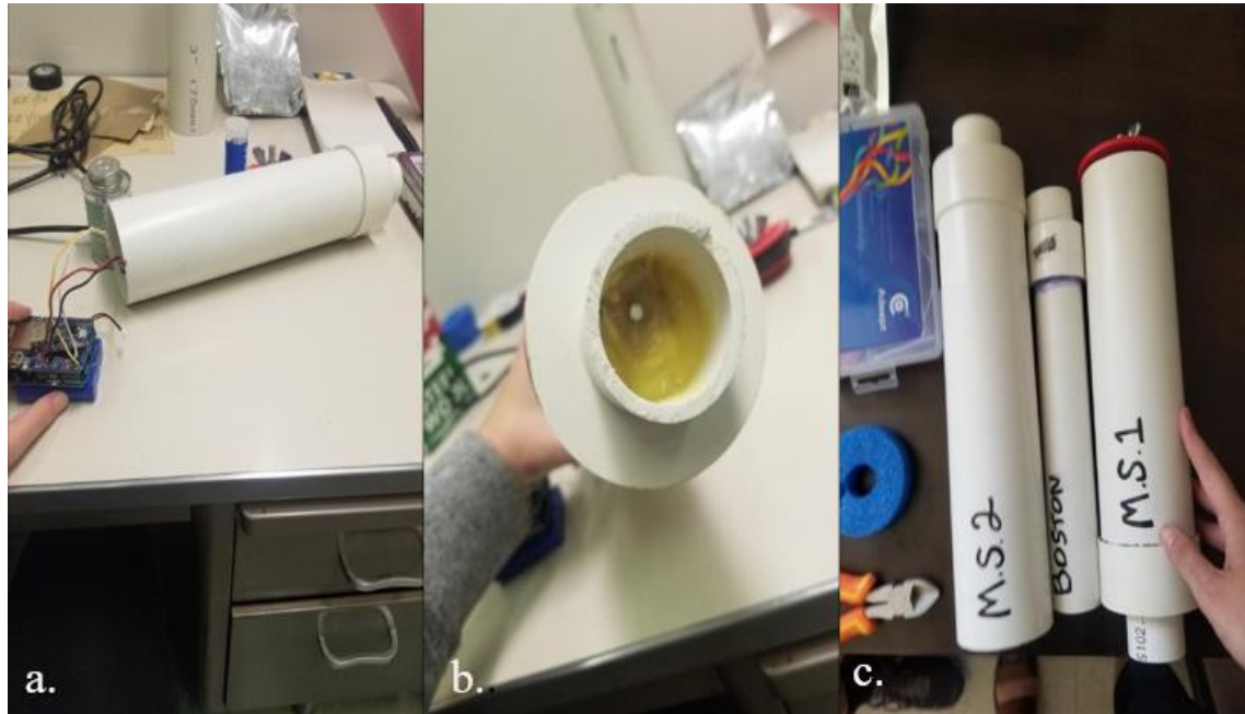
Figure 11: a. Wired Arduino kit soldered to the exposed sensor board. b: Top of the housing showing the actual sensor set in epoxy. c. Final model used for testing alongside prototypes.
