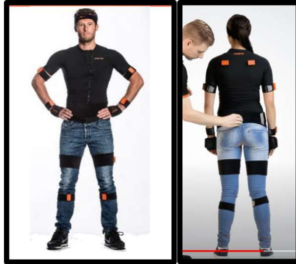
Figure 2: Anterior (left) and posterior (right) views of two individuals fully instrumented with all 17 IMUs. For this study, only the IMUs above the pelvis were used (Xsens, 2021; Xsens, 2016).
