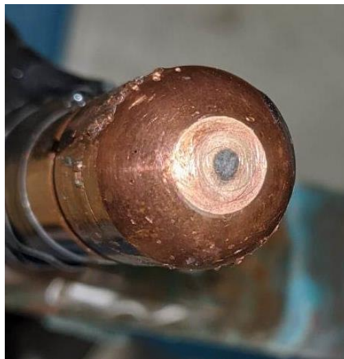
Figure 5-6 A graph showing the comparison between the different measuring methods for 20 flat cap geometry centered welds. It is observed that all the phased array measurements fall within uncertainty of the other measuring methods provided. The resulting cap used to conduct these 20 welds is shown below where the spot weld is concentrated in the center of the scanning axis.
