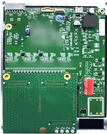
Figure 4-5 An image of the AOS acquisition system board. 19
