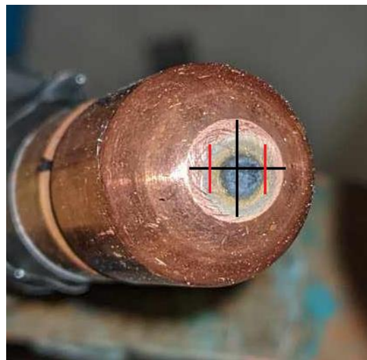
Figure 5-11 Cylindrical cap geometry off-centered welds are shown above. All 20 welds were conducted using the cap shown below. With only a slight deviation from the center, some welds were still entirely contained within the PA imaging region which showed agreement with other measuring methods. For welds that exceeded the imaging region, agreement was still shown for the part of the nugget exposed within the imaging region.
