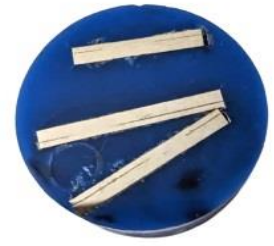
Figure 2-5 A weld cut cross section on the left imaged under an optical microscope where the regions of fused metal can be observed. On the right an image of where three cross sectional cuts are polished and await to be etched for observation.
