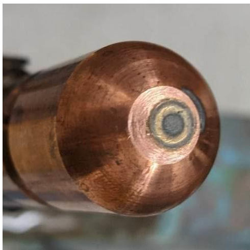
Figure 5-7 20 Spherical cap geometry centered welds are provided above. All the phased array measurements fall within uncertainty of the other measuring methods provided. The cap used for these welds are shown to have residue concentrated in the center which agree with the symmetrical scans observed using the phased array.
