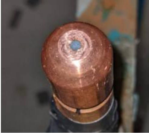
Figure 5-14 Copper cap used to weld a set of centered cylindrical. The welds can be seen to be centered, producing centered M-scans such as the one shown in figure 5.15.
