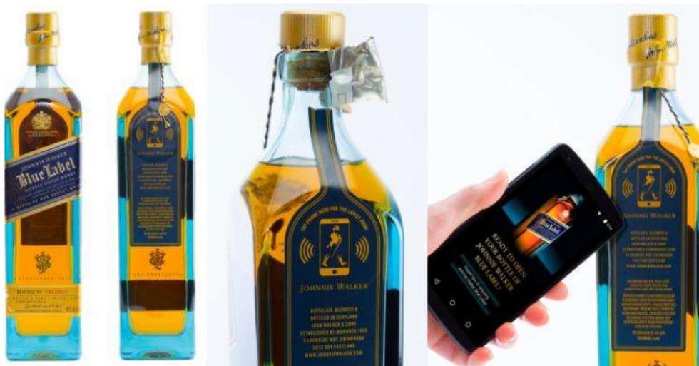
**Figure 1.1** Johnnie Walker Blue Label with incorporated electronic tag that is connected to the IoT a) shows the seamless integration into the product, b) the electrical component becomes exposed once opening the bottle, c) NFC lets consumers interact with the product using NFC-enabled smartphones.
