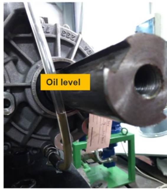
FIGURE 6.7: EDM oil level measure : It is performed by means of a pipe connected to the housing, that allow the visualization of the oil level and permits the measure of it.
