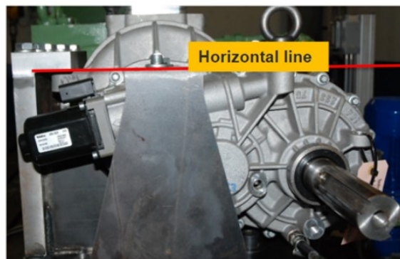
FIGURE 6.8: Inclination of the EDM while mounted on the test rig : an important parameter to be known to evaluate the level of immersion of each gear in the oil.
