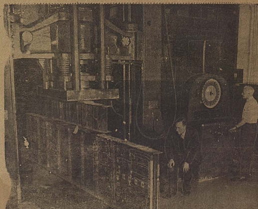
WITH A TOUCH OF THE FINGER, pressures in excess of 300 tons can be exerted by this new $20,000 universal testing machine recently instal- led in Montreal's McGill University. The machine, a gift to the university by an anonymous donor, will furnish exact data on stress and strain
