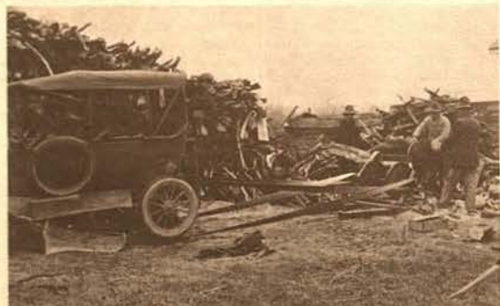
MODEL T POWER FOR A BUZZ SAW was only one of the many unusual uses to which owners put the versatile Model T. So much so that on one occasion Ford of Canada felt compelled to warn its customers "not to expect the impossible" from the car.
