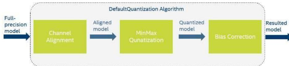
Figure 7: *DefaultQuantization* Algorithm [30]
