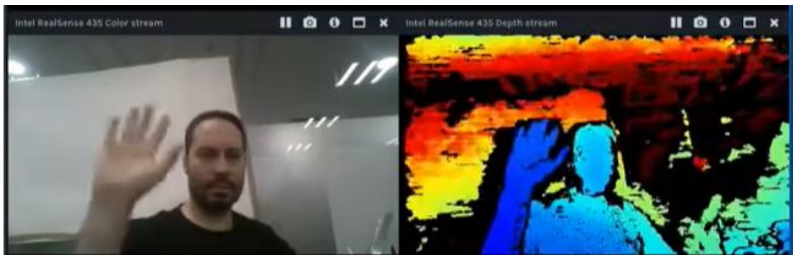
Figure B-2. An illustrative example of the D435if's output.
