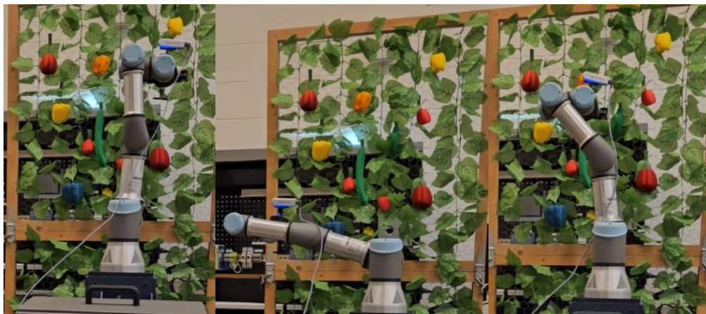
Figure 3-8. Camera movement at different angles and directions
