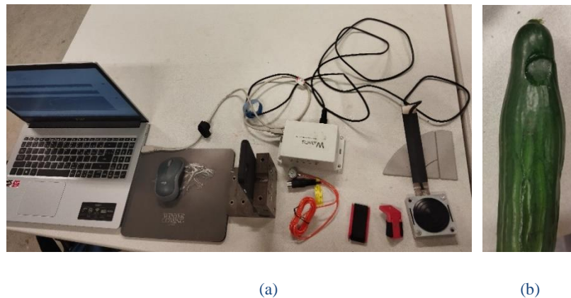
Figure 3-11. a. Experimental setup to find the peak forces that each cucumber can tolerate and a damage cucumber after applying force, b. Damaged cucumber after applying force on its surface
