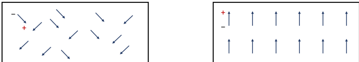
Figure 11. Schematic depiction illustrating dipole displacement resulting from the application of a direct current DC field.
