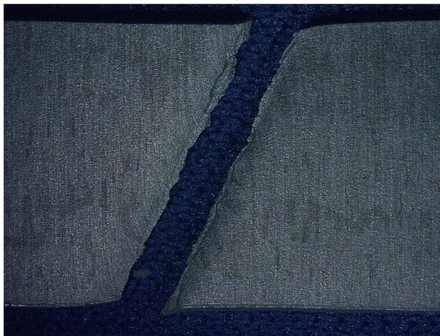
**Figure A.10** Tensile sample fractured at temperature of 25°C
