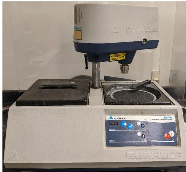
**Figure 3.3** Buehler EcoMet metallographic polishing machine.
