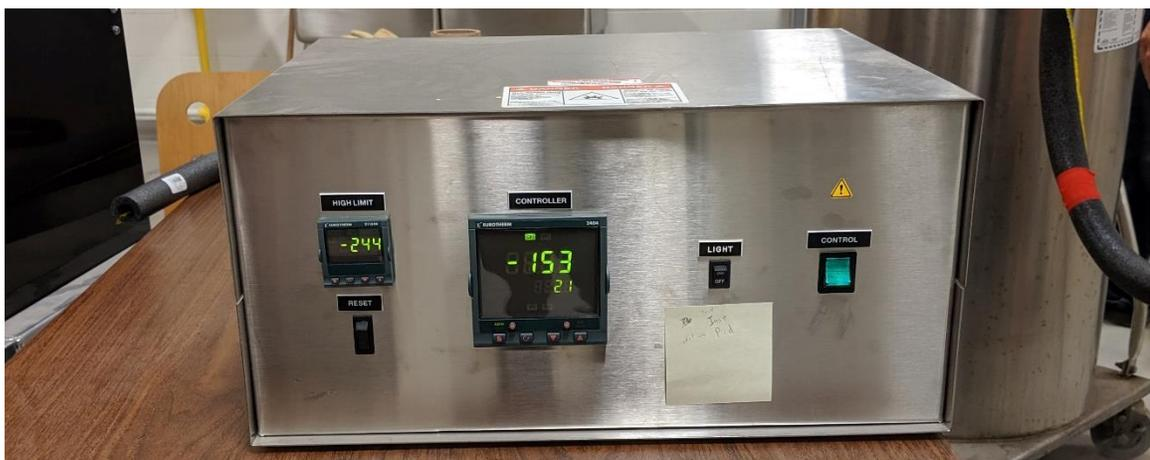
**Figure 3.16** Temperature control unit attached to the MTS tensile machine.
