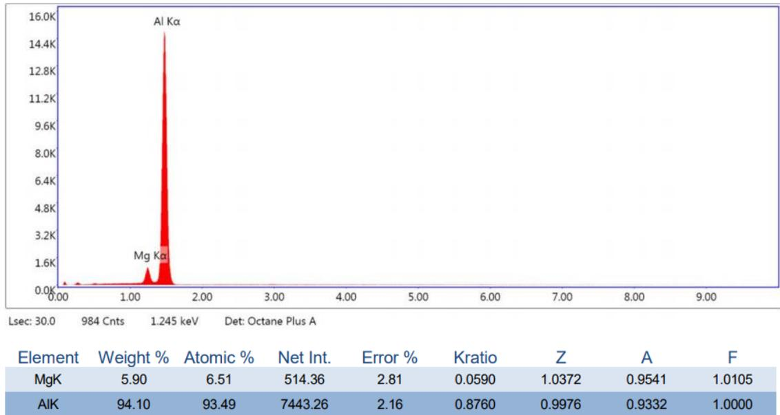
**Figure 4.7** Element distribution graph obtained from EDS analysis of spot 2
