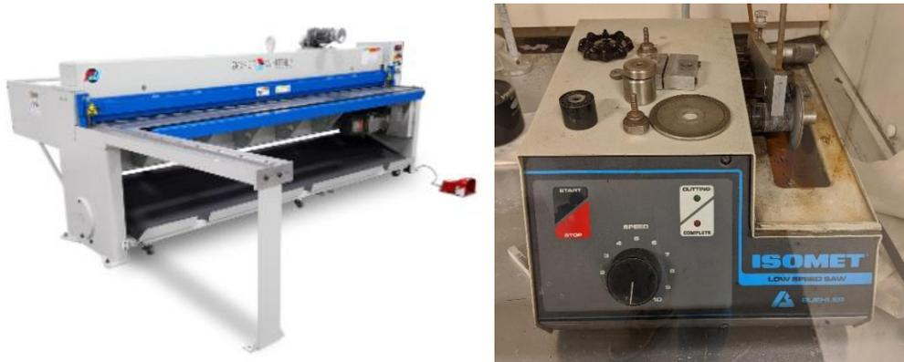
**Figure 3.1** Image of the (a) sheet metal shearing machine [1] and (b) low speed diamond saw cutter used to AA5182-O aluminum alloy samples for grinding and polishing.
