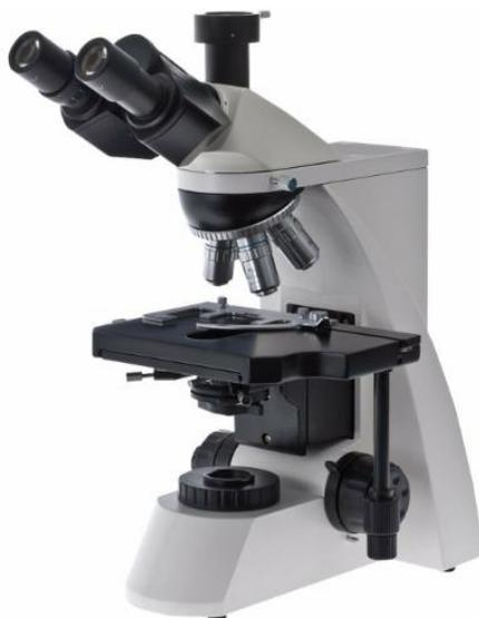
**Figure 3.6** Omano OM159T (40x-1,000x ) Trinocular Compound Microscope [6]
