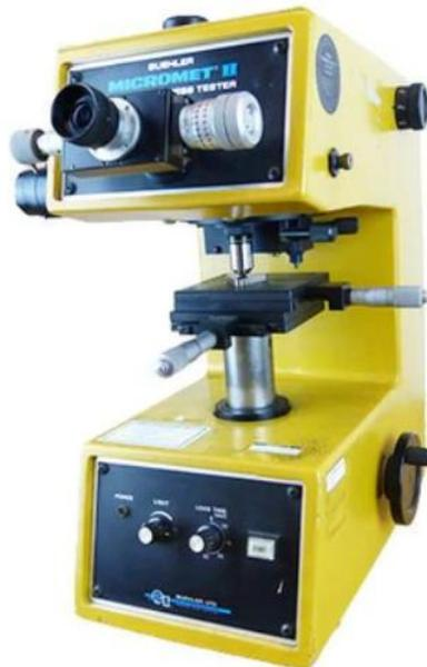
**Figure 3.5** Buehler Micromet II model MHT-1B Micro Hardness Tester [4].
