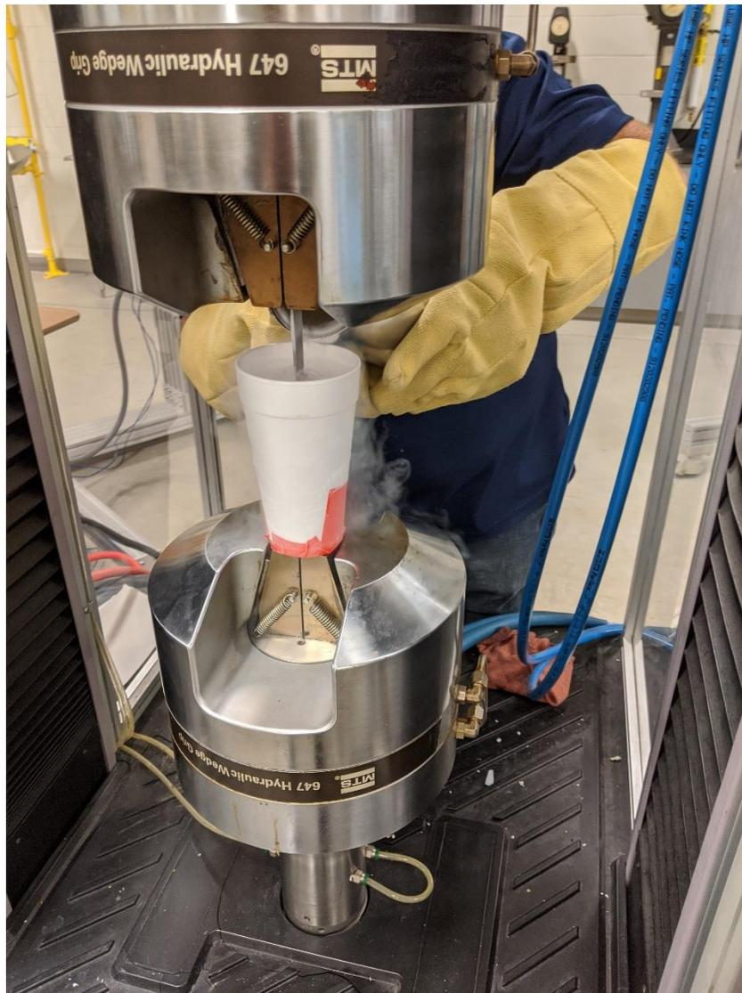
**Figure 3.17** Set-up for samples tested at  $-196^{\circ}\text{C}$  tensile testing temperature.
