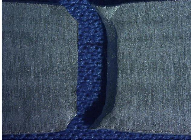
**Figure A.9** Tensile sample fractured at temperature of 120°C
