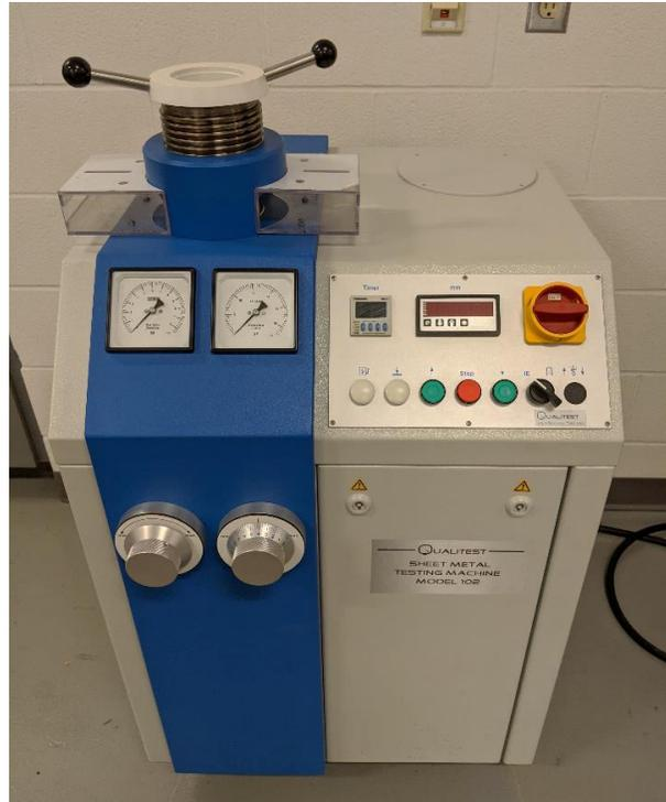
**Figure 3.18** Erichsen sheet metal testing machine model 102.
