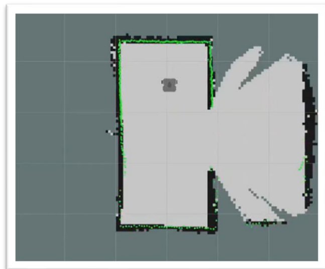
Figure 34: RViz Map of Test 2 – Driving alongside a mirror, Position C – Top of the experimental setup
