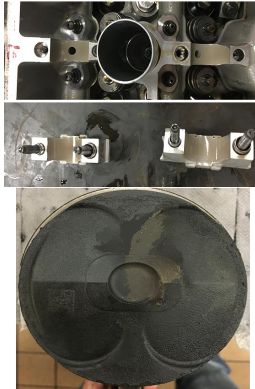
Figure 9-9. EJPO coated camshaft bores and pistons after vehicle durability test
