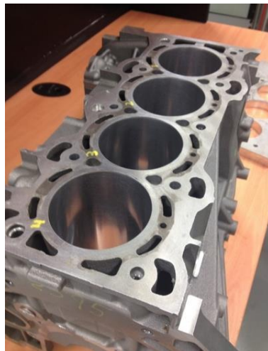
Figure 4-1. Flex brush honed linerless 2.0 L aluminum engine block
