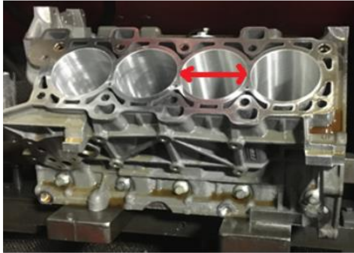
Figure 8-12. The cylinder bridge deformed when the honing pressure was applied using two stones honing head
