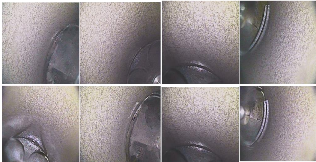
Figure 9-2. Cylinder bore images after Break-in test
