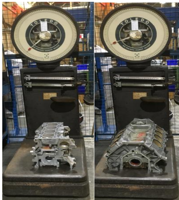
Figure 7. Weights of EJPO coated 2.0 L and 5.0 L engine blocks
