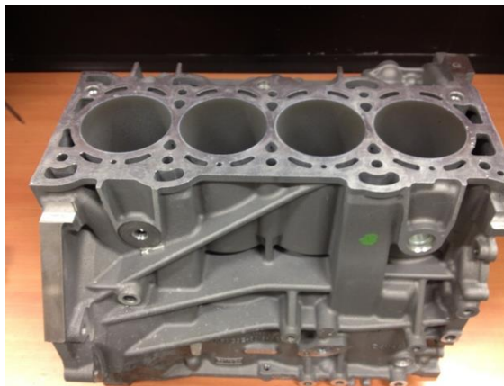
Figure 4-3. EJPO coated 2.0 L aluminum engine block with two kinds of coatings
