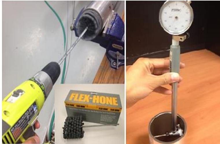
Figure 3-16. Flex brush honing and bore size measurement
