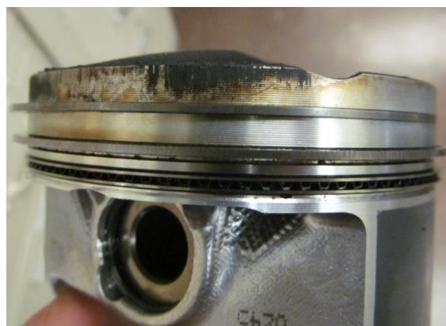
Figure 5-13. Scuffed cylinder one piston
