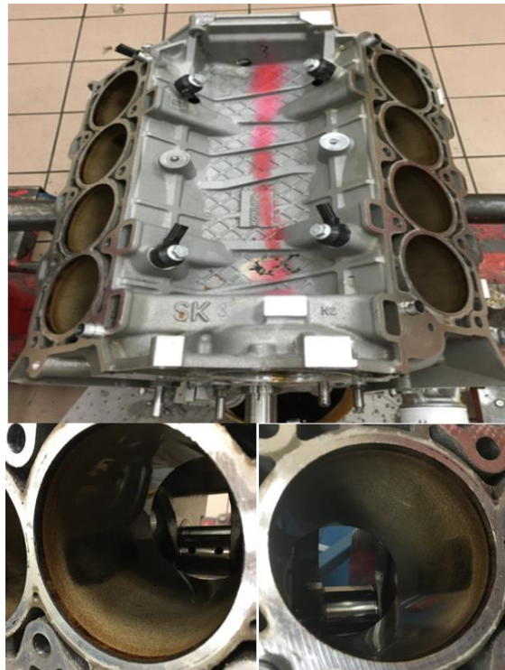
Figure 8-3. Cylinder bores with black marks after test
