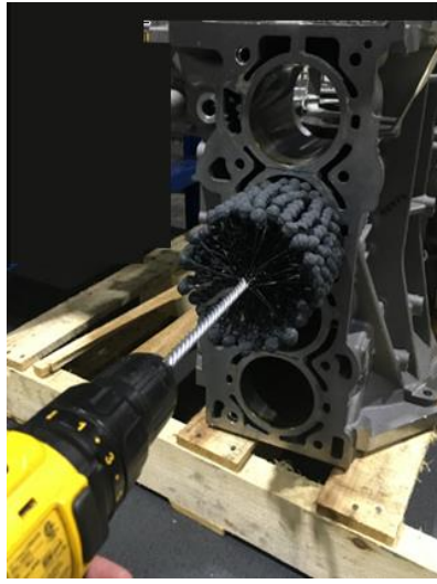
Figure 4-12. Flex brush honing process
