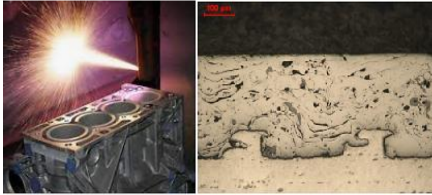
Figure 2-5. PTWA coating spray and coating cross section view [9]
