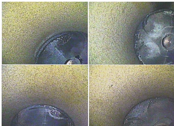
Figure 5-6. Cylinder borescope pictures after Break-in test
