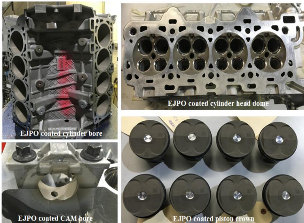
Figure 6-18. Honed EJPO coated engine block and EJPO coated camshaft bore, cylinder head dome, and piston crown
