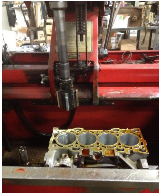
Figure 5-1. Diamond stone honing process
