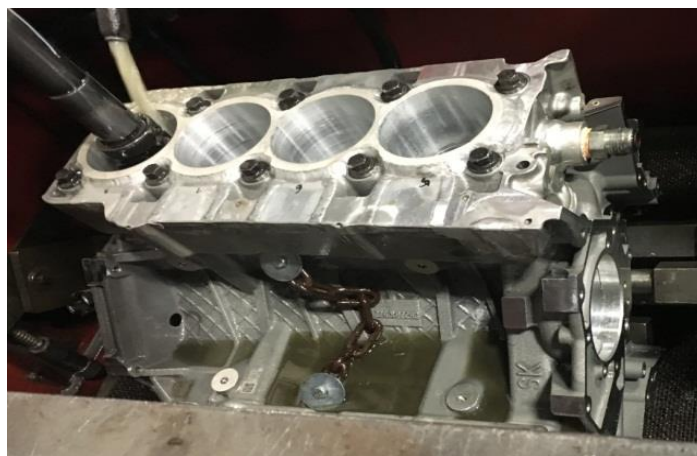
Figure 8-10. Honing process with torque plates installed
