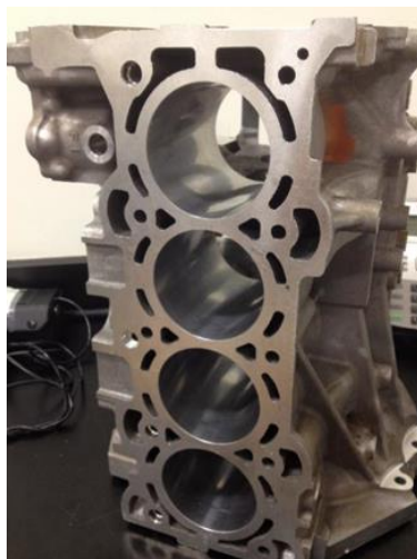
Figure 4-9. Flex brush honed aluminum engine cylinder bore
