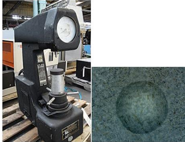
Figure 3-3. Rockwell hardness tester and SEM image of dented coating
