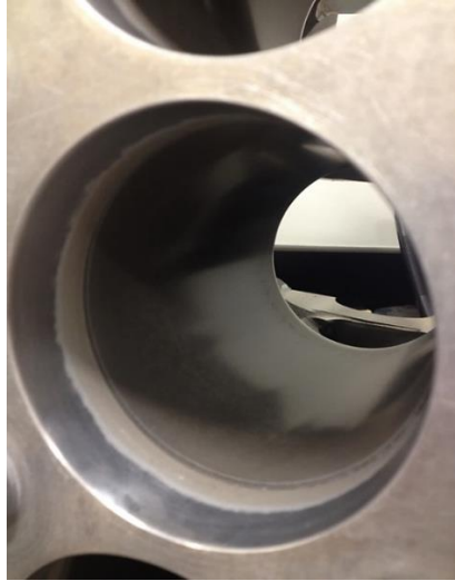
Figure 4-4. Flex brush honed cylinder bore
