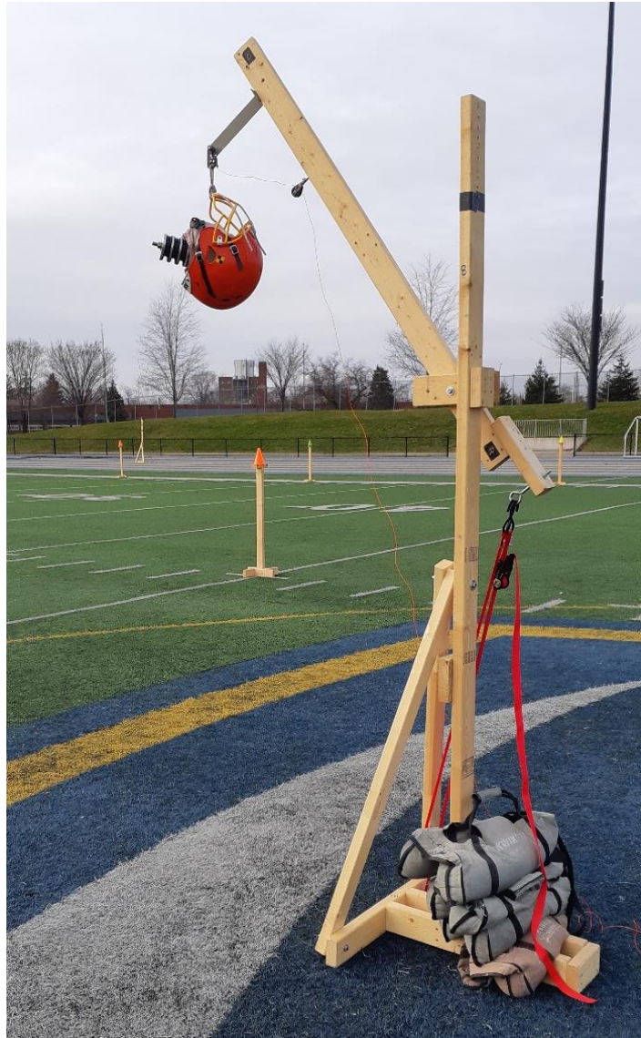
Figure 4.2 – Apparatus set-up for free fall drop test of helmeted anthropomorphic test device (Hybrid III 50th percentile male) head and neck assembly.
