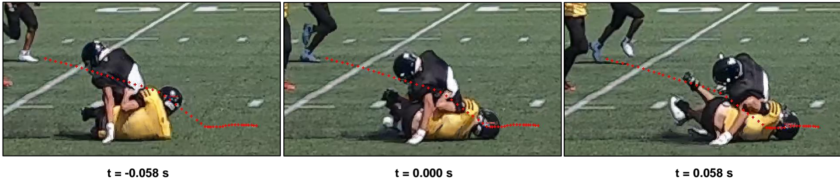
Figure 2.2 – Example of a 2D helmet track using the motion analysis software for a single-camera view along the side line. The series of images shows the frame of helmet-to-ground (H2G) impact ( t = 0.000 \text{ s} ) and the frames \pm 0.058 \text{ s} pre- and post-impact. Appendix A provides further detail of the video analysis procedures used to quantify the 3D helmet motion for this example, such as additional pre-impact frames and the 2D track corresponding to a second camera view.
