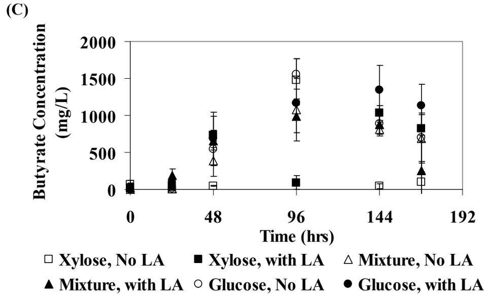
**Figure 5.11 Volatile fatty acid production for cultures at pH 5.6 and fed 2,000 mg/L LA plus 5,000 mg/L sugars (glucose, xylose and glucose plus xylose). Sugars injected on t = 0 and t = 96 hrs (the data points represent triplicate samples; errors are indicated using the standard deviation). (A) Acetate Production, (B) Propionate Production, and (C) Butyrate Production.**
