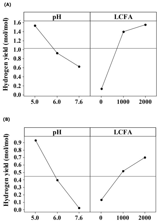
**Figure 4.6 Factorial plots of hydrogen yield in a two factor, three level FFD, (A) LA main effects plot (B) OA main effects plot**
