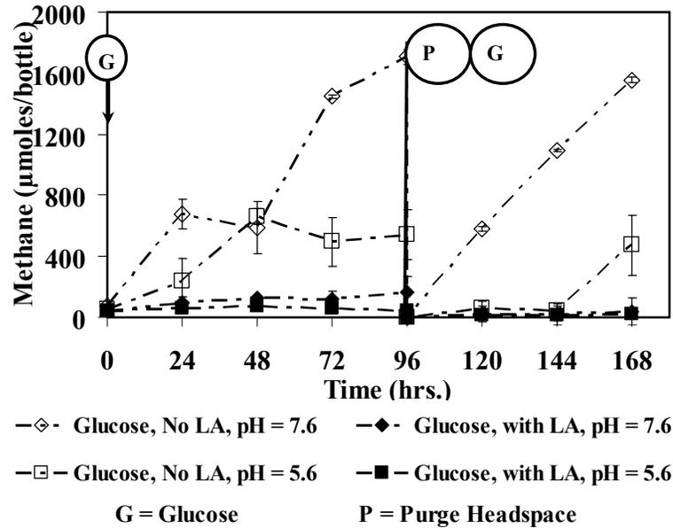
**Figure 5.7 Gas production for glucose (5,000 mg/L) degradation under different pH conditions in the presence of LA at 2,000 mg/L. Glucose injected at t = 0 and again after purging at t = 96 hrs (the data points represent triplicate samples; errors are indicated using the standard deviation). (A) Hydrogen production and (B) Methane production.**
