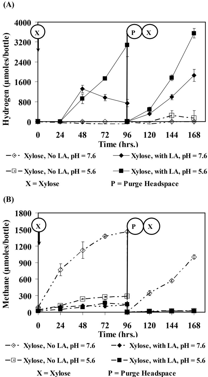
Figure 5.1 Gas production profiles for xylose (5,000 mg/L) degradation under different pH conditions in the presence of LA at 2,000 mg/L. Xylose injected at  $t = 0$  and again after purging at  $t = 96$  hrs (the data points represent triplicate samples; errors are indicated by the standard deviation). (A) Hydrogen production and (B) Methane production.
