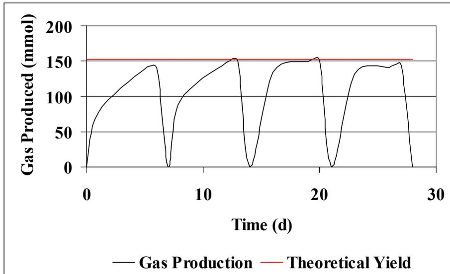
Figure 3.1 Gas production profile for Reactor B
