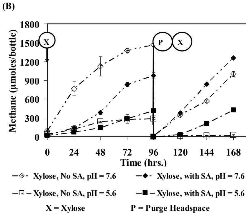
**Figure 5.4 Gas production profiles for xylose (5,000 mg/L) degradation under different pH conditions in the presence of SA at 2,000 mg/L. Xylose injected at  $t = 0$  and again after purging at  $t = 96$  hrs (the data points represent triplicate samples; errors are indicated by the standard deviation). (A) Hydrogen production and (B) Methane production.**
