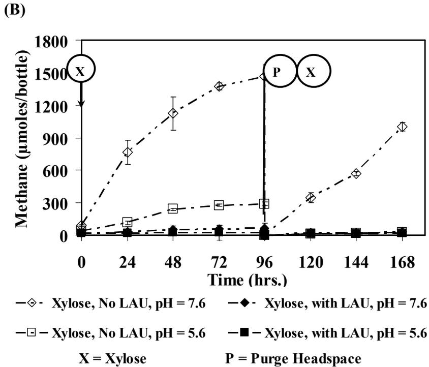
**Figure 5.3 Gas production profiles for xylose (5,000 mg/L) degradation under different pH conditions in the presence of LAU at 2,000 mg/L. Xylose injected at  $t = 0$  and again after purging at  $t = 96$  hrs (the data points represent triplicate samples; errors are indicated by the standard deviation). (A) Hydrogen production and (B) Methane production.**
