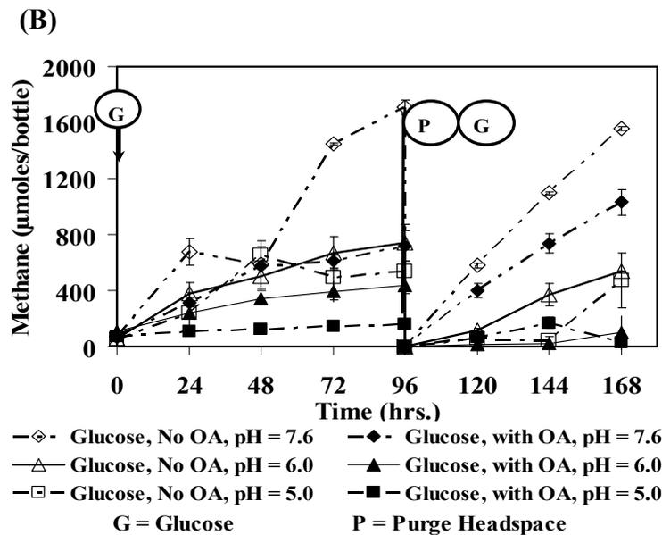
**Figure 4.5 Effect of pH on gas production in cultures receiving 1,000 mg/L OA and 5,000 mg/L glucose. Glucose addition and pH adjustment at  $t = 0$  and  $t = 96$  hrs (the data points represent triplicate samples; errors are indicated using the standard deviation). (A) Hydrogen Production, (B) Methane Production.**
