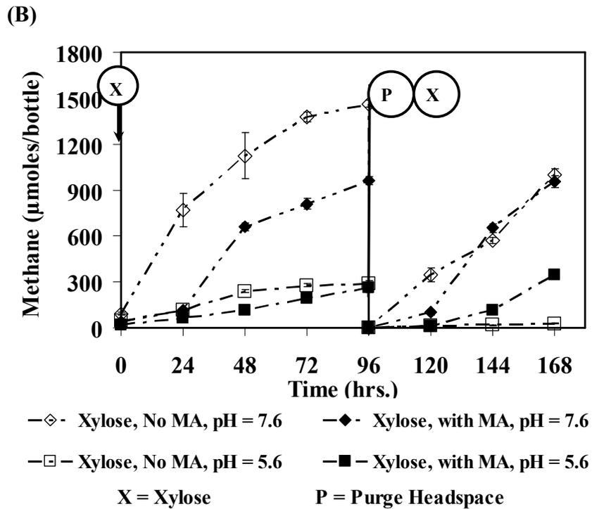
**Figure 5.6 Gas production profiles for xylose (5,000 mg/L) degradation under different pH conditions in the presence of MA at 2,000 mg/L. Xylose injected at  $t = 0$  and again after purging at  $t = 96$  hrs (the data points represent triplicate samples; errors are indicated by the standard deviation). (A) Hydrogen Production and (B) Methane Production.**
