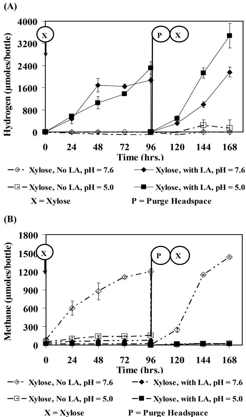
**Figure 5.8 Gas production for the degradation of a 25%/75% mixture of xylose plus glucose (5,000 mg/L) under different pH conditions in the presence of LA at 2,000 mg/L. Sugars injected at  $t = 0$  and  $t = 96$  hrs (the data points represent triplicate samples; errors are indicated using the standard deviation). (A) Hydrogen production and (B) Methane production.**
