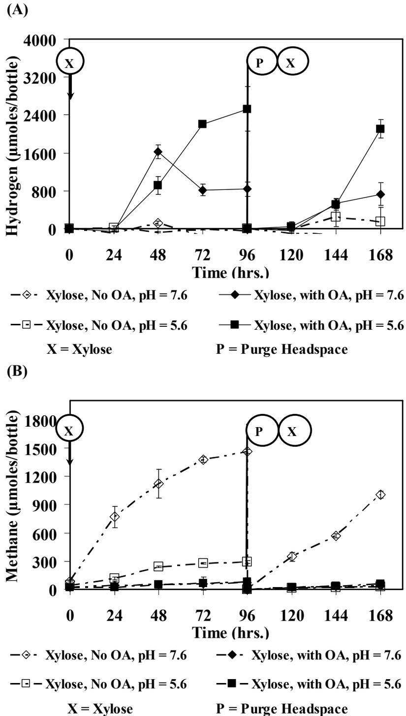
Figure 5.2 Gas production profiles for xylose (5,000 mg/L) degradation under different pH conditions in the presence of OA at 2,000 mg/L. Xylose injected at  $t = 0$  and again after purging at  $t = 96$  hrs (the data points represent triplicate samples; errors are indicated by the standard deviation). (A) Hydrogen production and (B) Methane production.
