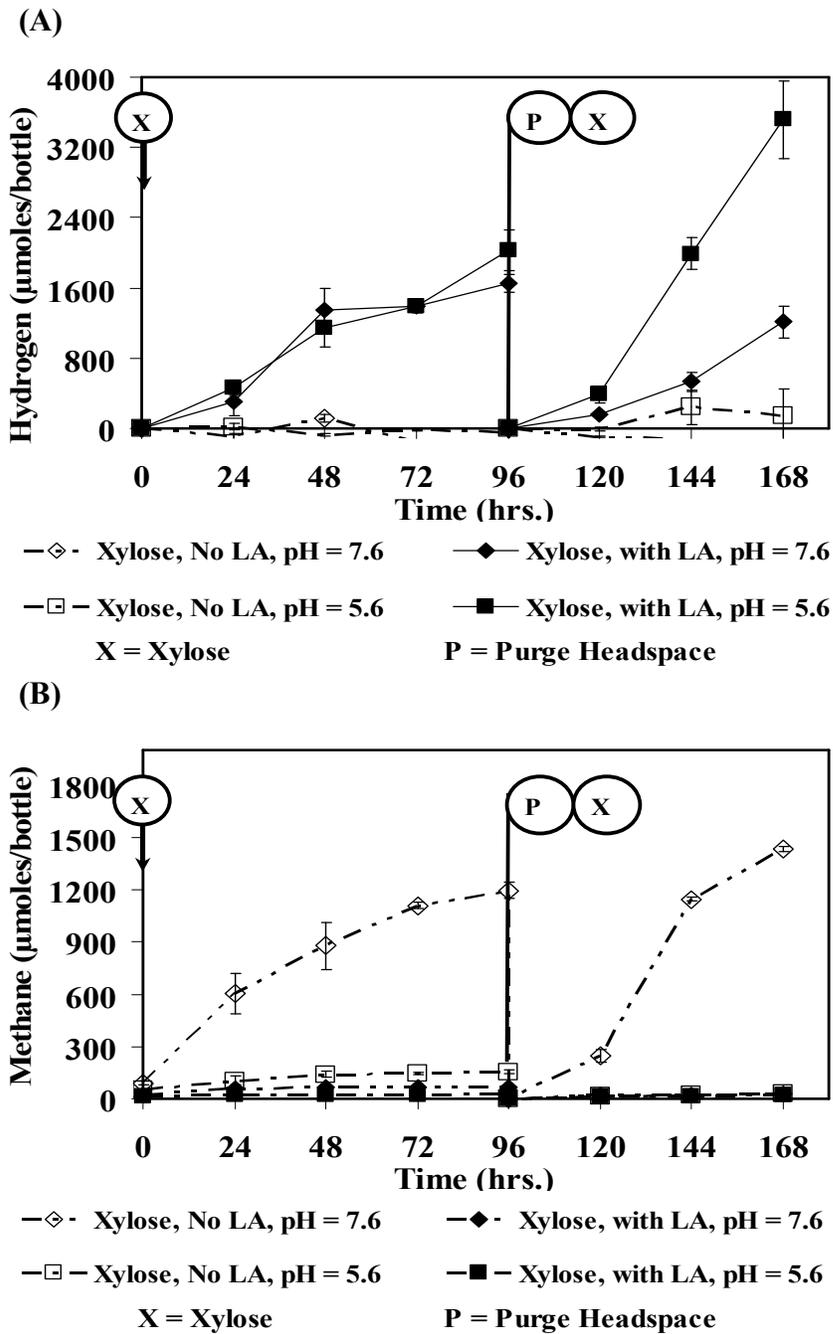
Figure 5.10 Gas production for the degradation of a 75%/25% mixture of xylose plus glucose (5,000 mg/L) under different pH conditions in the presence of LA at 2,000 mg/L. Sugars injected at  $t = 0$  and  $t = 96$  hrs (the data points represent triplicate samples; errors are indicated using the standard deviation). (A) Hydrogen production and (B) Methane production.
