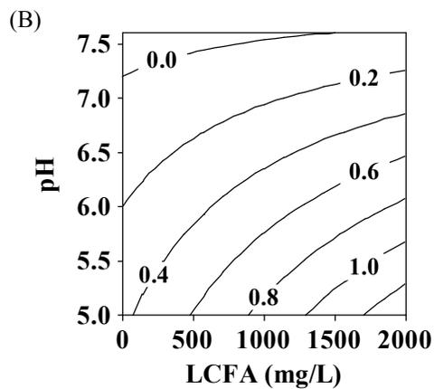
**Figure 4.8 Effect of variables on response ( $H_2$  yield). (A) Contour plot of response for pH versus LA concentration. (B) Contour plot of response for pH versus OA concentration.**
