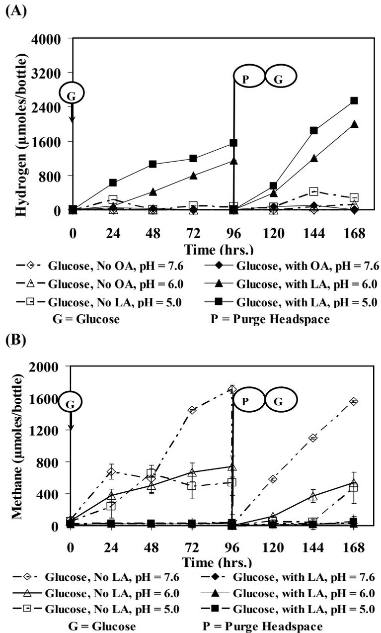
Figure 4.2 Effect of pH on gas production in cultures receiving 1,000 mg/L LA and 5,000 mg/L glucose. Glucose addition and pH adjustment at  $t = 0$  and  $t = 96$  hrs (the data points represent triplicate samples; errors are indicated using the standard deviation). (A) Hydrogen Production, (B) Methane Production.
