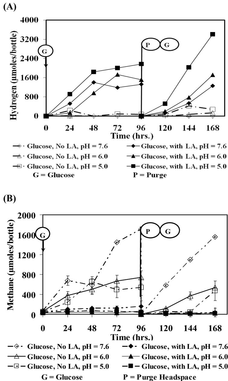
**Figure 4.1 Effect of pH on gas production in cultures receiving 2,000 mg/L LA and 5,000 mg/L glucose. Glucose addition and pH adjustment at  $t = 0$  and  $t = 96$  hrs (the data points represent triplicate samples; errors are indicated using the standard deviation). (A) Hydrogen production, (B) Methane Production.**
