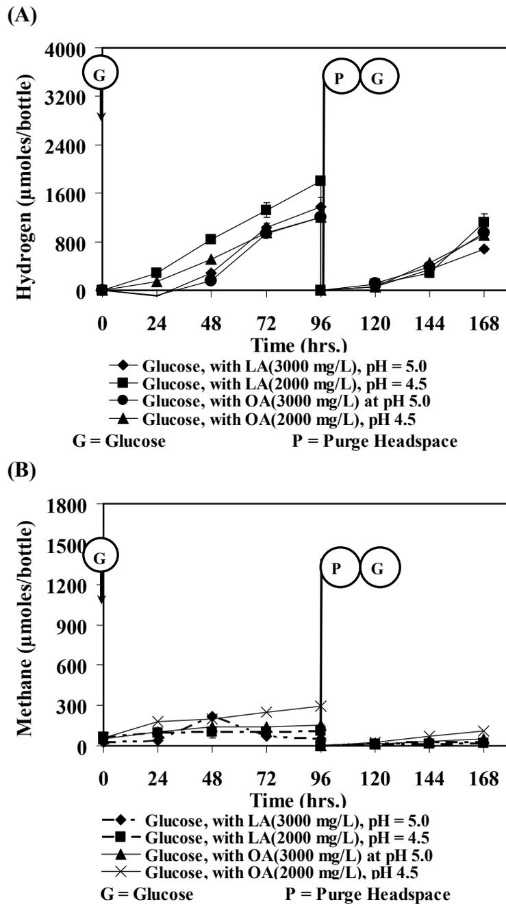
Figure 4.3 Gas production profiles for cultures receiving 3,000 mg/L LA or OA at pH 5 and culture receiving 2,000 mg/L LA or OA at pH 4.5, glucose addition (5,000 mg/L) at  $t = 0$  and  $t = 96$  hrs (each data point are for triplicate samples; errors are indicated using the standard deviation). (A) Hydrogen Production, (B) Methane Production.
