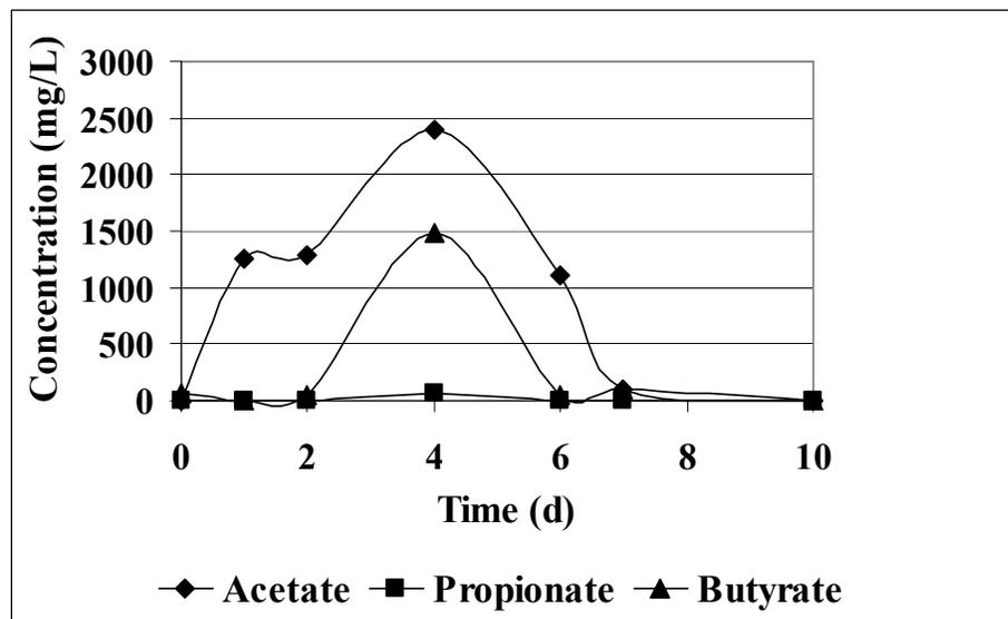
Figure 3.2 Profile for Reactor B VFA production and degradation
