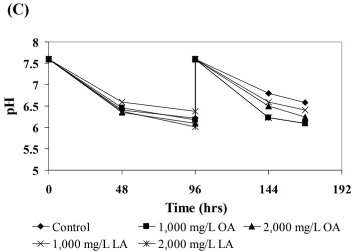
**Figure 4.12 The pH profile of the experiments conducted at different initial pH values with the pH set at  $t=0$  hrs and re-adjusted at  $t=96$  hrs. (A) Samples run at initial pH 5, (B) samples run at initial pH 6, and (C) samples run at initial pH 7.6.**
