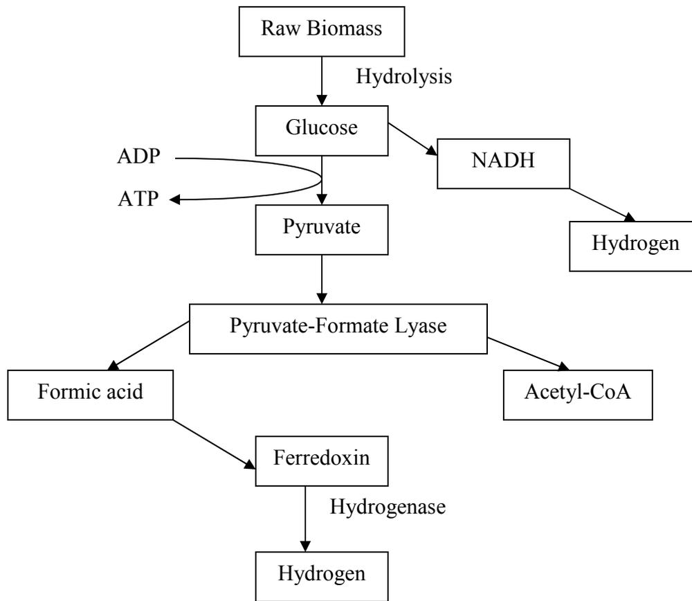
**Figure 2.2 Biochemical decomposition of biomass into hydrogen (adapted from Nath and Das, 2004).**
