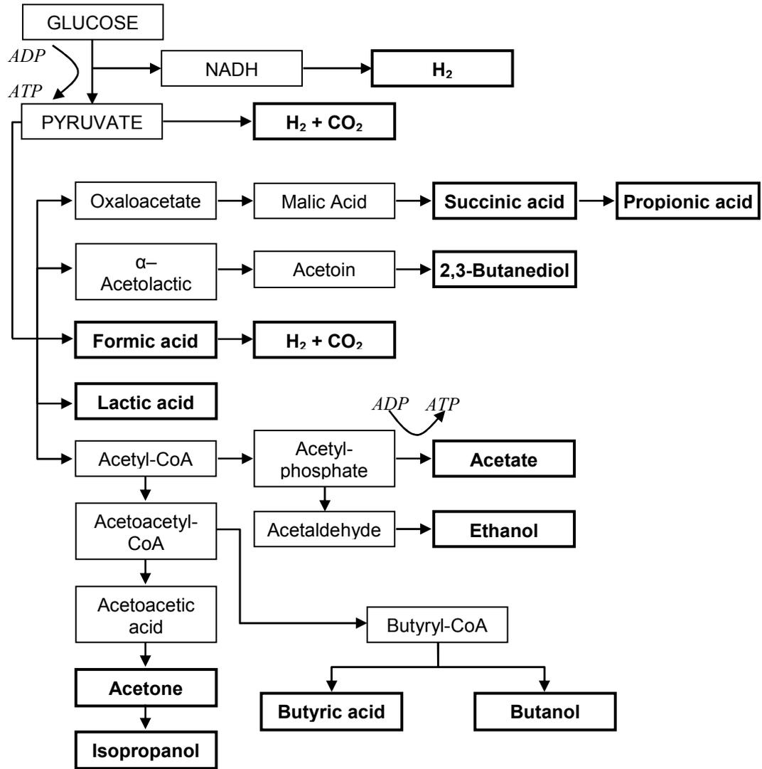
Figure 2.5 Pathways to the end products of the fermentation of sugars. (End products indicated by bold text) (Adapted from Gaudy & Gaudy, 1980)
