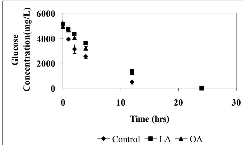
**Figure 4.11** Glucose degradation of 5,000 mg/L glucose containing 0 and 2,000 mg/L LCFA at a pH of 7.6 (data for glucose added at t=0) (each data point are for triplicate samples; errors are indicated using the standard deviation).
