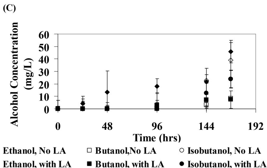
**Figure 5.12** Alcohol production for cultures at pH 5.6 and fed 2,000 mg/L LA plus sugars (glucose, xylose and glucose plus xylose). Sugars injected at  $t = 0$  and  $t = 96$  hrs (the data points represent triplicate samples; errors are indicated using the standard deviation). (A) Samples fed 5,000 mg/L xylose. (B) Samples fed 5,000 mg/L glucose. (C) Samples fed 2,500 mg/L xylose and 2,500 mg/L glucose together.
