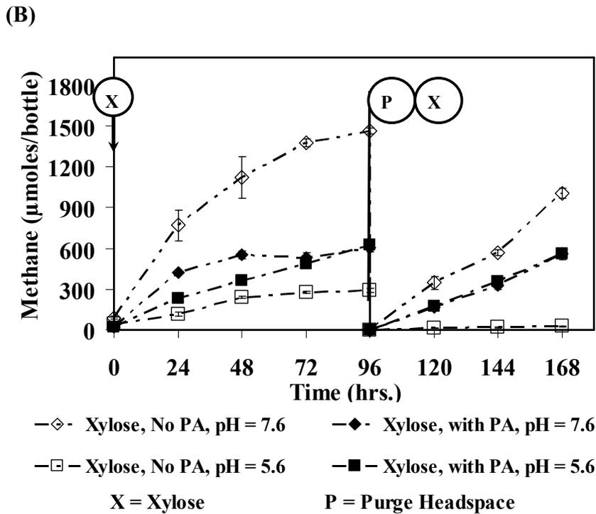
**Figure 5.5 Gas production profiles for xylose (5,000 mg/L) degradation under different pH conditions in the presence of PA at 2,000 mg/L. Xylose injected at  $t = 0$  and again after purging at  $t = 96$  hrs (the data points represent triplicate samples; errors are indicated by the standard deviation). (A) Hydrogen production and (B) Methane production.**
