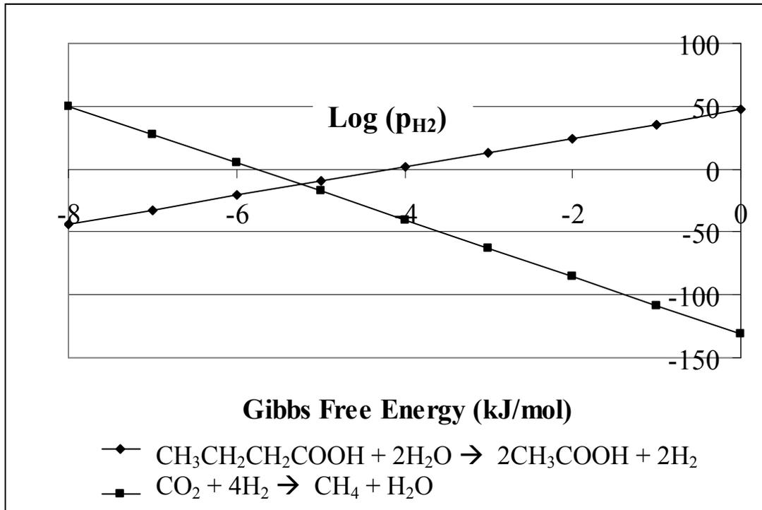
**Figure 2.6  $\Delta G$  vs. hydrogen partial pressure ( $P_{H_2}$ ) plot of a hydrogen producing reaction and a hydrogen consuming reaction**
