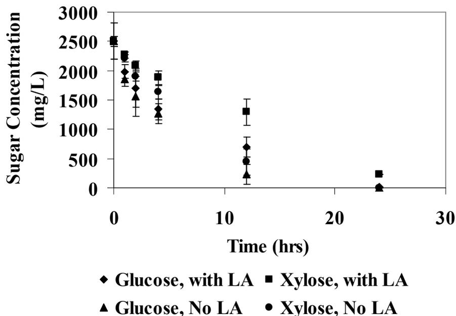
**Figure 5.13 Xylose and glucose (5,000 mg/L total) degradation plus 2,000 mg/L LA at a pH of 7.6 (glucose and xylose added at  $t = 0$ , the data points represent triplicate samples; errors are indicated using the standard deviation).**
