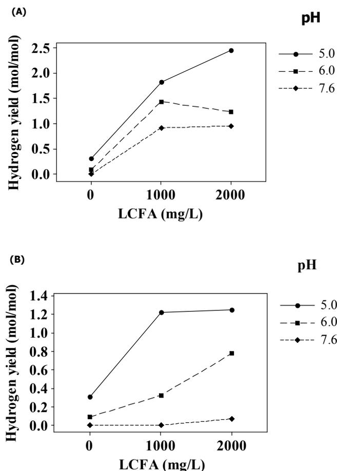
**Figure 4.7 Factorial plots of hydrogen yield in a two factor, three level FFD, (A) LA two factor interaction plot (B) OA two factor interaction plot**
