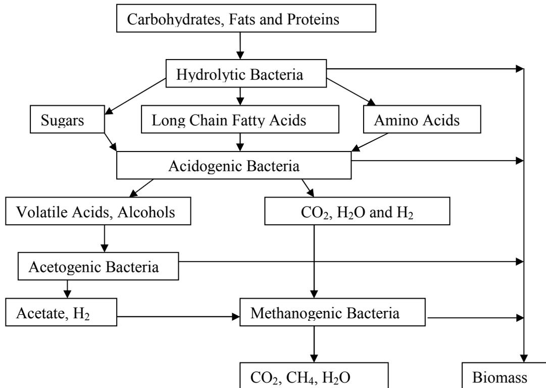
**Figure 2.1 Typical anaerobic degradation pathway of organic substrates**
