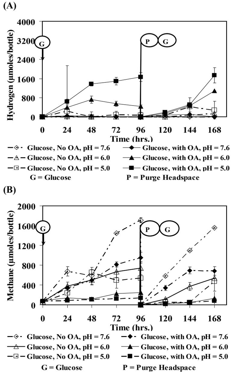
Figure 4.4 Effect of pH on gas production in cultures receiving 2,000 mg/L OA and 5,000 mg/L glucose. Glucose addition and pH adjustment at  $t = 0$  and  $t = 96$  hrs (each data point are for triplicate samples; errors are indicated using the standard deviation). (A) Hydrogen Production, (B) Methane Production.
