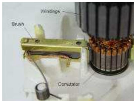
*Figure C.1. DC commutator and brush*
