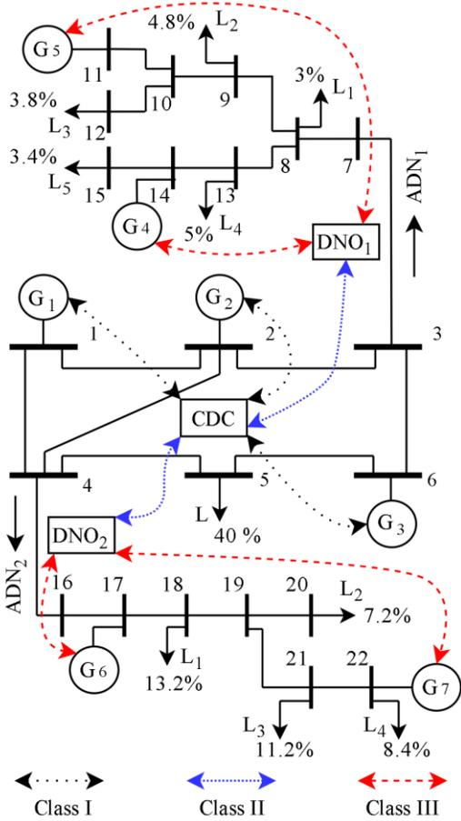
Fig. 2. Six-bus transmission system with two ADNs (T6D2),  $G_1$ - $G_3$  are bulk generators while  $G_4$ - $G_7$  are DGs.
