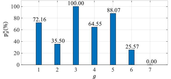
Fig. 5. The normalized output power obtained by solving the EDP-CTADS-WL and recalculating the slack output power ( $g = 1$  for the slack generator).
