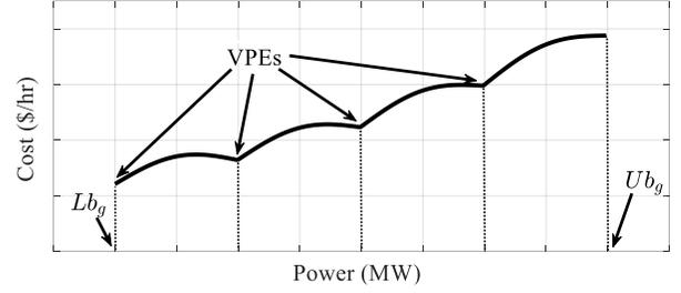
Fig. 7. Non-convex cost function of a unit having VPEs.
