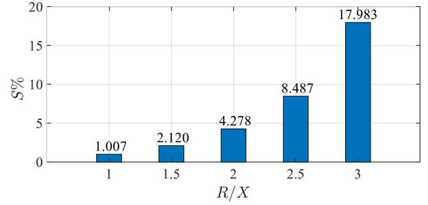
Fig. 3. Percentage saving (S%), due to considering the network losses, as a function of the R/X ratio.
