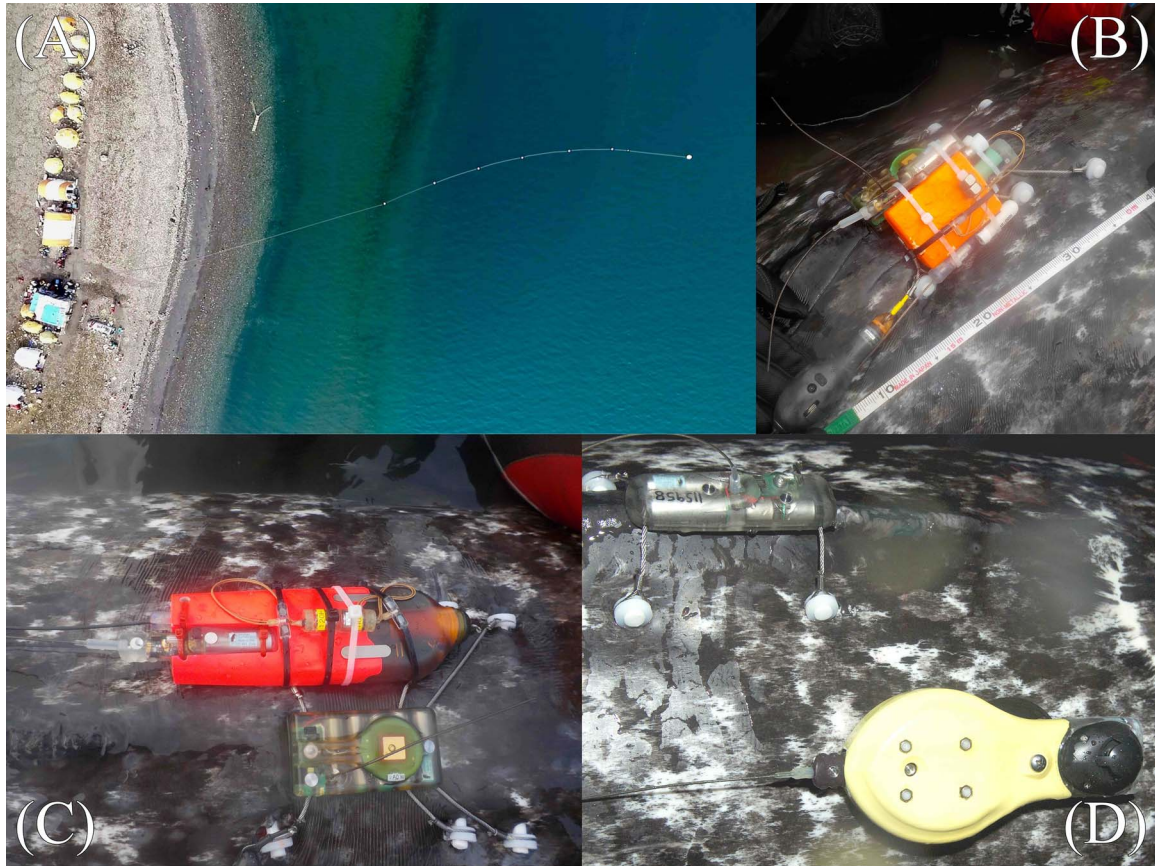
Figure 1: Images showing net deployment anchored perpendicular to shore (A) in Tremblay Sound ( 72^{\circ}21.389\text{ N} , -81^{\circ}05.855\text{ W} ), an example of attachment of the bolt-on configuration (3 pins) for a TDR-10 satellite tag, and accompanying (B) Maritime Biologgers (MBL) deployment package with timed release mechanism attached to pins or (C) Acousonde unit attached via both a suction cup mounting and little Leonardo releases held across the spider wires holding the TDR-10 satellite tag to the dorsal ridge and (D) a Daily Diary (TDR-DD) tag attached with a suction cup under a bolt-on satellite tag (2 pins).
