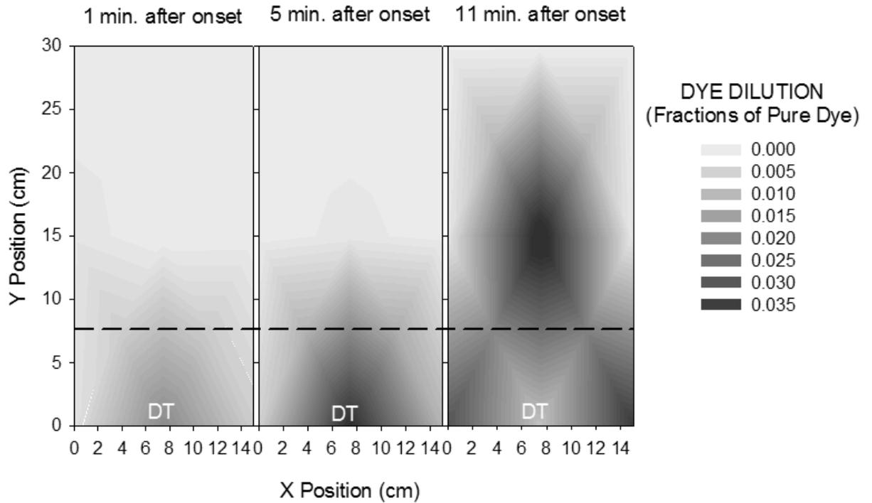
**Figure 11.** Contour plots showing average (over ten trials) dye dilutions (expressed as fractions of the pure dye delivered) at given points throughout the assay tanks at 1 minute, 5 minutes, and 11 minutes after the onset of dye delivery. Dye was delivered for 10 minutes. The dashed line denotes the boundary of the inflow zone, and DT denotes the location of the dye delivery tube.
