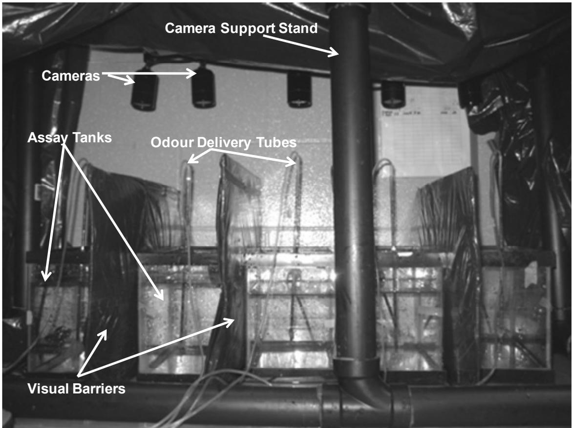
**Figure 10.** Five-tank behavioural assay set-up with inflow tubes and drains. Barriers were placed between the tanks to prevent fish from seeing each other. Each tank is below an infrared digital video camera, which send video to a computer (not shown).
