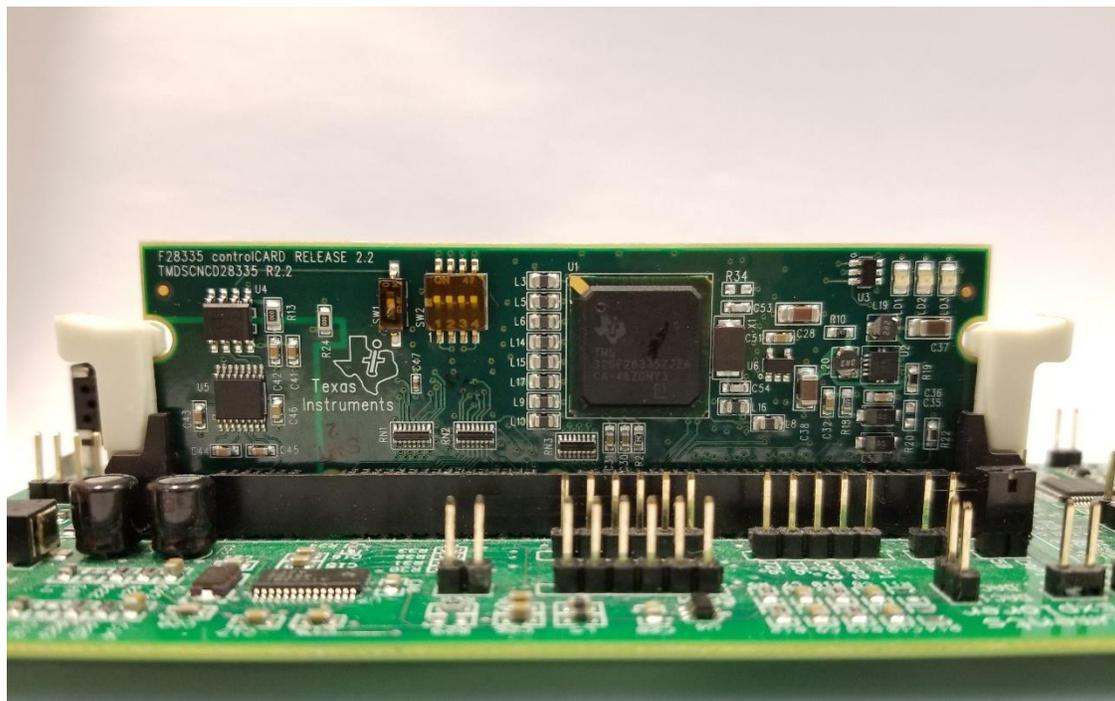
Figure 2: View of the microcontroller on the evaluation board
