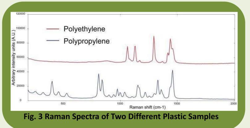
Fig. 3 Raman Spectra of Two Different Plastic Samples
