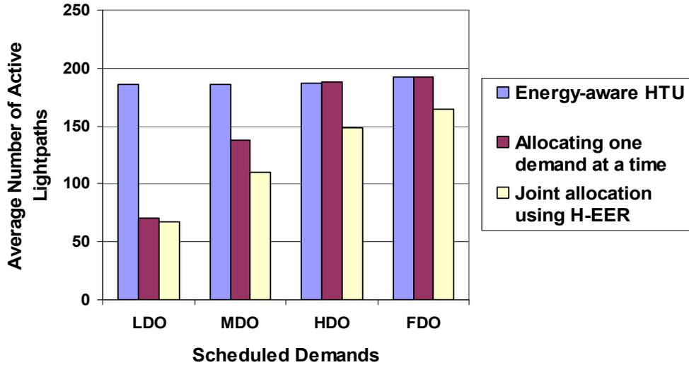
Figure 4.4: Comparison of the average number of active lightpaths used for single and joint demand allocation.
