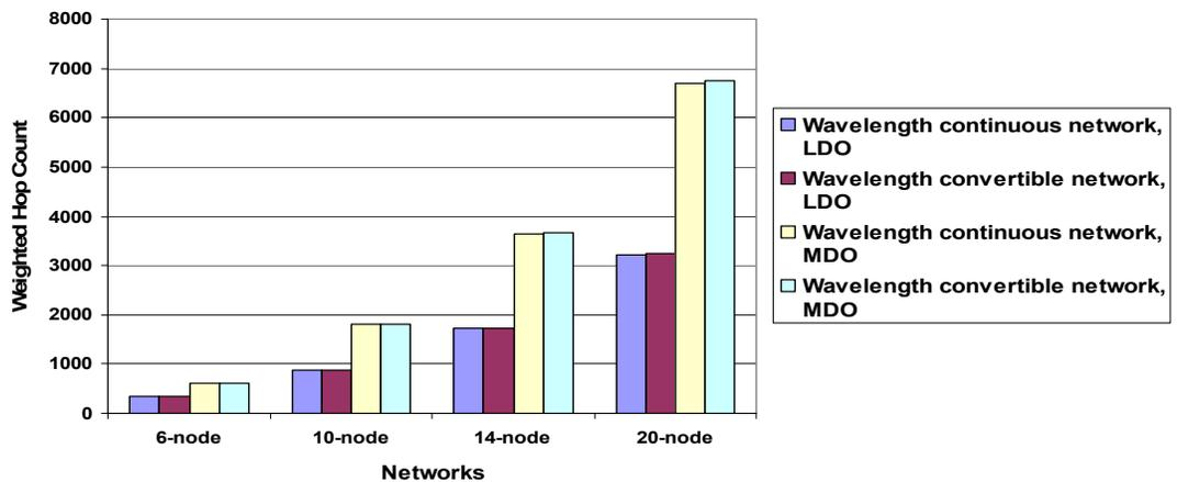
Figure 3.5: Comparison of resource requirements in wavelength continuous and wavelength convertible networks under LDO and MDO models.
