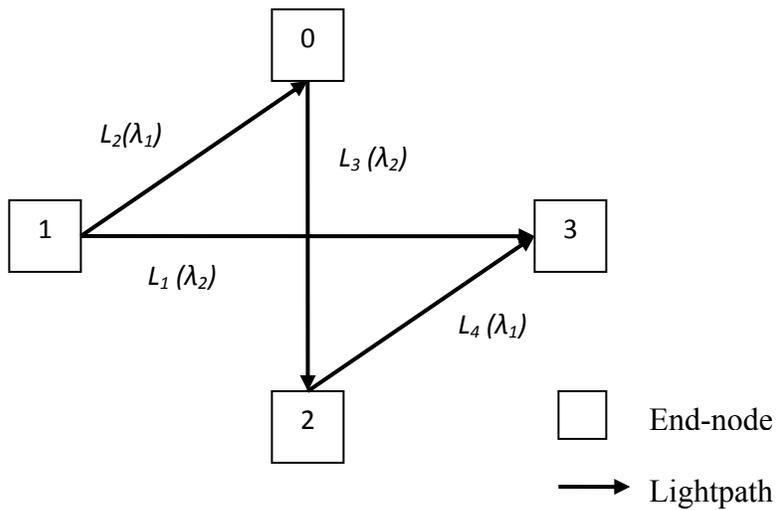
Figure 1.2: Logical topology corresponding to the lightpaths shown in Fig. 1.1.
