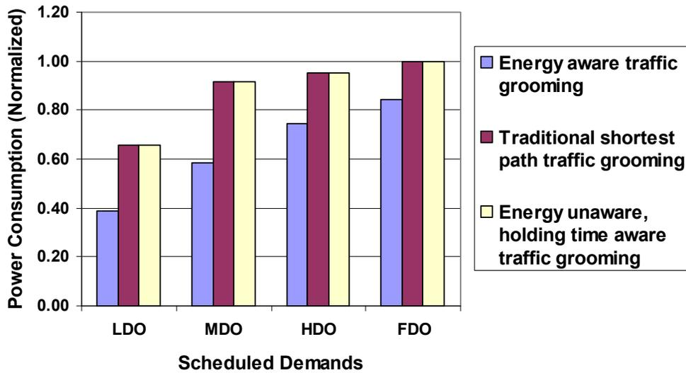
Figure 4.6: Comparison of total power consumption for FDO case, traditional traffic grooming and H-EER for a 10-node network.
