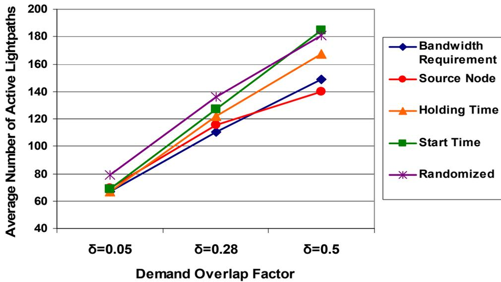
Figure 4.8: Comparison of the average number of active lightpaths used for different sorting criteria.
