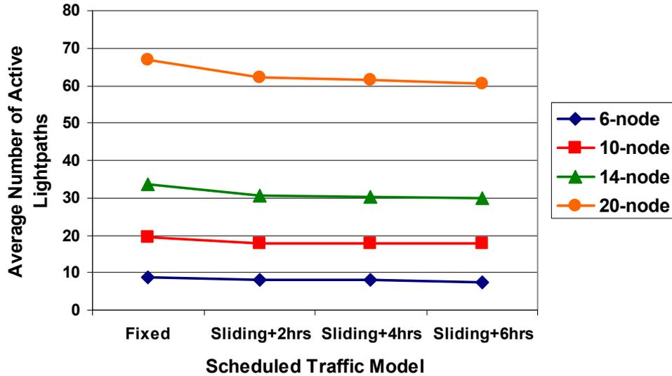
Figure 4.10: Effect of increasing window size for different topologies.
