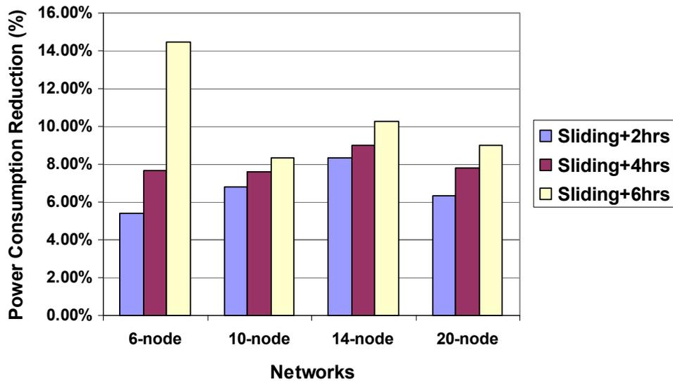
Figure 4.9: Percentage reduction in total power consumption compared with the fixed scheduled traffic model.
