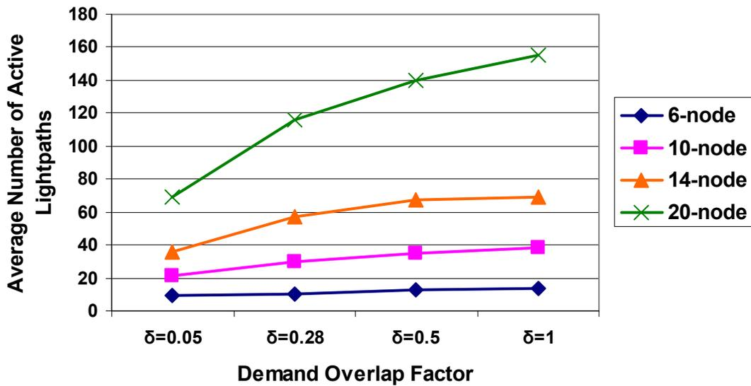
Figure 4.7: Comparison of the average number of active lightpaths used for different topologies.
