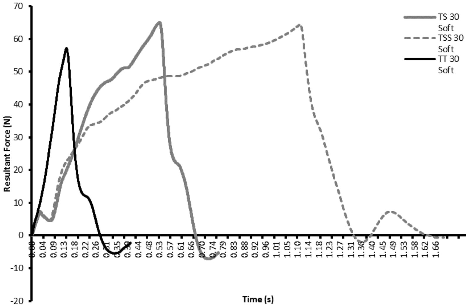
Figure 47: A visual representation of the three fastening strategies recorded by the RAPT handle for soft joints displaying the time periods and resultant forces for 30 Nm hard joints. This shows that the turbo tight fastening strategy takes place over a short period of time and results in a lower force occurring at the RAPT handle.
