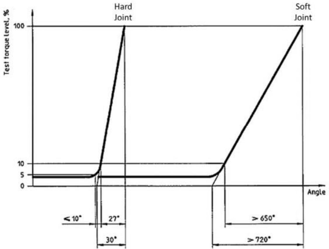
Figure 5: Spindle head angle vs. torque level in hard and soft-joints (International Standards Organization, 1994).
