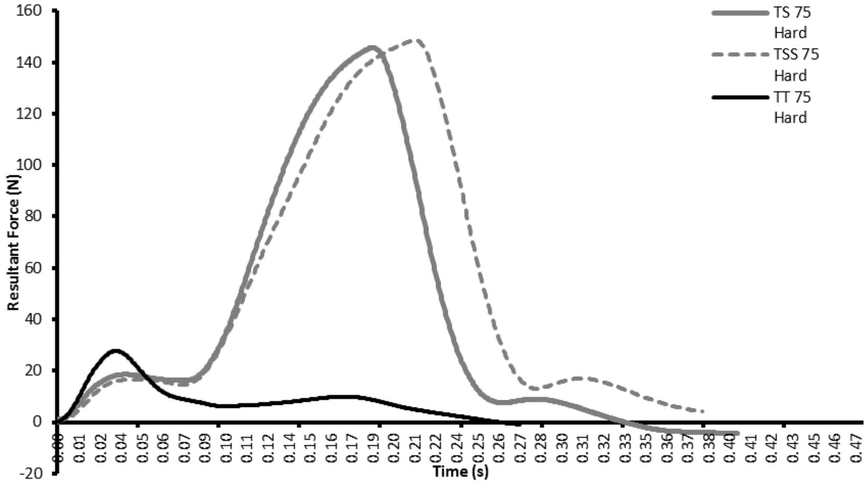
Figure 46: A visual representation of the three fastening strategies recorded by the RAPt handle for hard joints displaying the time periods and resultant forces for 75 Nm hard joints. This shows that the turbo tight fastening strategy takes place over a short period of time and results in a lower force occurring at the RAPt handle.
