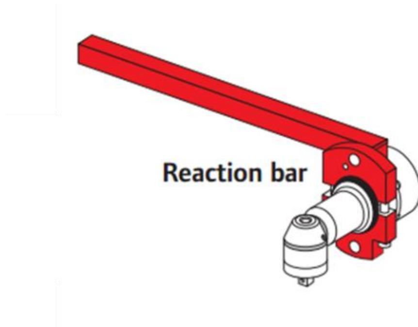
Figure 7: Reaction bar placed on a RAPT to help reduce the force produced by the tool (Ingersoll Rand, 2008). reaction forces to lessen what the operator experiences (Radwin et al., 1989). Unfortunately, this reaction bar can add weight and restrict tool placement so it may only be suitable for specific jobs and joints (Forsman et al., 2002).
