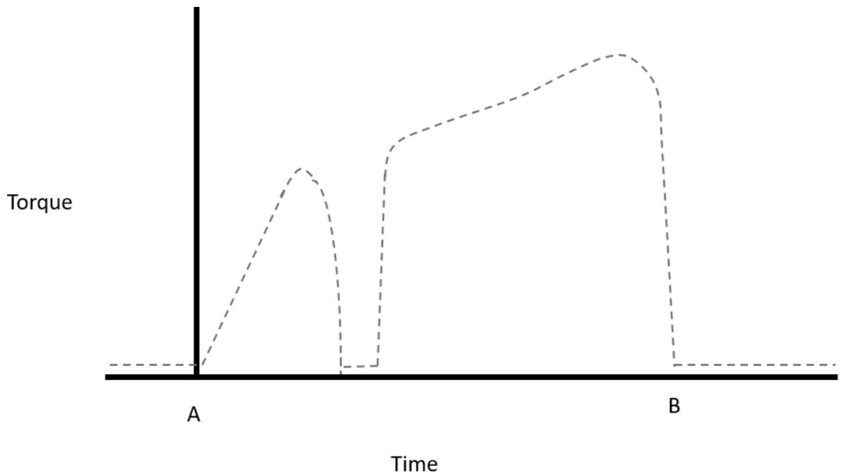
Figure 25: Time history of a torque curve during fastening rundown broken into impulse time periods: A. Trigger initiation. B. End of rundown.
