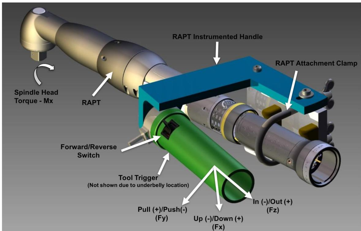
Figure 21: RAPT and Instrumented Handle Attached with Direction of Forces and components of the instrumented handle
