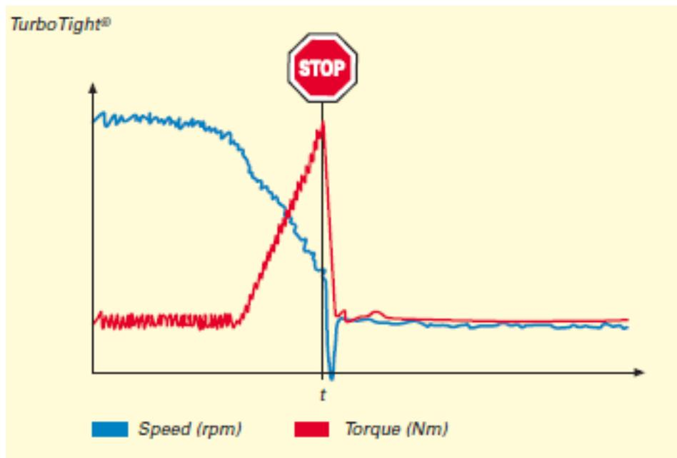
Figure 3: Turbo tight fastening strategy showing torque and speed profile during rundown (Atlas Copco, 2013a).
