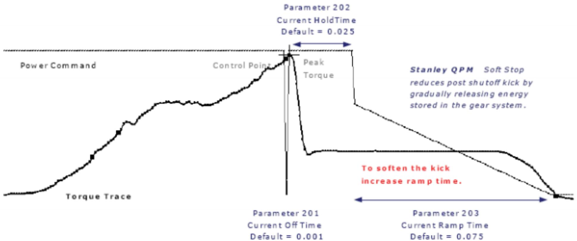
Figure 4: Fastening rundown profile with soft stop feature added, showing current off time, hold time and ramp time of the feature with the default times associated with each phase (Mukherji, 2008).
