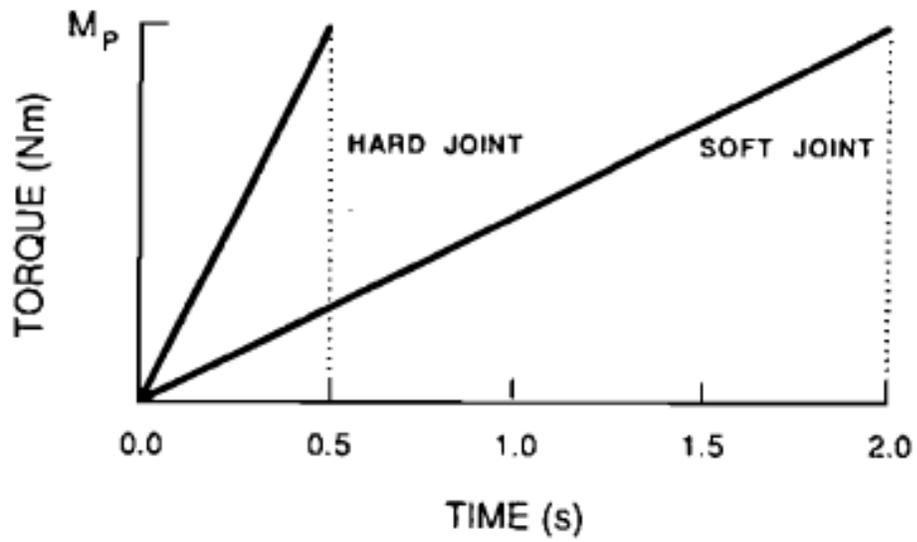
Figure 6: Torque buildup time for hard and soft-joints (Radwin et al., 1989) .
