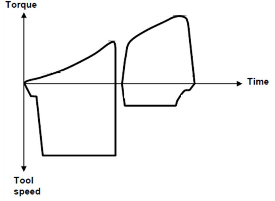
Figure 2: Tightening profiles: A) One stage with one constant velocity B) Two stage with high speed first step, a break and a lower speed second step (Atlas Copco, 2013b).
