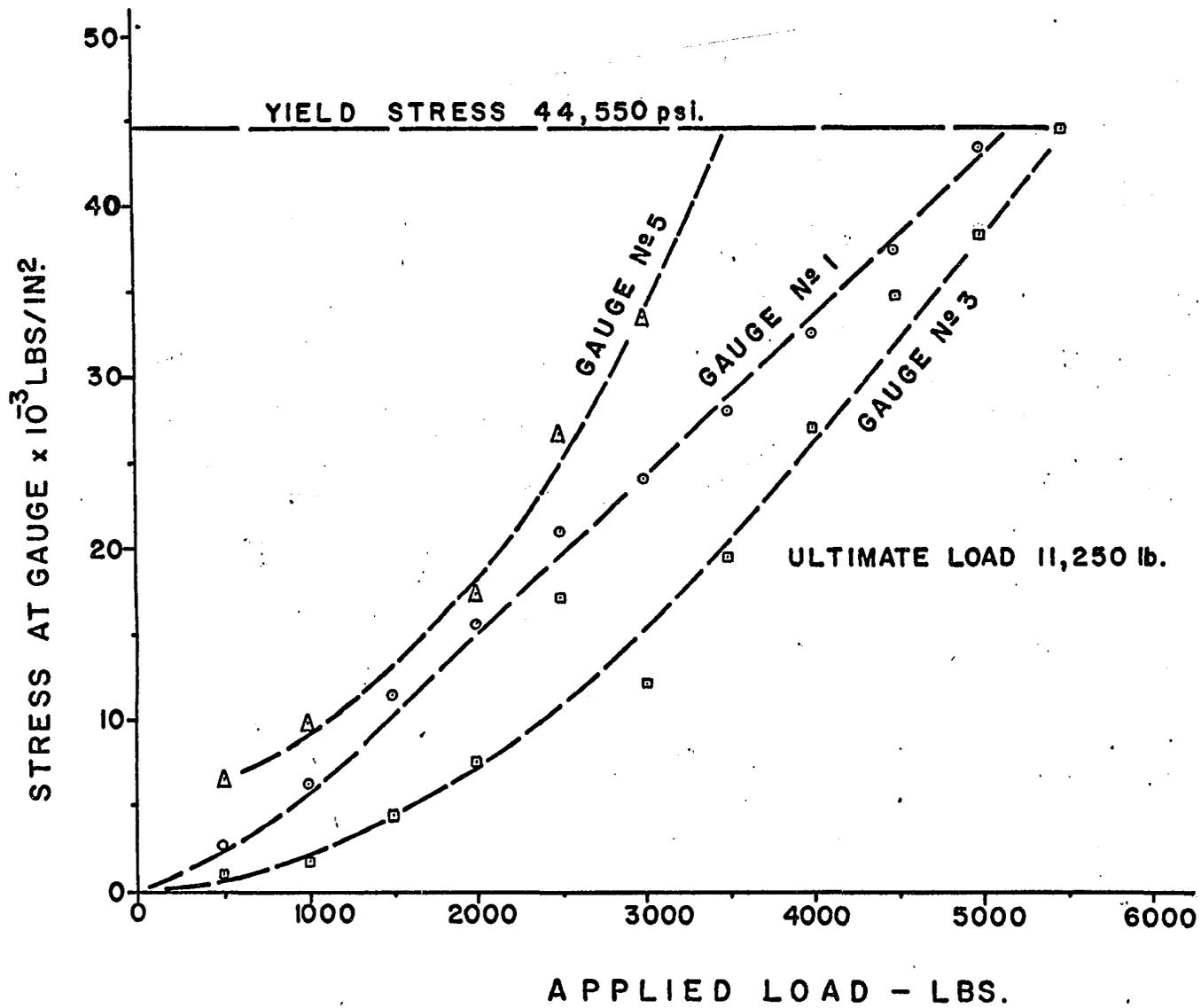
STRESS vs CONNECTION LOAD FOR TEST NO. 734-C
