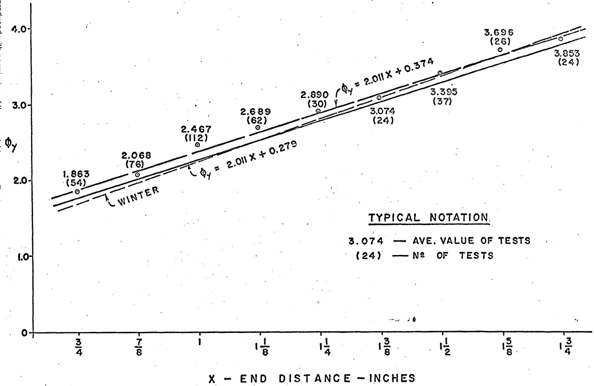
RELATIONSHIP BETWEEN  $\phi_y$  AND END DISTANCE FOR END FAILURE
