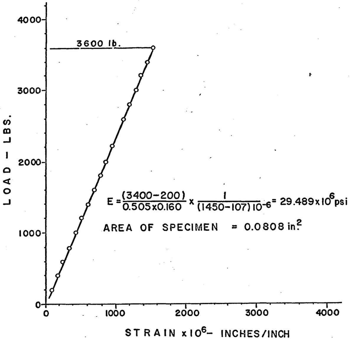
LOAD-STRAIN CURVE FOR TENSION
