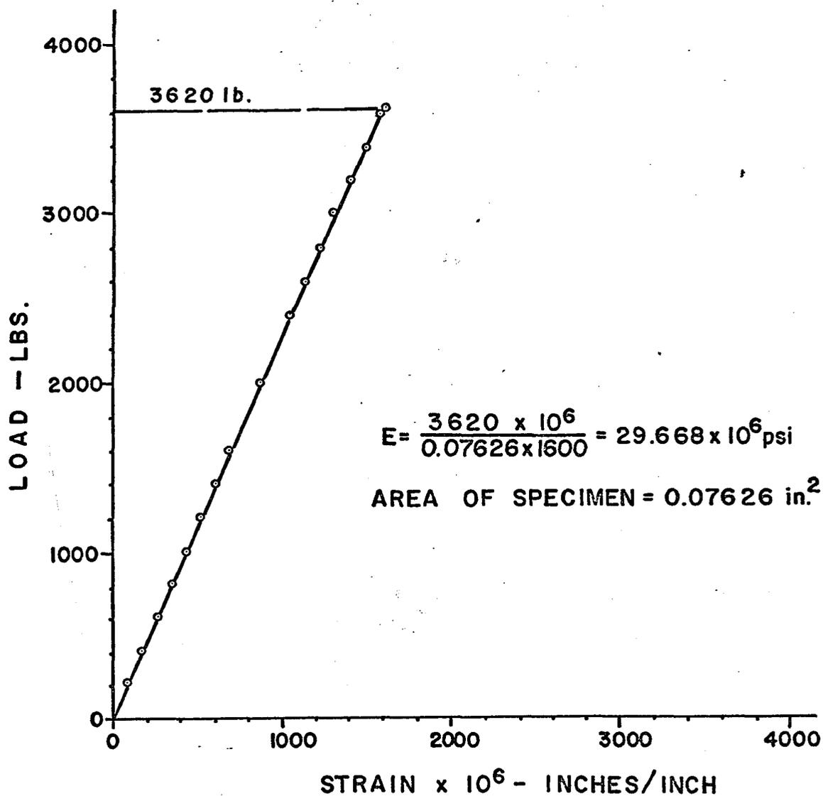
LOAD-STRAIN CURVE FOR TENSION
