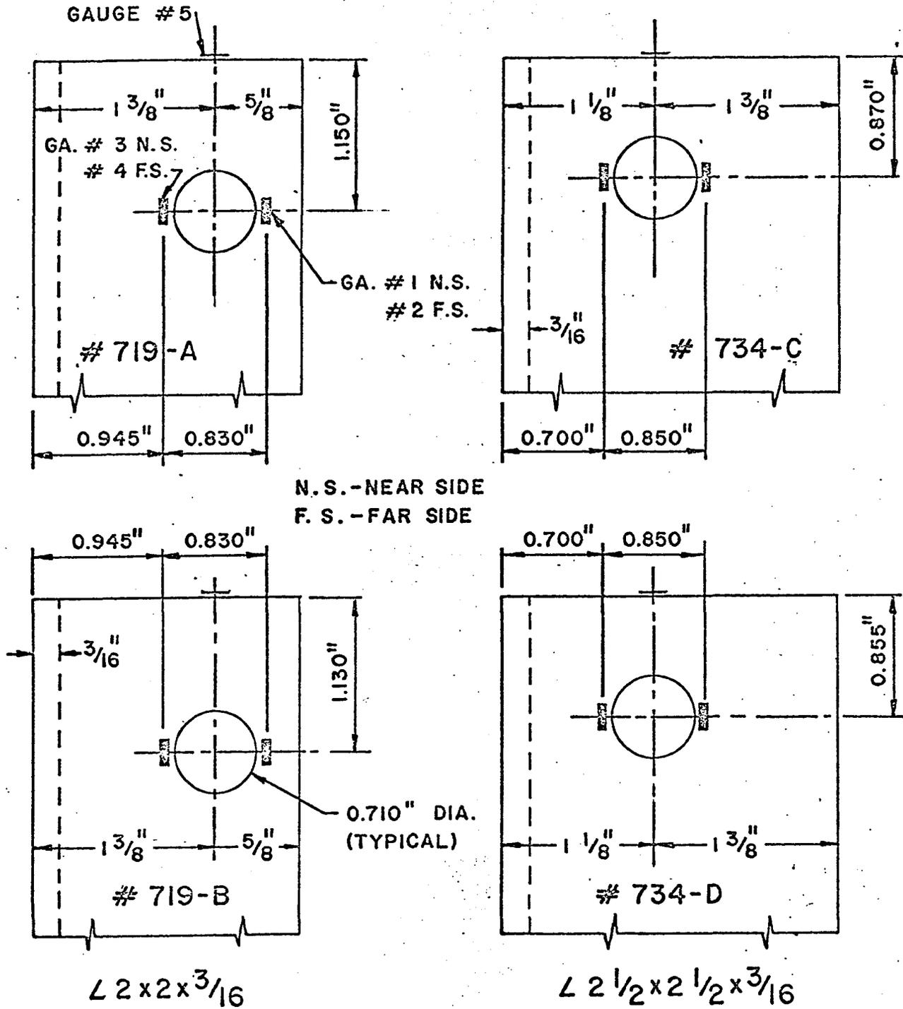
DETAIL OF TEST PIECES SHOWING LOCATIONS OF STRAIN GAUGES
