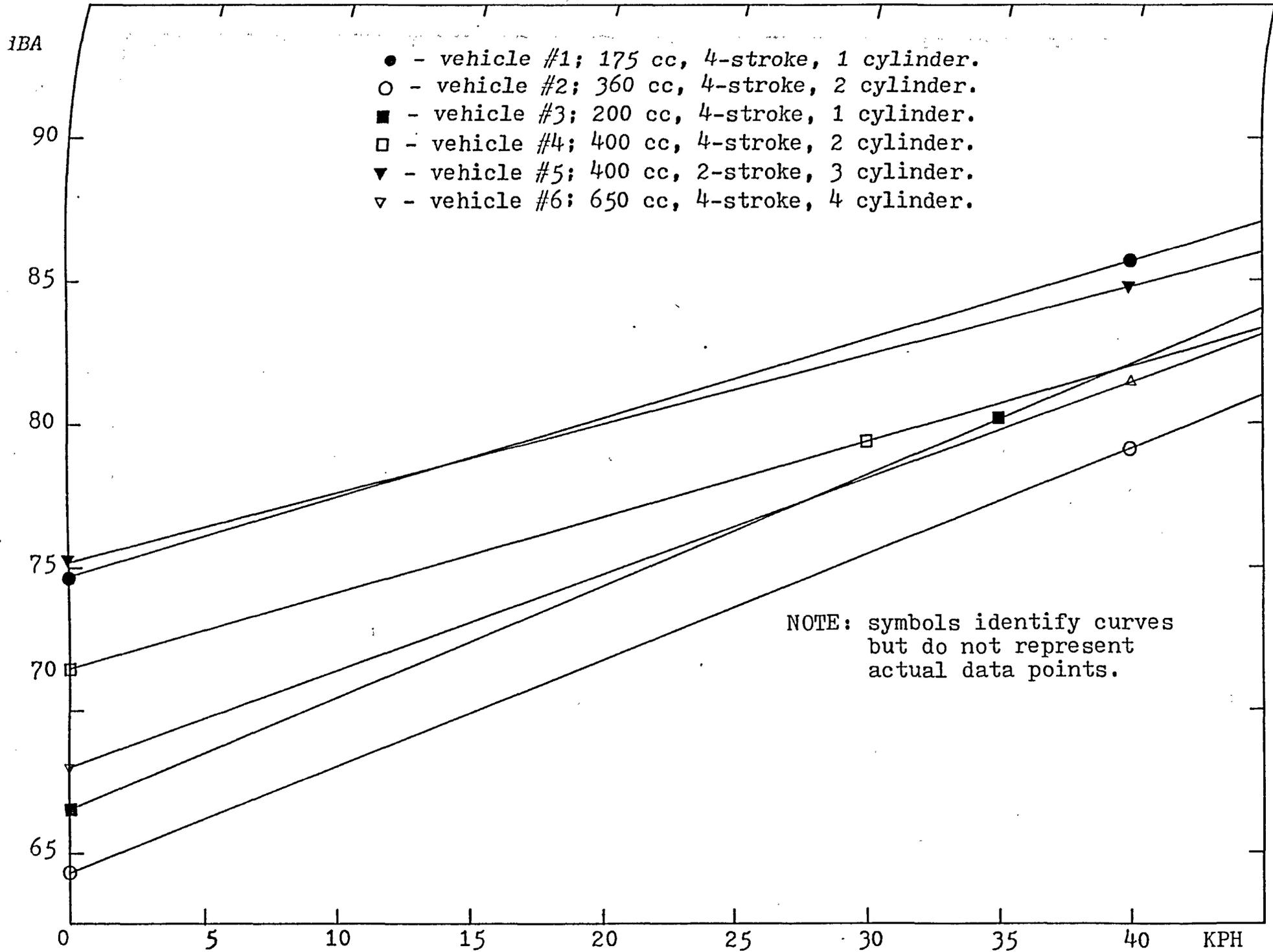
FIGURE F10- Vehicle comparison of  $AVG_2$  for slope and zero-intercept.
