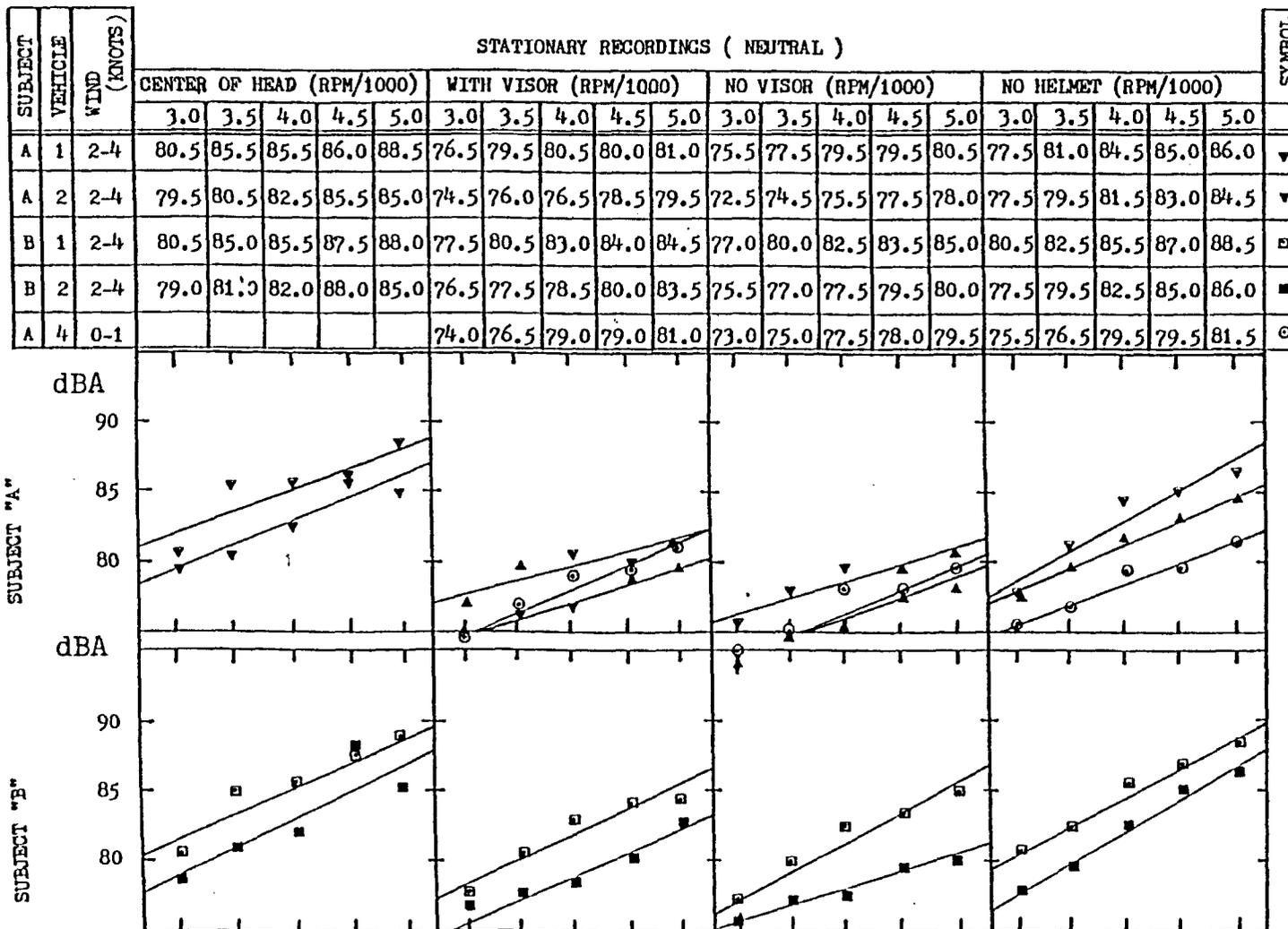
TABLE TB3 - Sound level data from auxiliary stationary testing.
