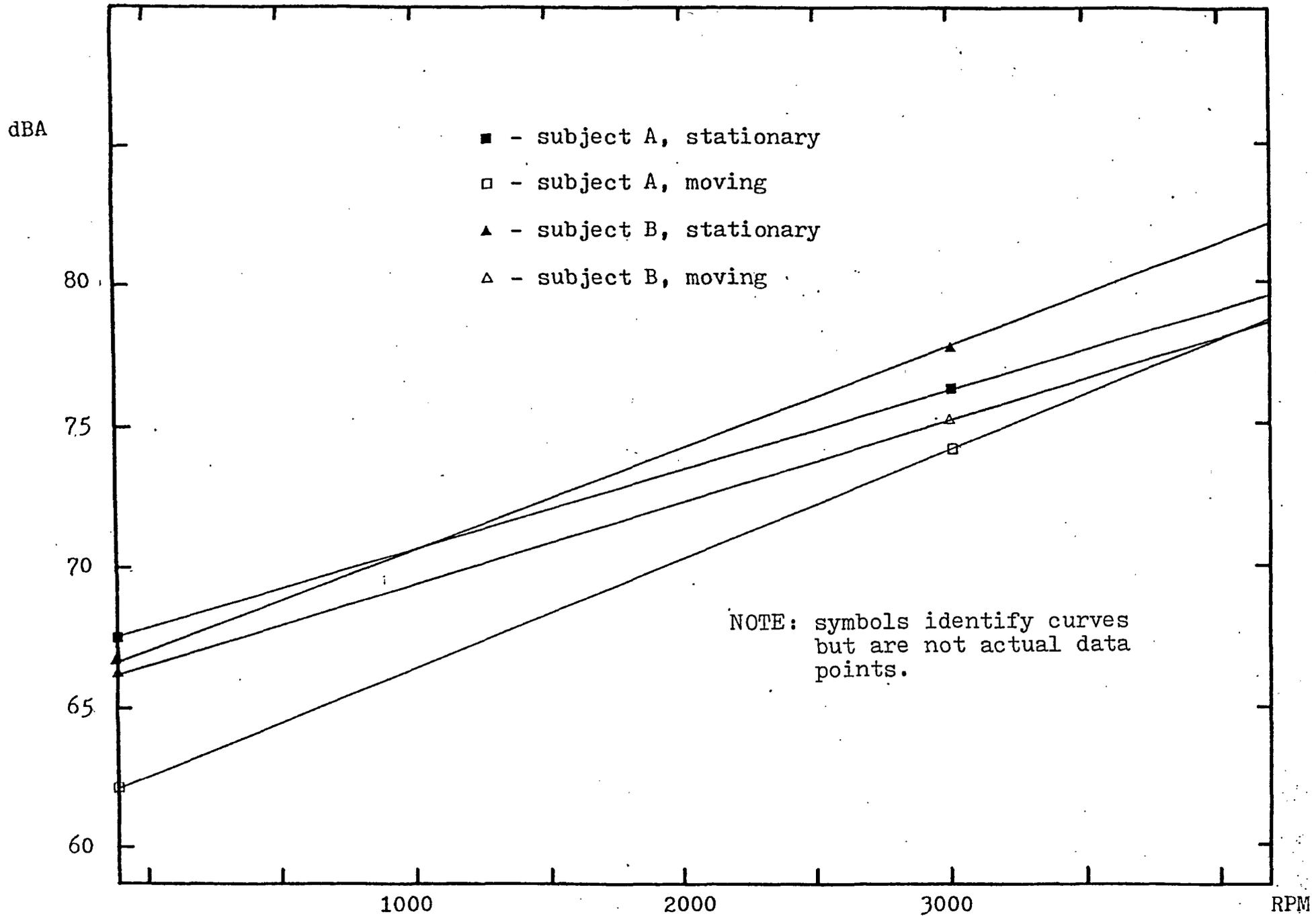
FIGURE FB4 - Plot of  $AVG_2$  of auxiliary recording results for stationary versus moving test (subject comparison).
