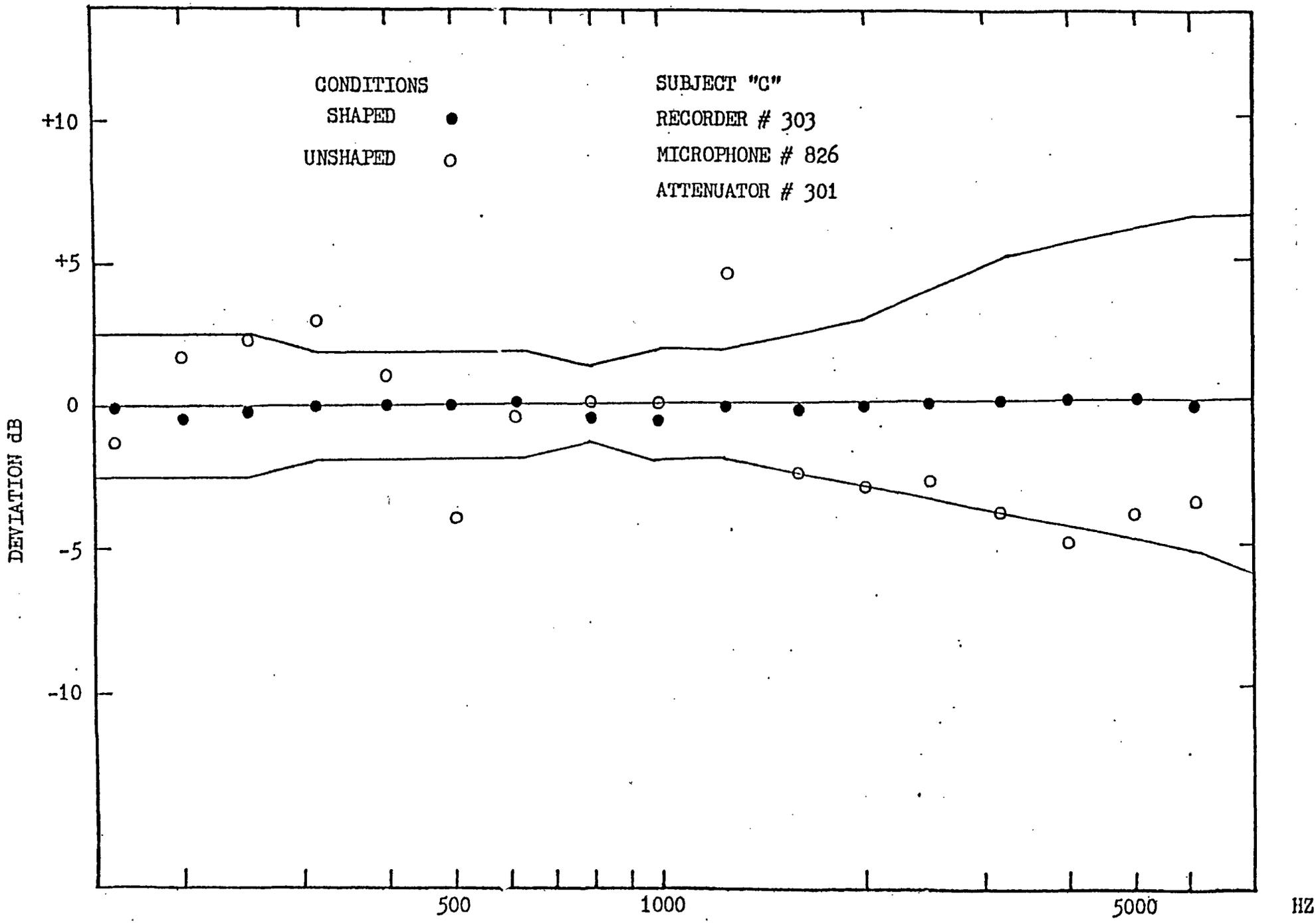
FIGURE FB8 - Narrow band frequency spectrum of shaped and unshaped frequency characteristics for a particular ear bug unit.
