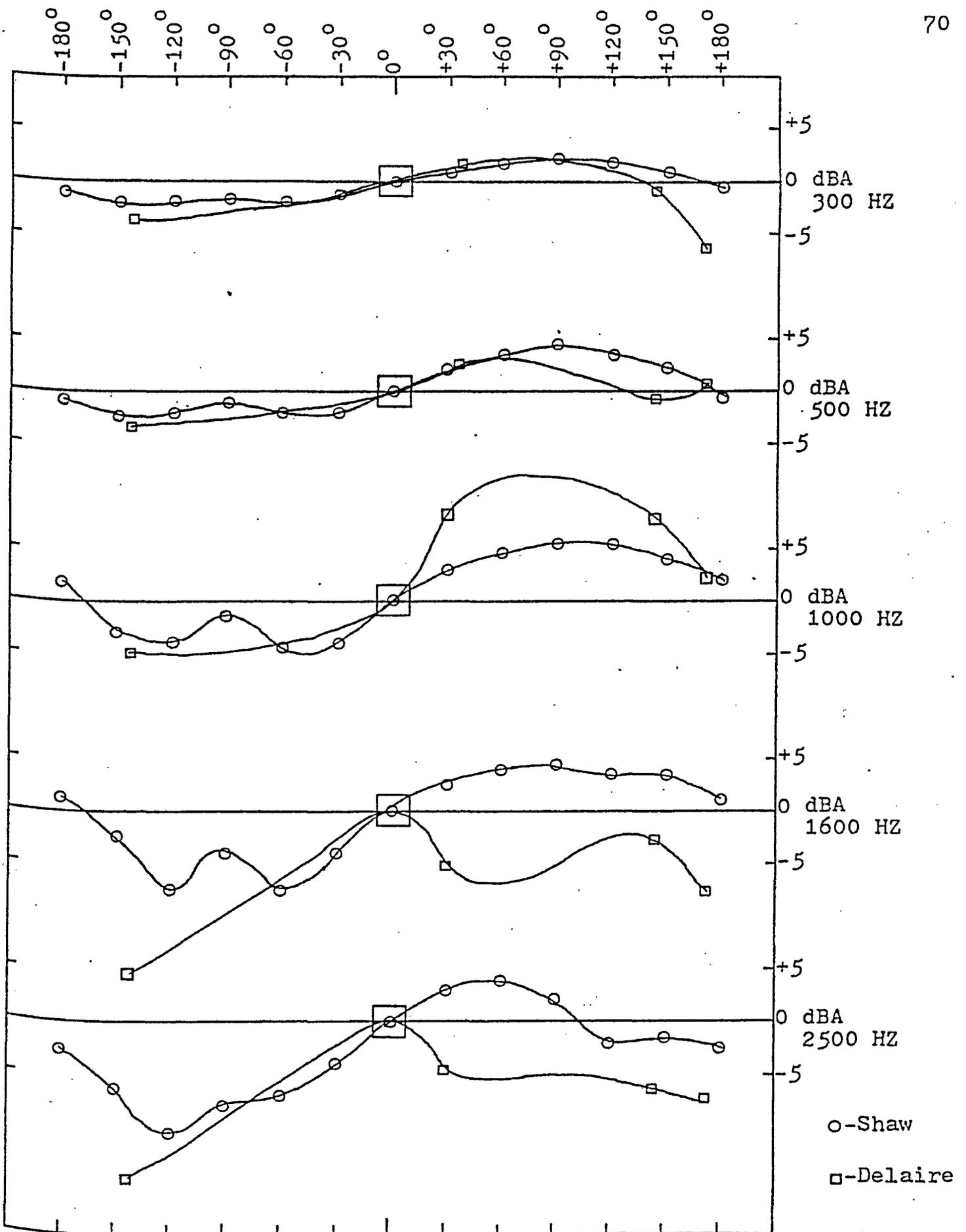
FIGURE F9 - Sound pressure versus angle of incidence at specific frequencies. (Shaw- azimuthal plane only; Delaire- floor plane + azimuthal plane).
