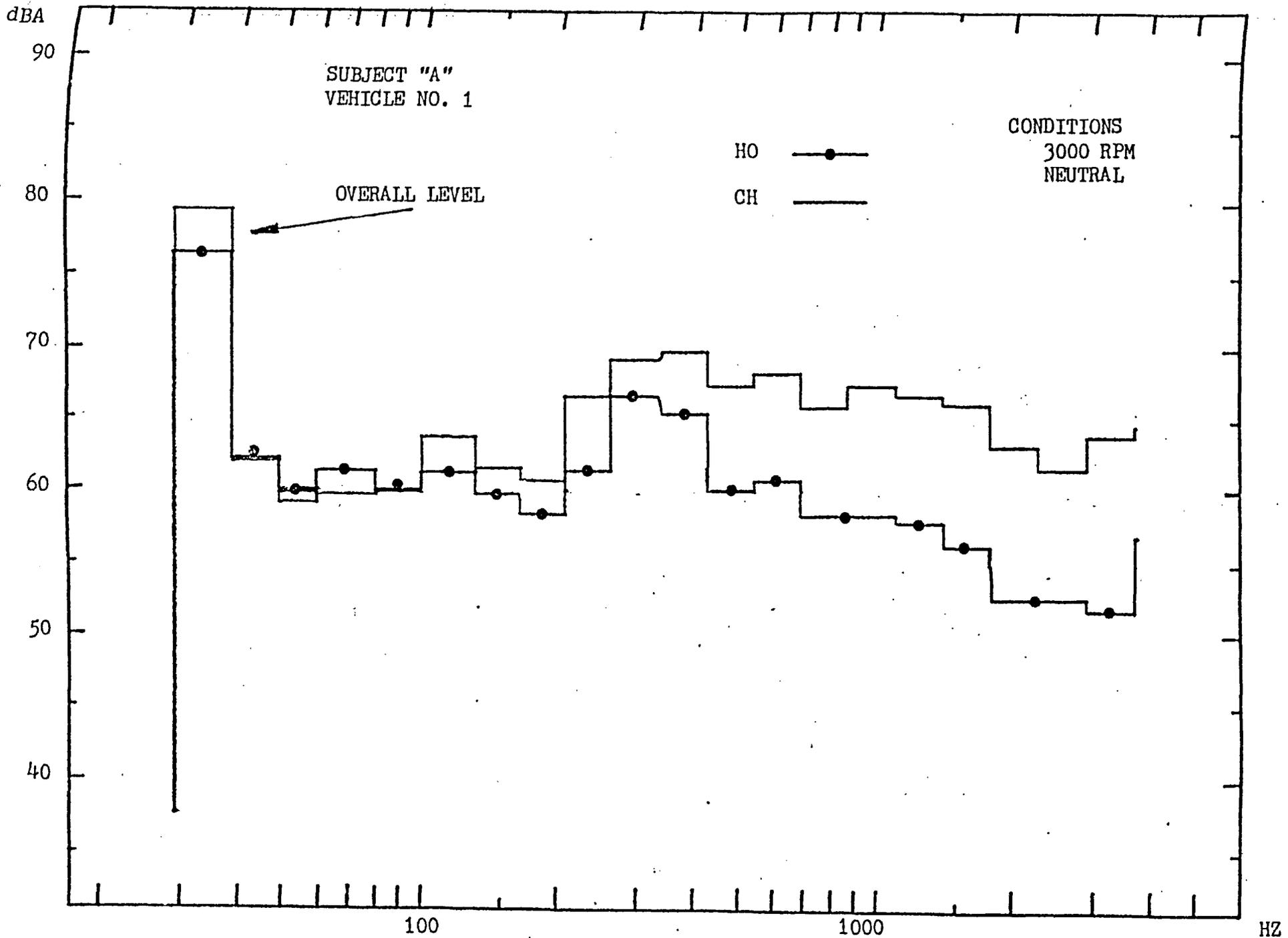
FIGURE F8- Typical 1/3- octave plot of motorcycle noise via real time analyzer.
