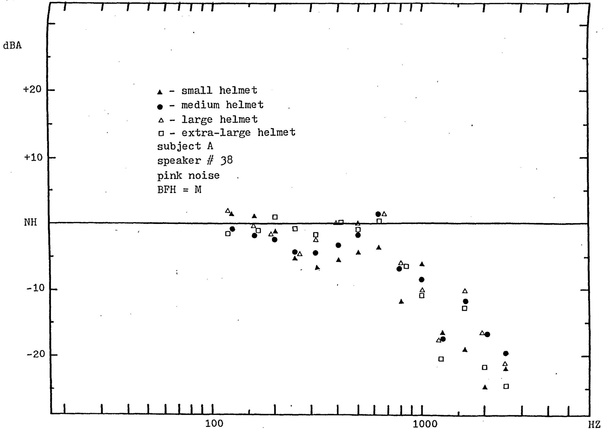
FIGURE F168 - 1/3 octave frequency spectrum of helmet + visor attenuation for all helmet sizes.
