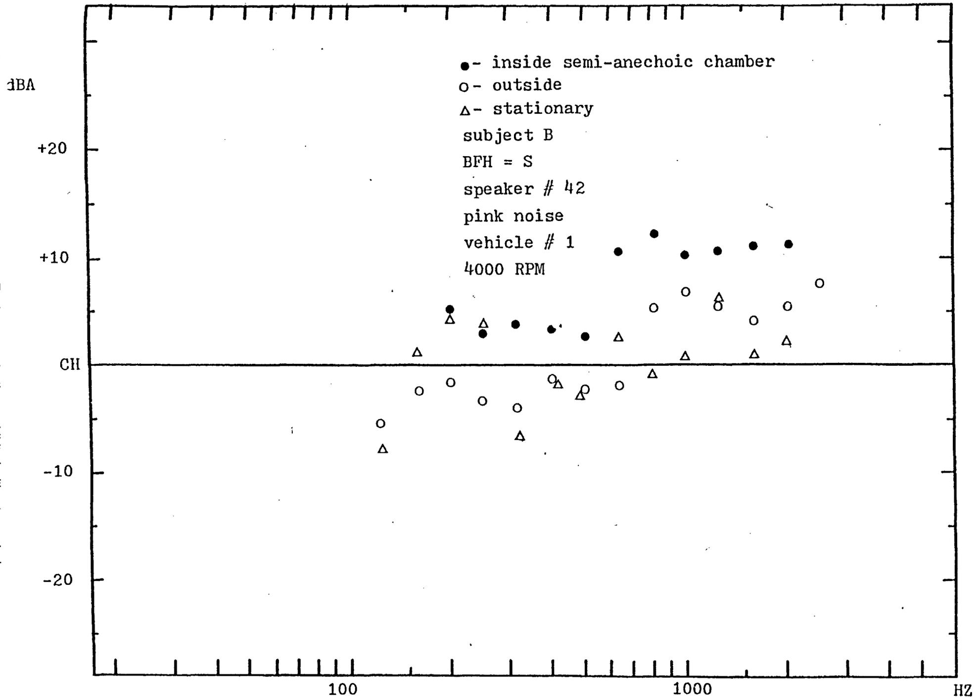
FIGURE FB2 $\alpha$  - 1/3 octave frequency spectrum of transfer function for inside-outside-stationary comparison.
