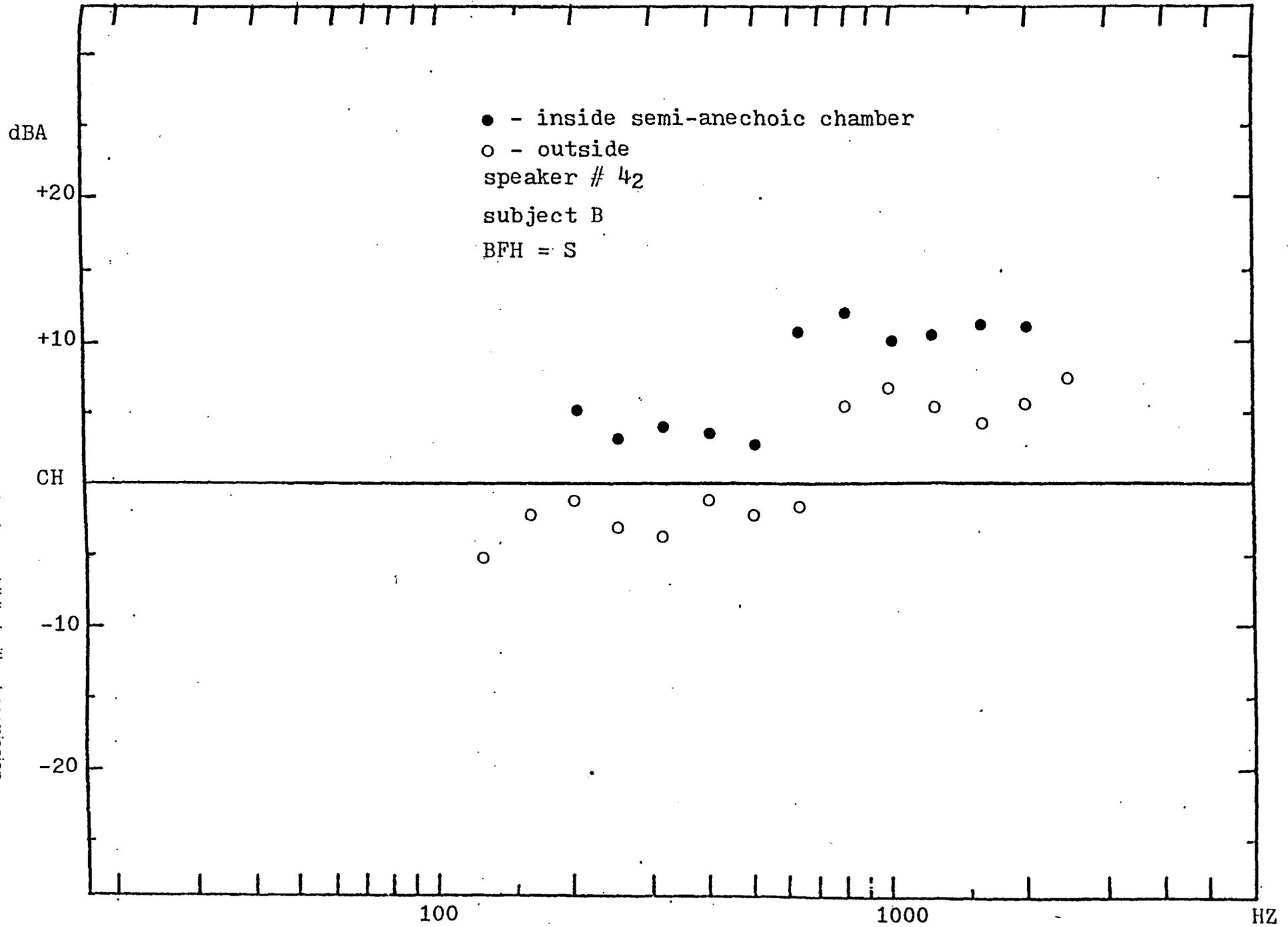
FIGURE FB1α - 1/3 octave frequency spectrum of transfer function for recordings made inside and outside.
