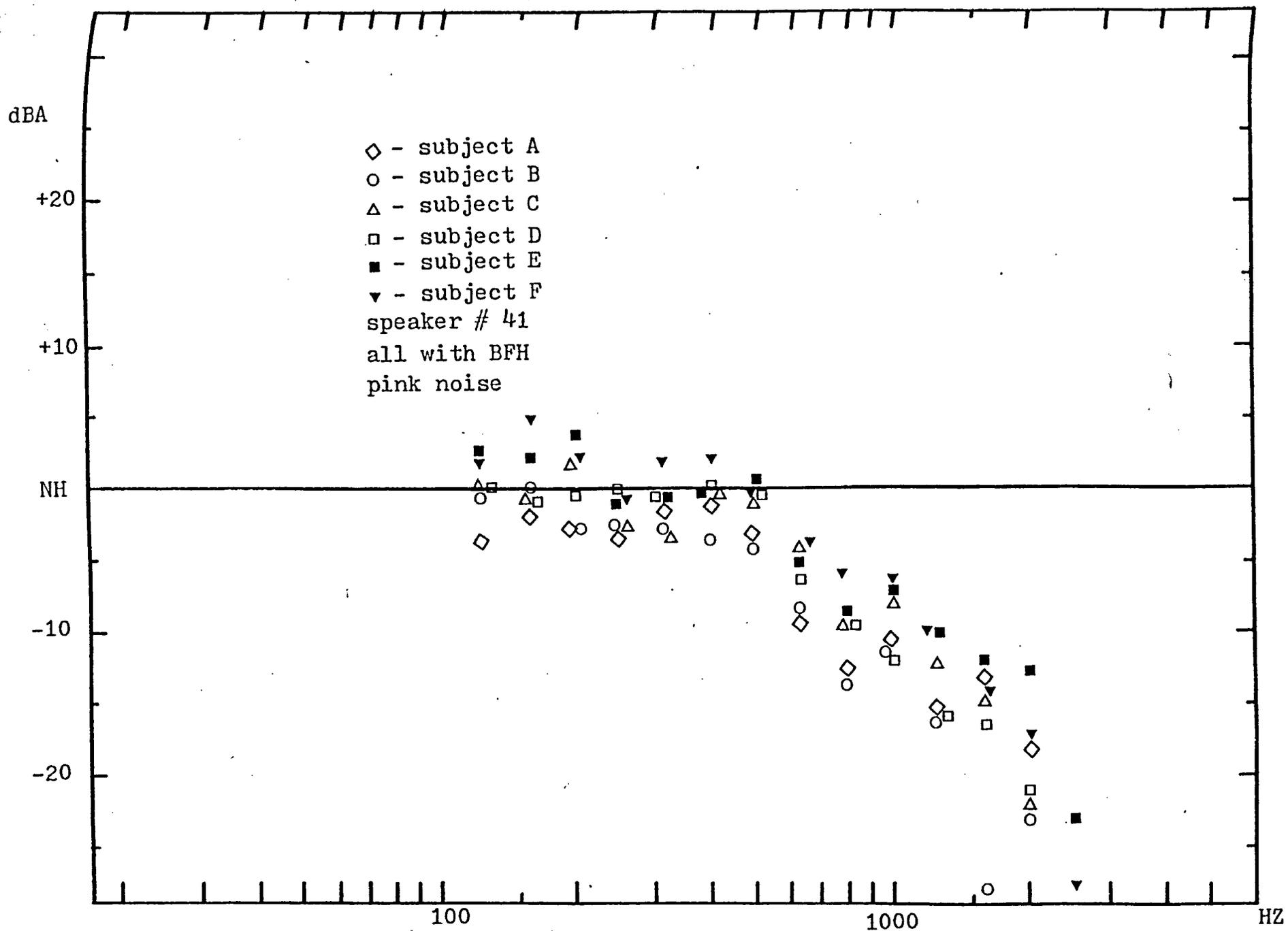
FIGURE F158 - 1/3 octave frequency spectrum of helmet + visor attenuation for all subjects.
