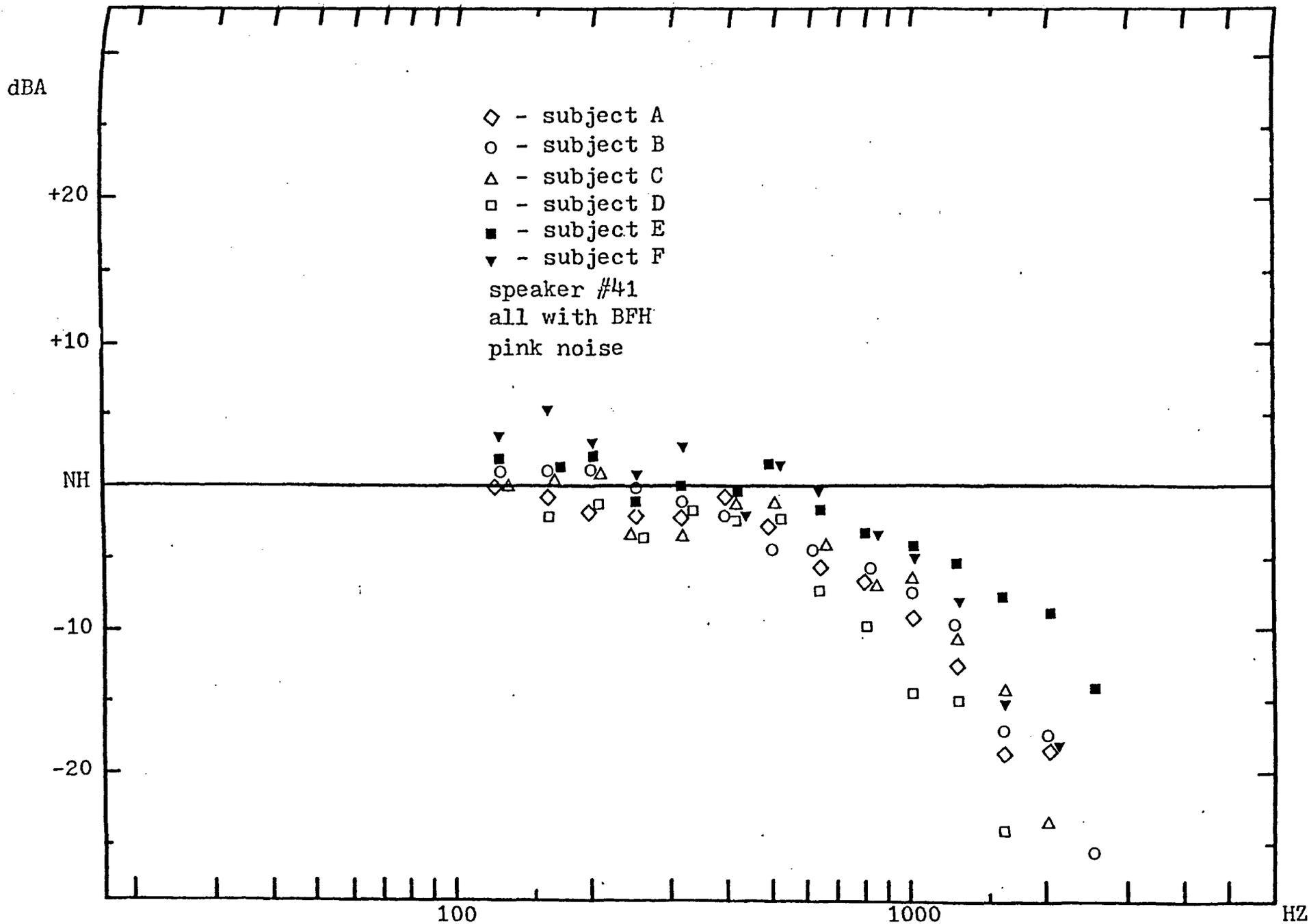
FIGURE F15 $\beta$  - 1/3 octave frequency spectrum of helmet attenuation for all subjects.
