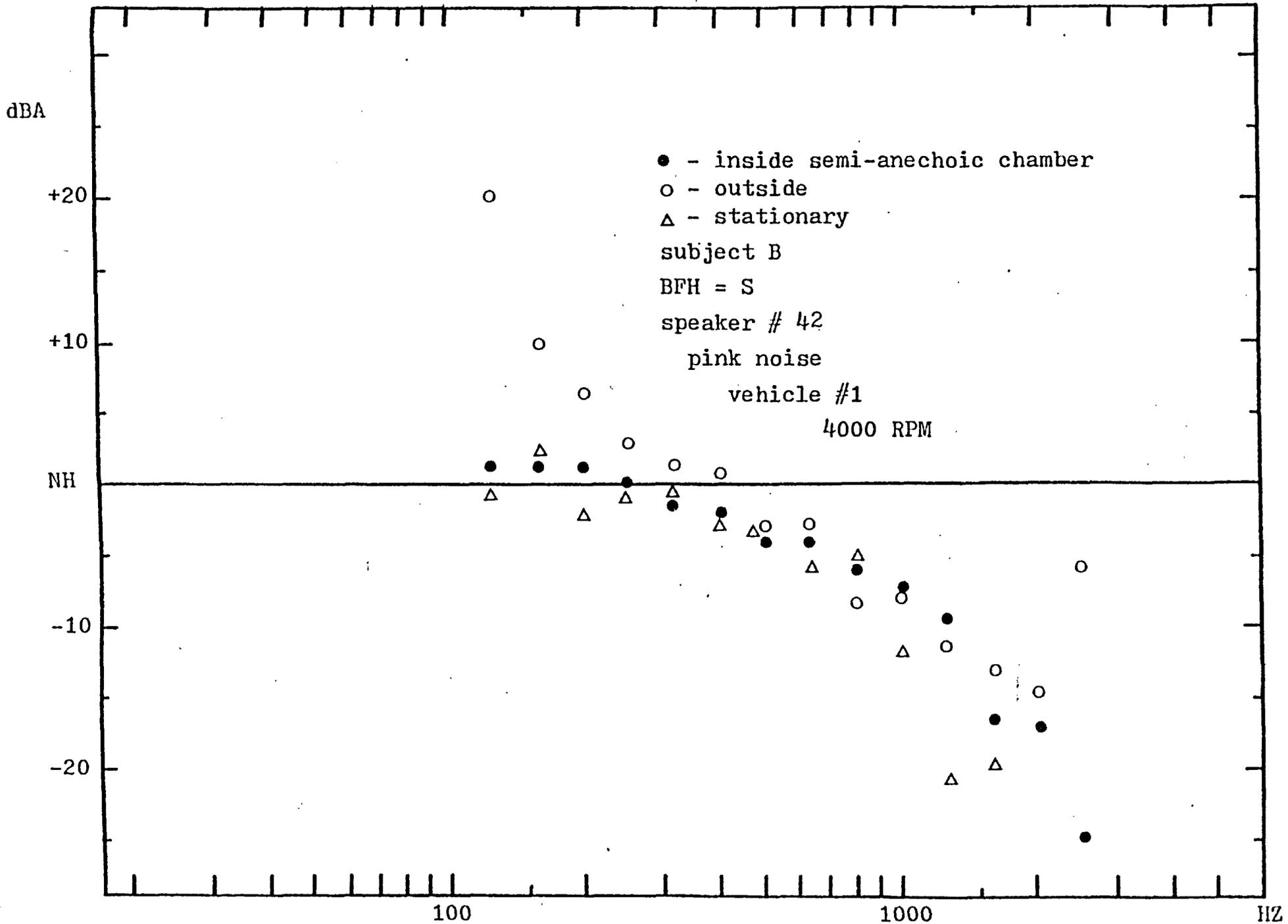
FIGURE FB2 $\beta$  - 1/3 octave frequency spectrum of helmet attenuation for inside-outside-stationary comparison.
