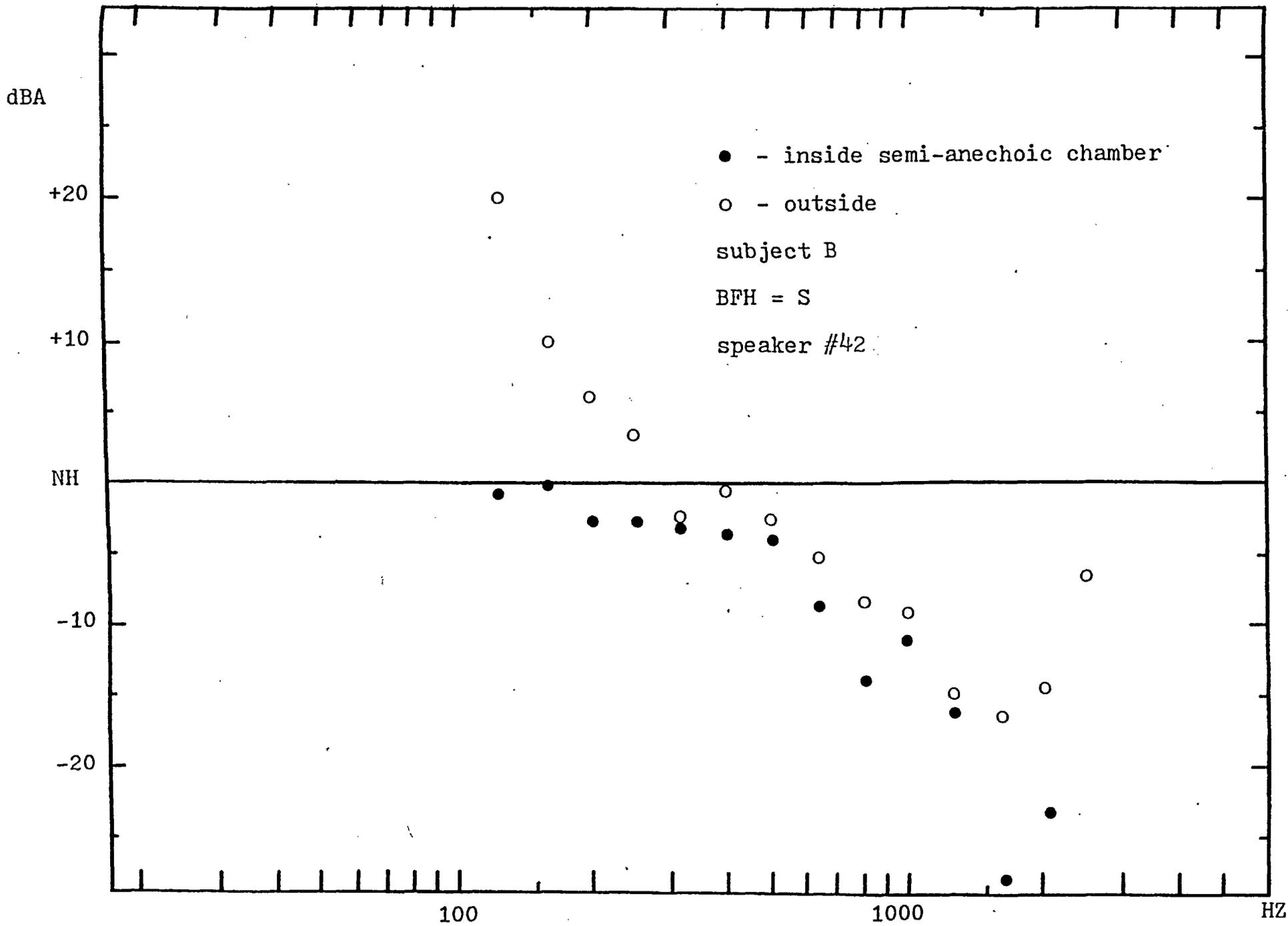
FIGURE FB17 - 1/3 octave frequency spectrum of helmet + visor attenuation for inside-outside comparison.
