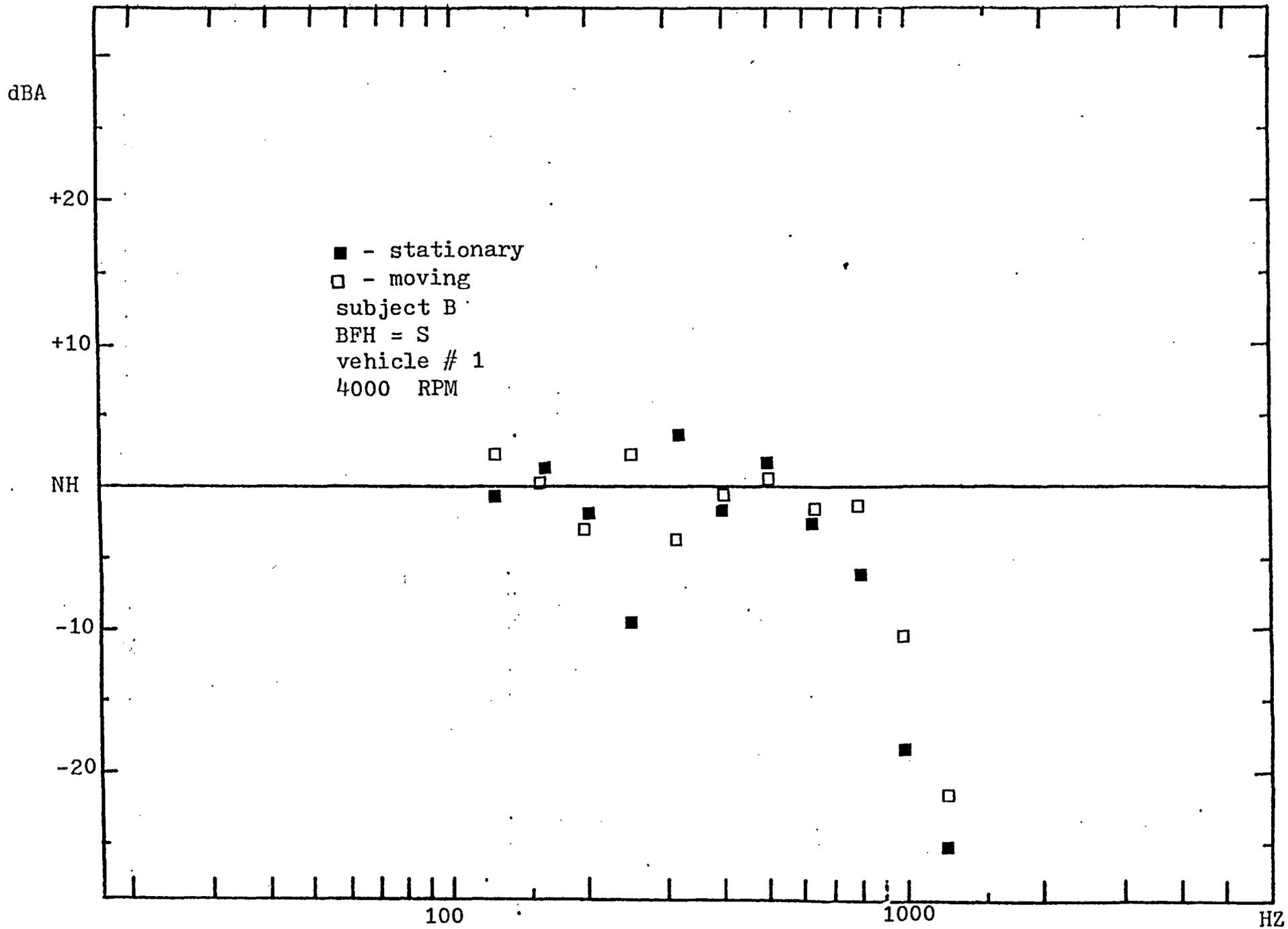
FIGURE FB3γ - 1/3 octave frequency spectrum of helmet + visor attenuation for moving versus stationary test.
