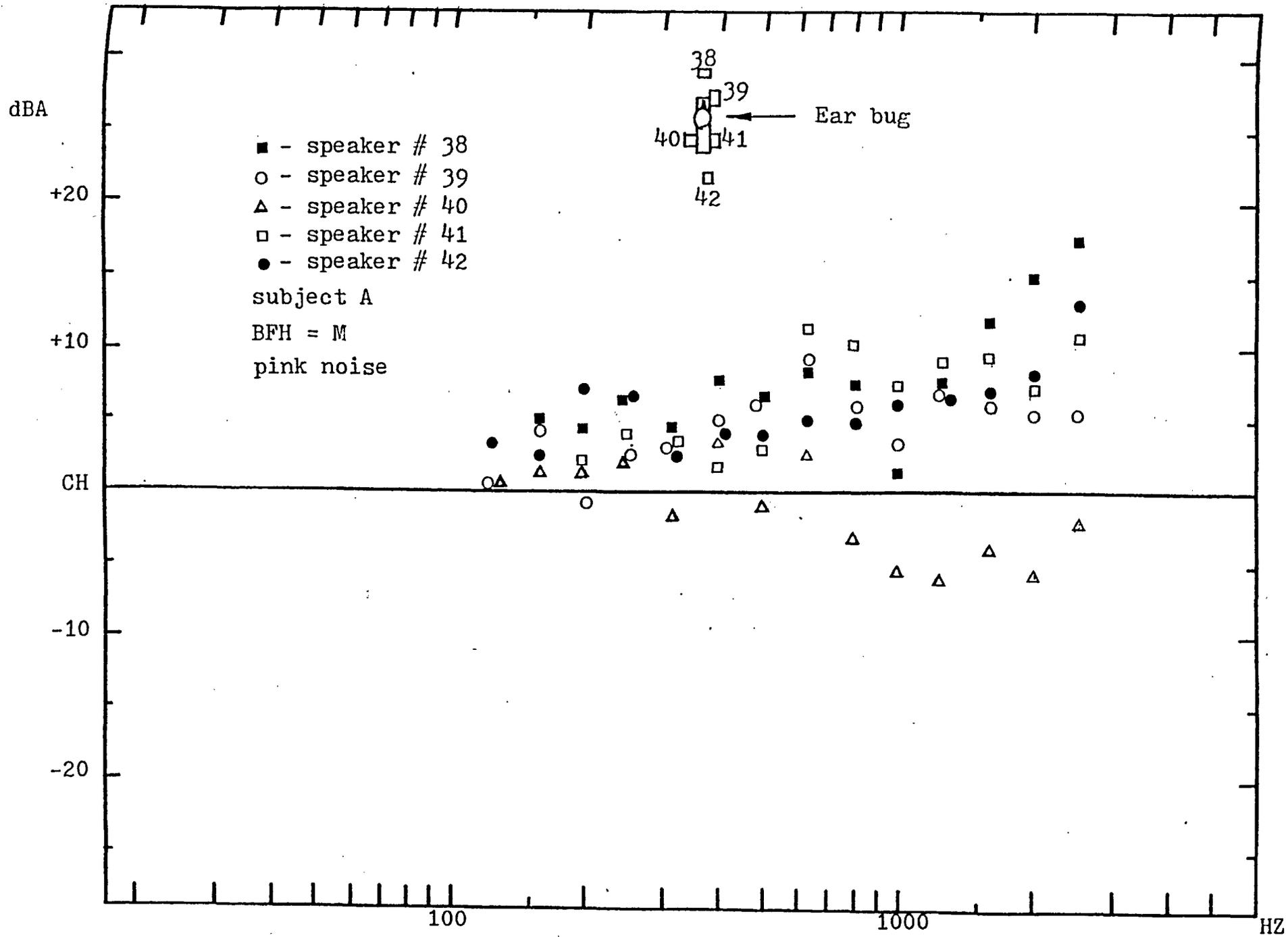
FIGURE F14 $\alpha$  - 1/3 octave frequency spectrum of transfer function for all speakers.
