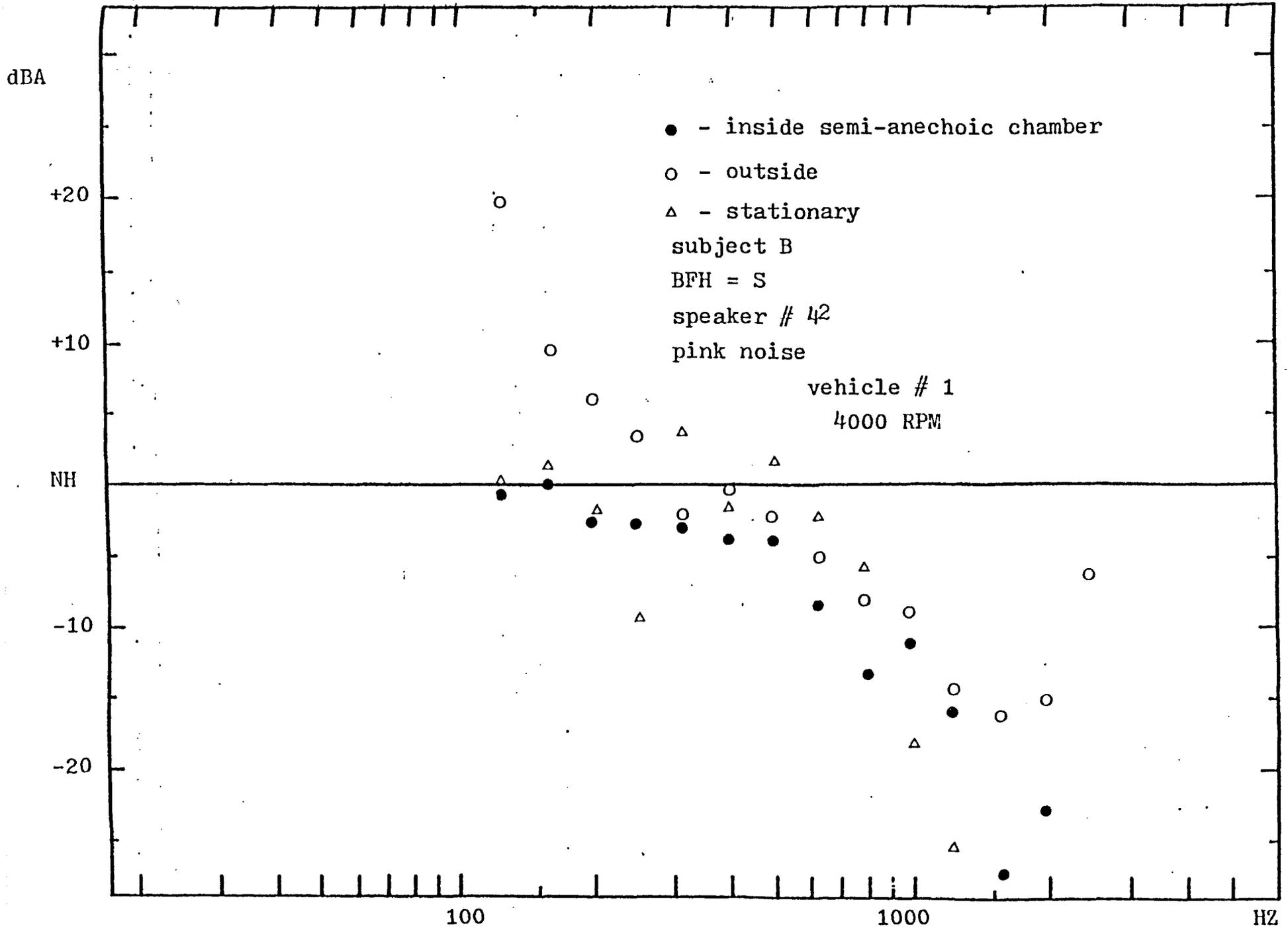
FIGURE FB28 - 1/3 octave frequency spectrum of helmet + visor attenuation for inside-outside-stationary comparison.
