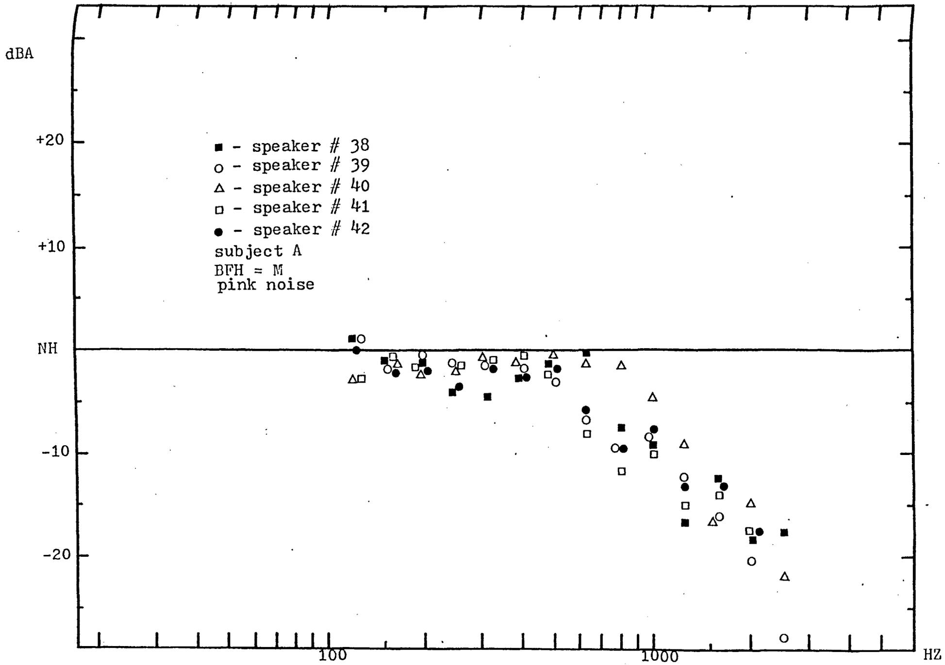
FIGURE F148 -1/3 octave frequency spectrum of helmet + visor attenuation for all speakers.
