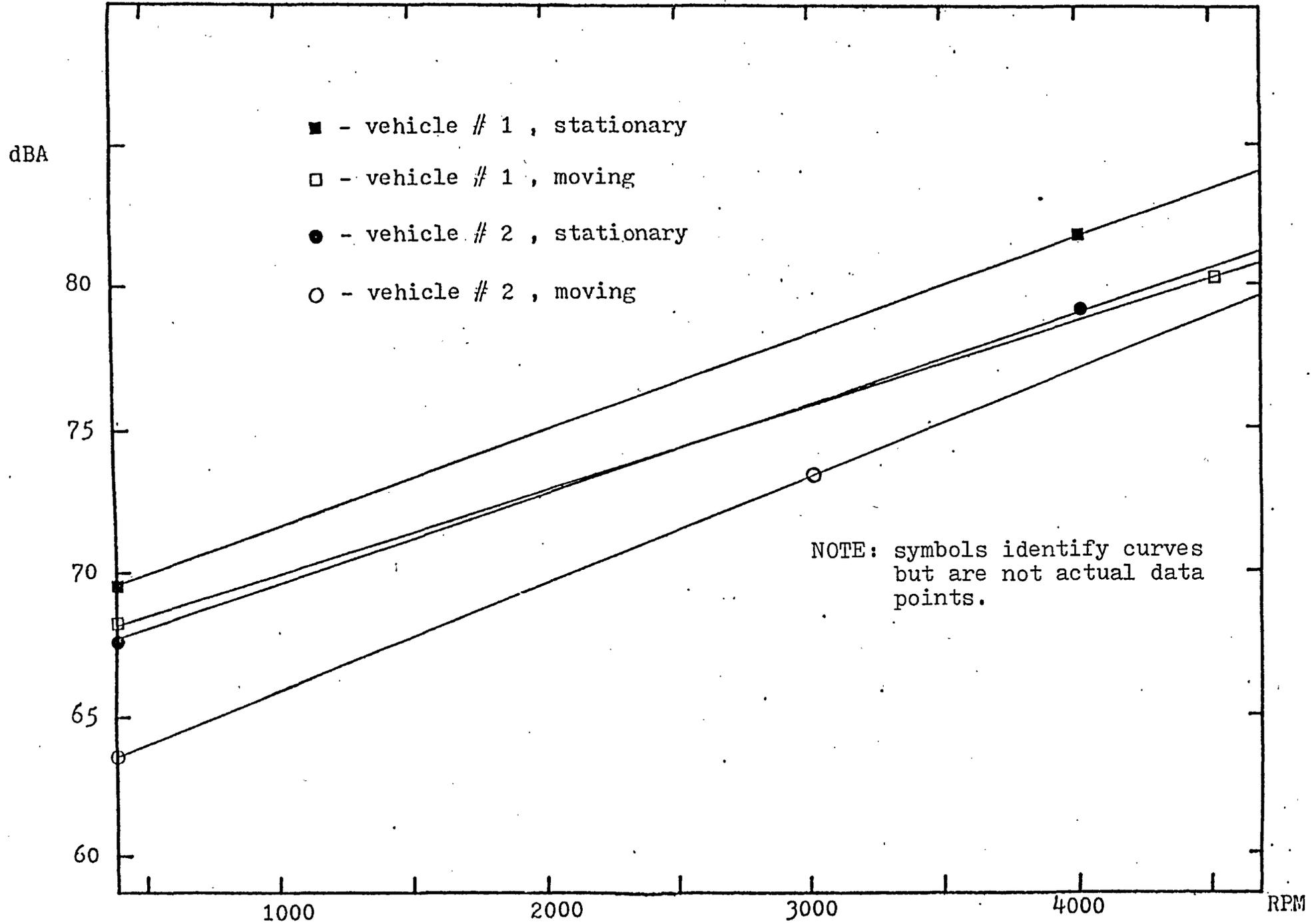
FIGURE FB5 - Plot of  $AVG_2$  of auxiliary recording results for stationary versus moving test (vehicle comparison).
