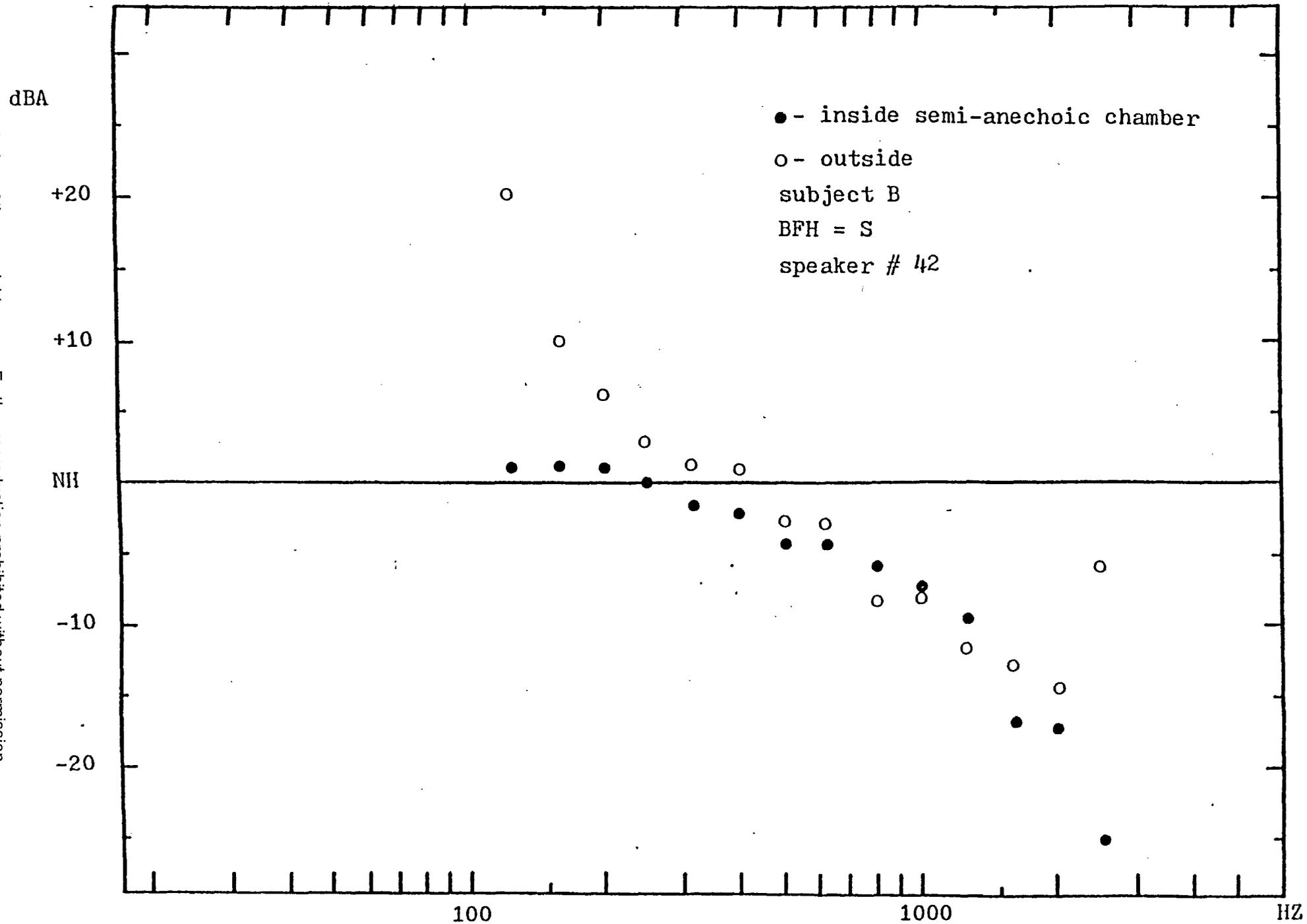
FIGURE FB1 $\beta$  - 1/3 octave frequency spectrum of helmet attenuation for inside-outside comparison.
