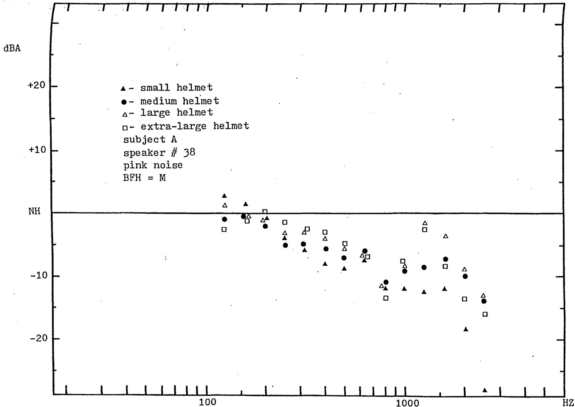
FIGURE F16 $\beta$  - 1/3 octave frequency spectrum of helmet attenuation for all helmet sizes.
