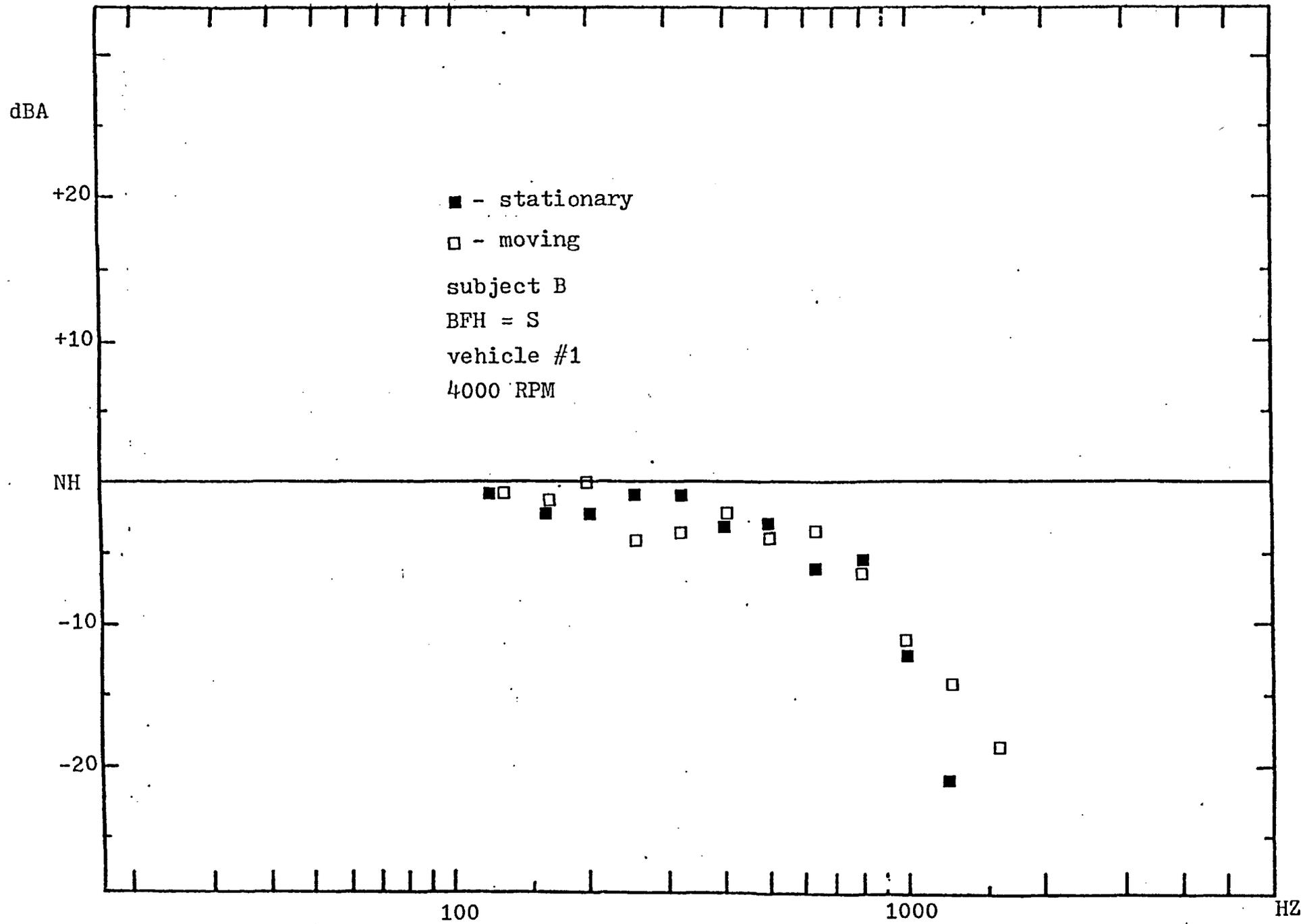
FIGURE FB3 $\beta$  - 1/3 octave frequency spectrum of helmet attenuation for moving versus stationary test.
