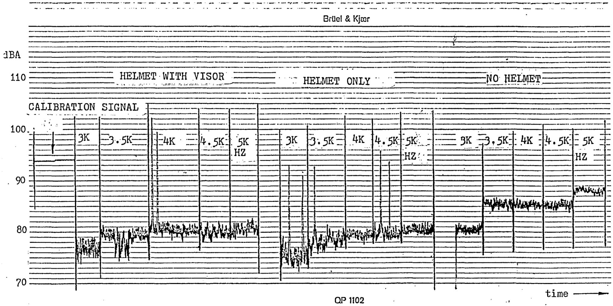
FIGURE F7- Typical Graphic Recording of Motorcycle Noise
