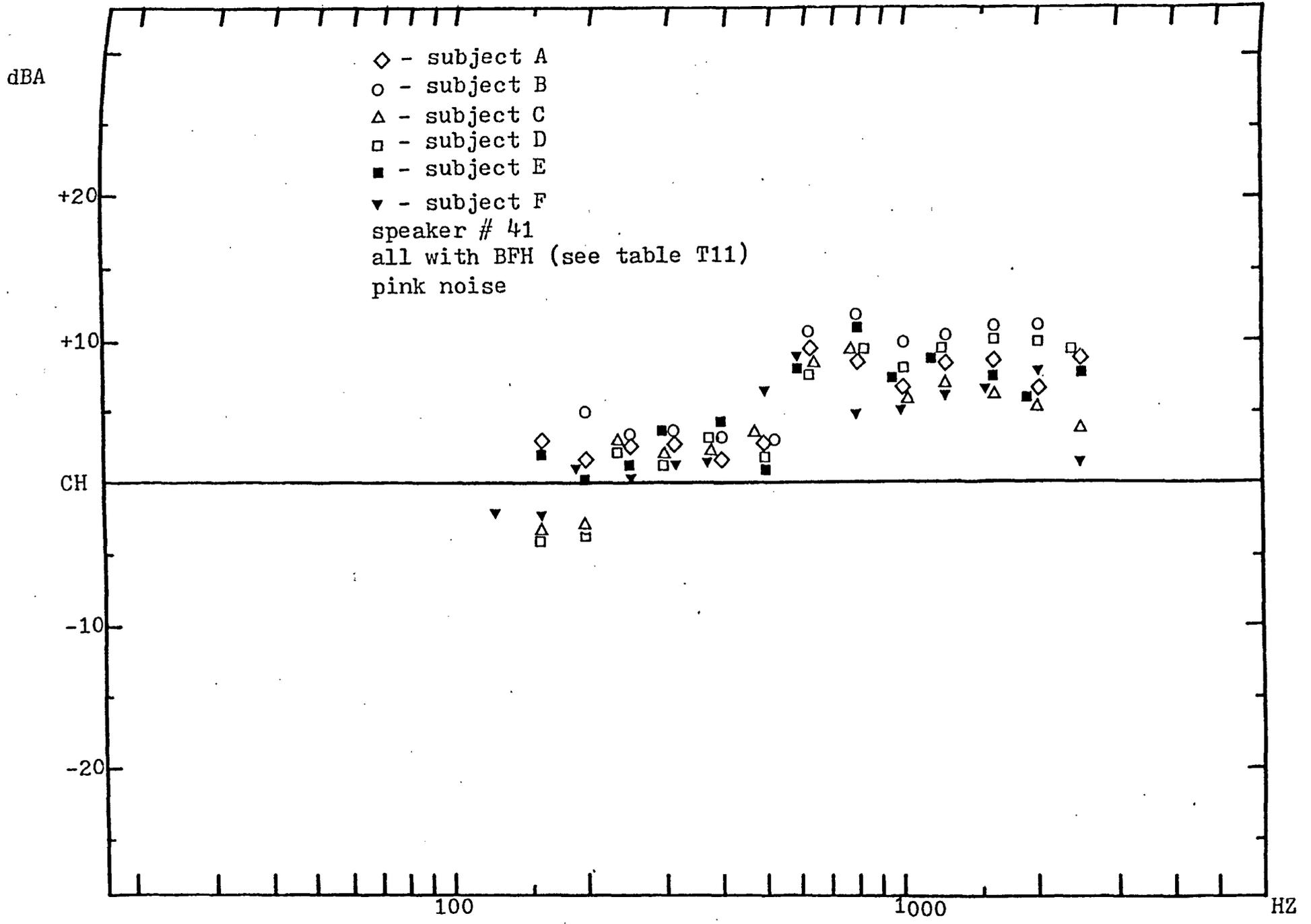
FIGURE F15 - 1/3 octave frequency spectrum of transfer function for all subjects.
