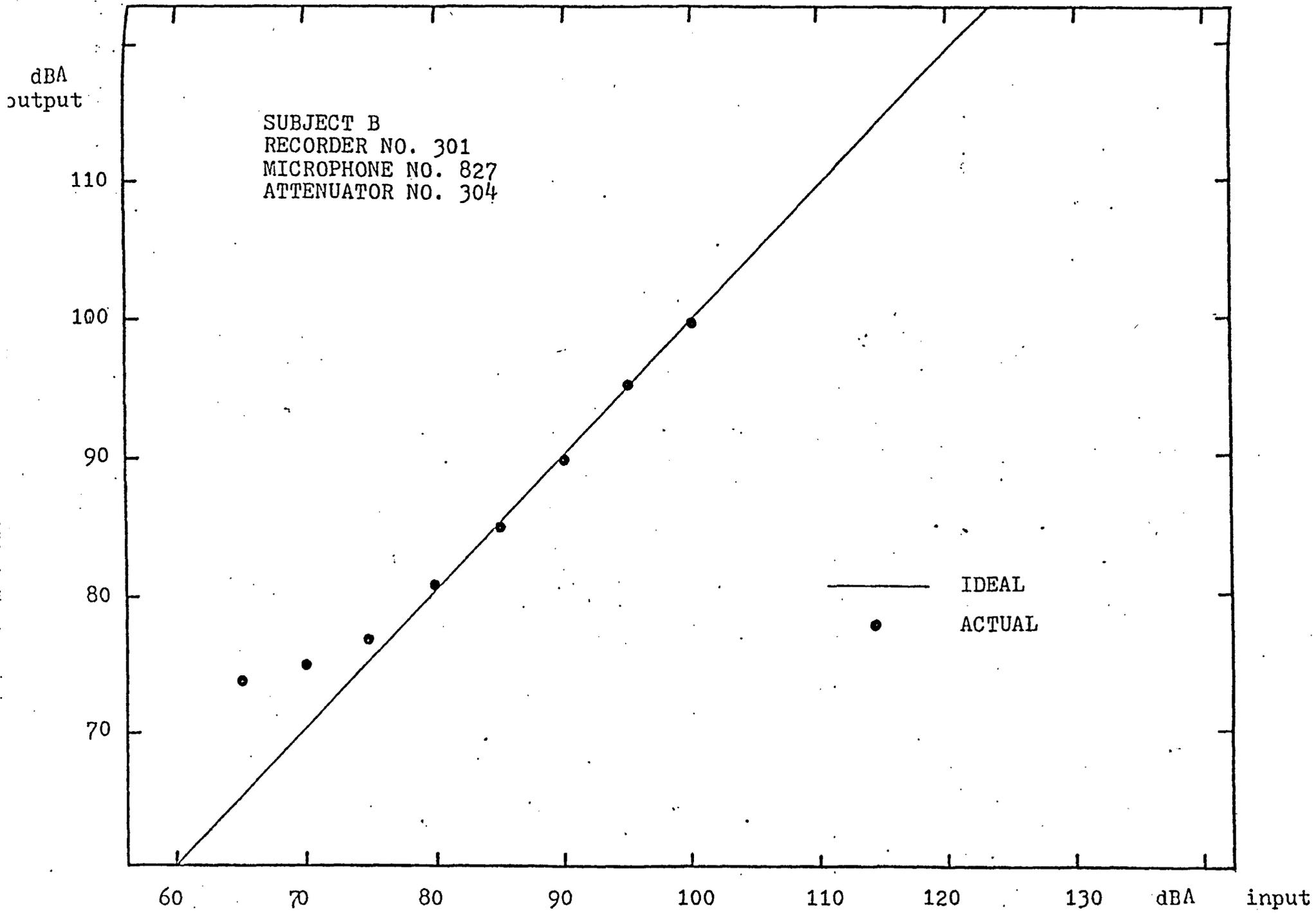
FIGURE F6- Typical dynamic characteristics of an ear bug.
