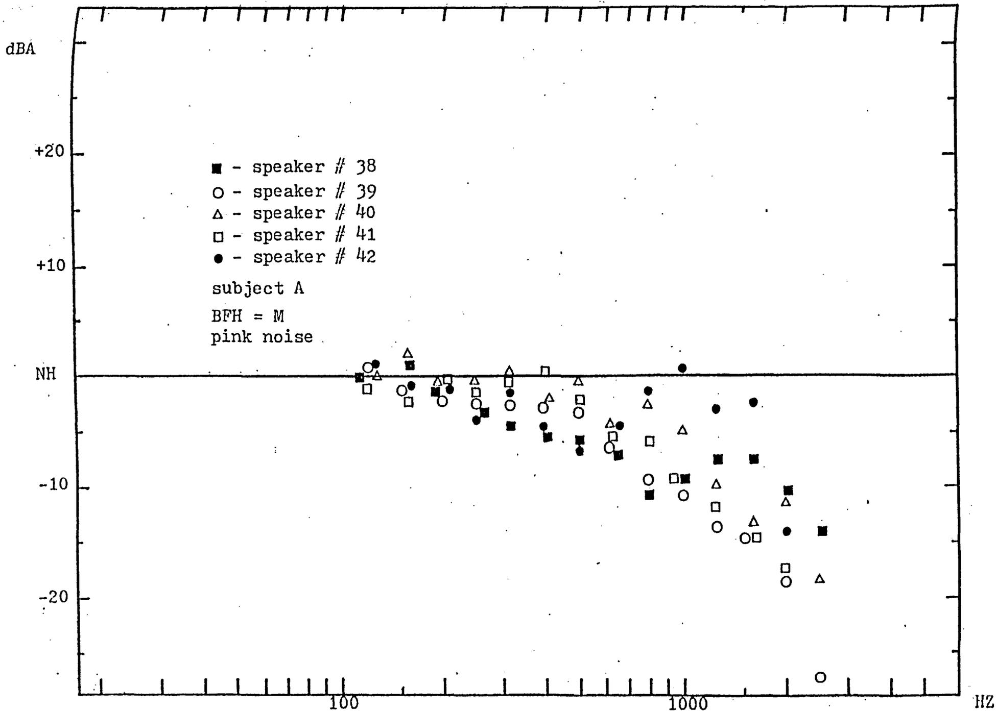
FIGURE F14β- 1/3 octave frequency spectrum of helmet attenuation for all speakers.
