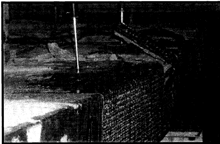
Fig. 3-68: The rehabilitated specimen (REHAB35) after failure
