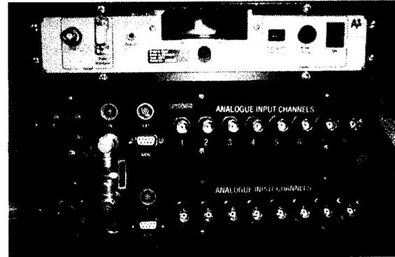
Figure 3.5: The Prosig 5600 System rear view.
