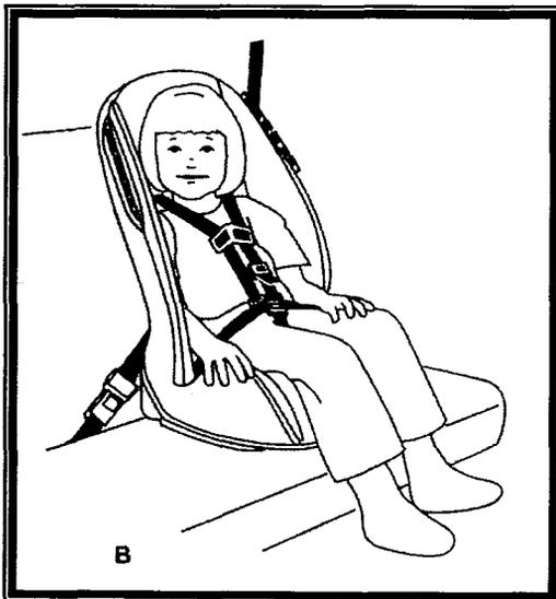
Figure 2A. Combination Child Restraint
