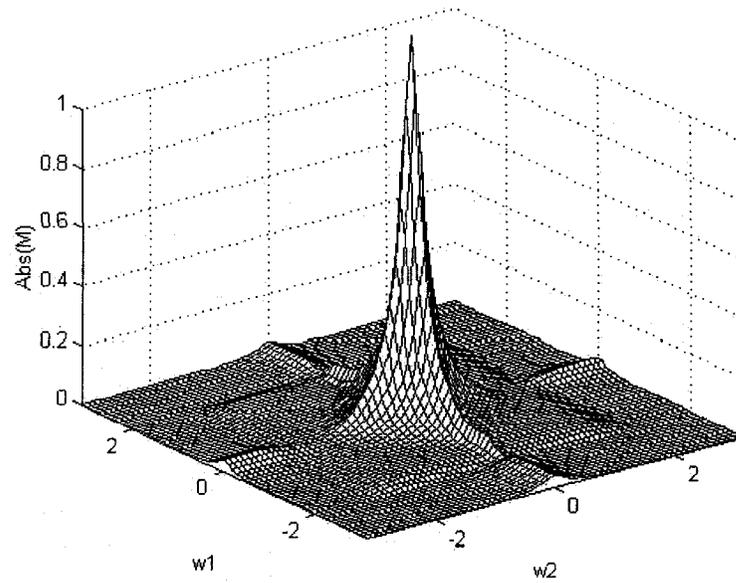
*Fig. 5.6. Amplitude Response of the 2-D Filter using Cascaded 2nd order 1-D Filters with CSD Coefficients.*
