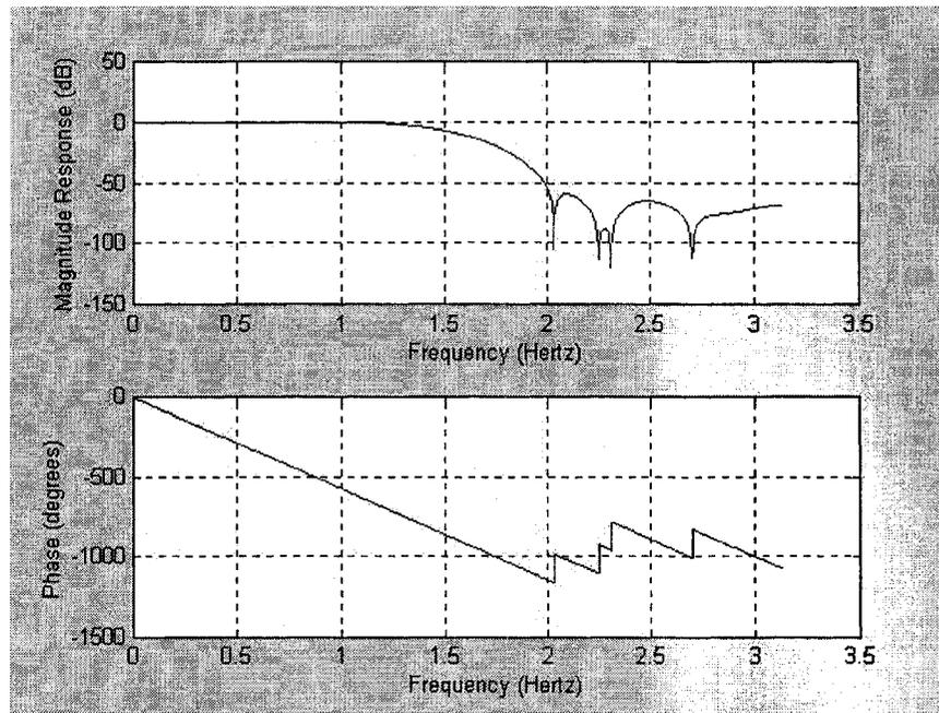
*Fig. 3.14 Response of filter with CSD coefficients converted from IP with maximum 4 non-zero digits.*
