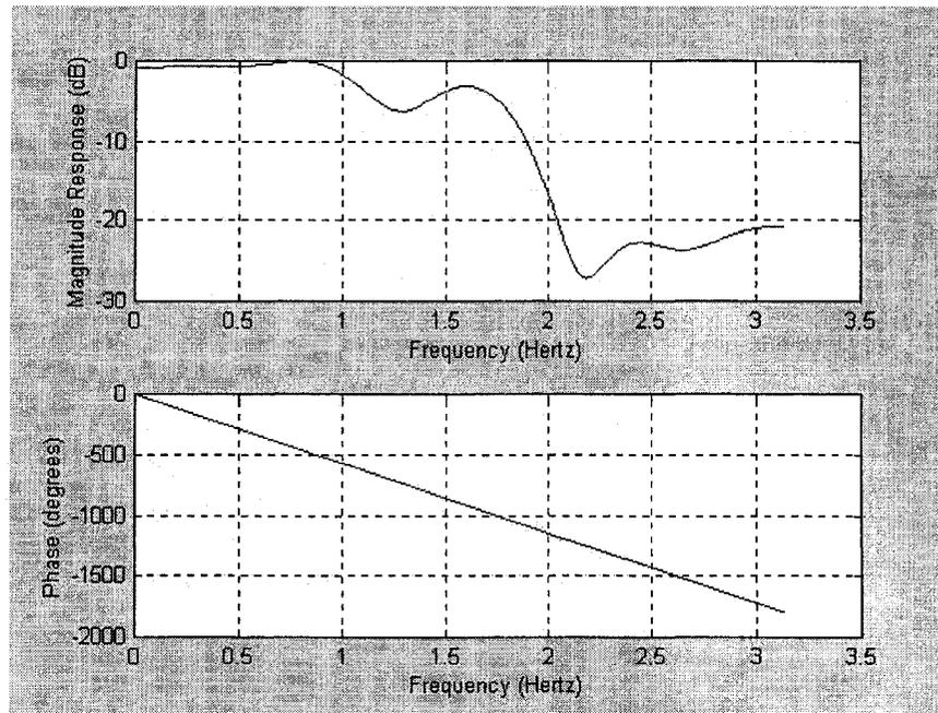
*Fig. 3.21 Response of the Filter with CSD Coefficients Designed by GA with a Maximum of 1 Non-Zero Digit*
