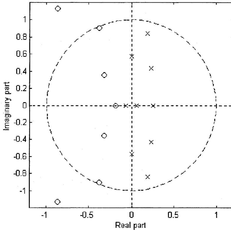
Fig. 4.2 z-Plane Plot of the Poles (X) and Zeros (O) of the Example Non-Recursive Filter
