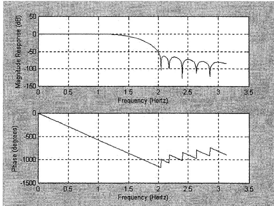
*Fig. 3.11 Response of Filter with CSD Coefficients Designed by GA with Maximum 6 Non-Zero Digits*
