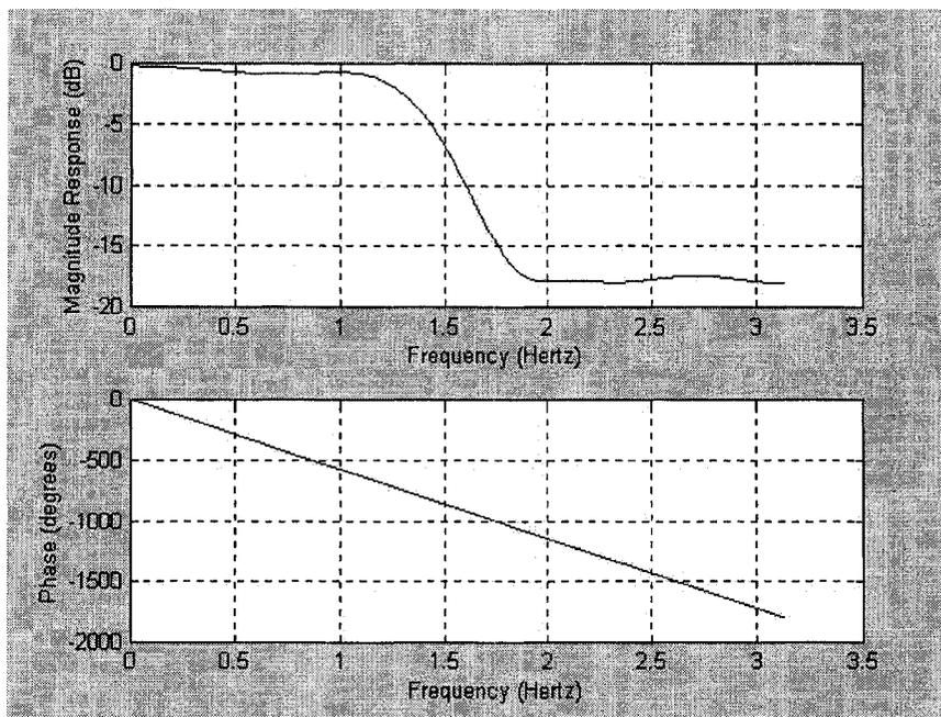
*Fig. 3.20 CSD Coefficients Converted from IP with a Maximum of 1 non-zero digit*
