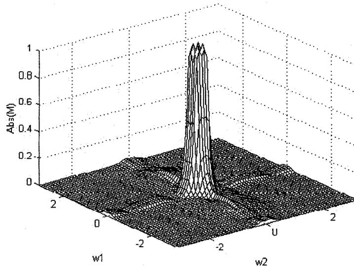
Fig. 5.8 Amplitude response of the 2-D filter using cascaded 4th order 1-D filters with CSD coefficients.
