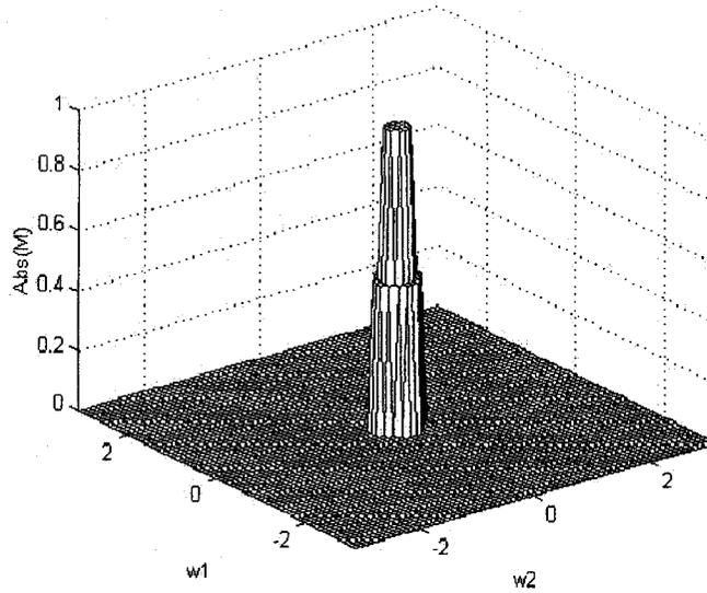
Fig. 5.5. Desired Magnitude Response of the 2-D Filter.
