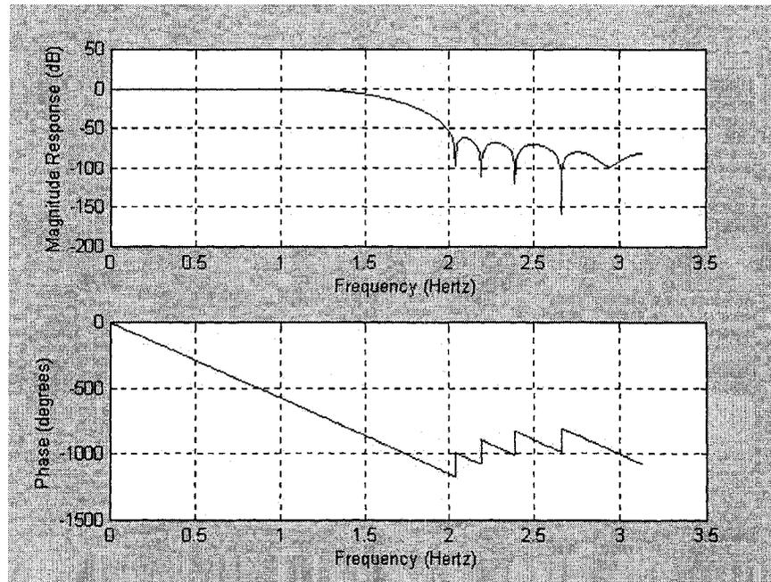
*Fig. 3.13 Response of filter with CSD Coefficients Designed by proposed GA method with a Maximum 5 of Non-Zero Digits*
