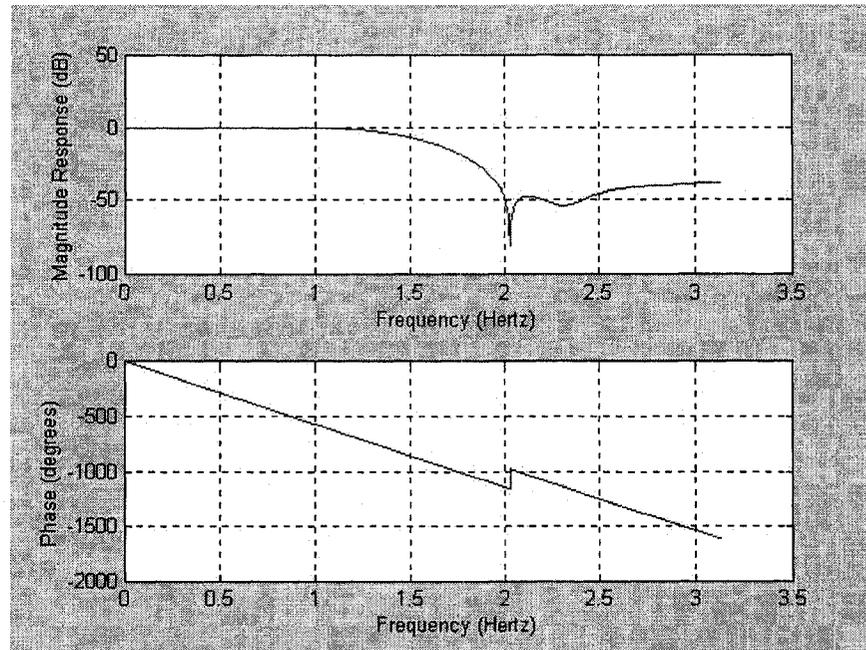
*Fig. 3.19 Response of the Filter with CSD Coefficients Designed by GA with a Maximum 2 Non-Zero Digits*
