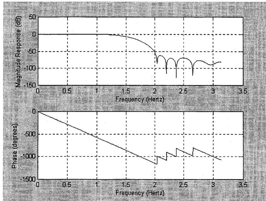
*Fig. 3.12 Response of Filter with CSD Coefficients Converted from IP with a Maximum of 5 Non-Zero Digit.*
