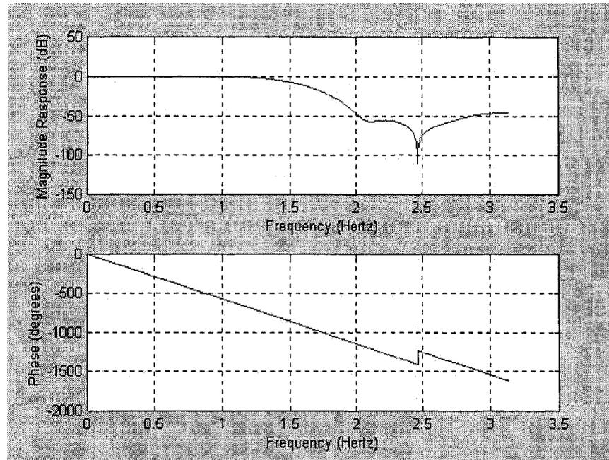
*Fig. 3.16 Response of Filter with CSD Coefficients Converted from IP with a Maximum of 3 Non-Zero Digits*
