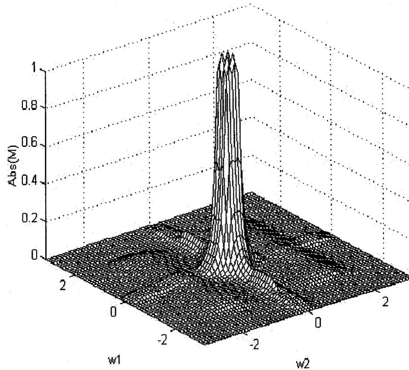
*Fig. 5.7 Amplitude Response of the 2-D Filter using Cascaded 3rd Order 1-D filters with CSD Coefficients*
