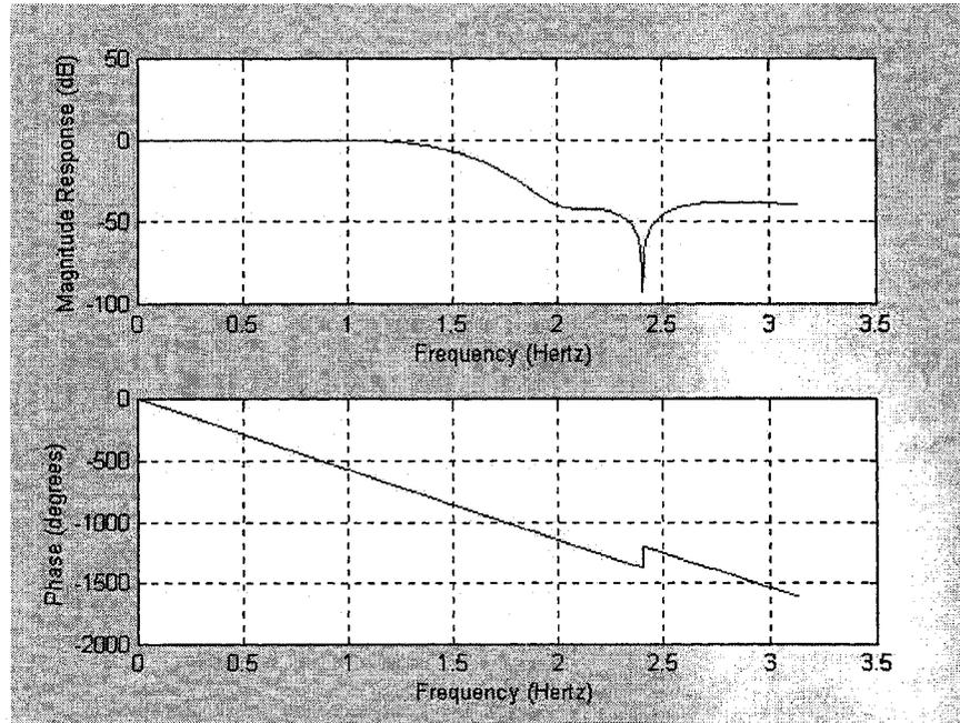
*Fig. 3.18 Response of the Filter with CSD Coefficients Converted from IP with a maximum of 2 Non-Zero Digits*
