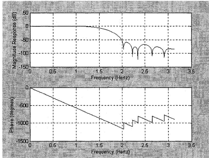
*Fig. 3.15 Response of filter with CSD coefficients designed by GA with maximum 4 non-zero digit.*
