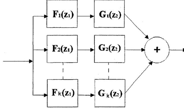
Fig. 5.1 Cascaded 1-D Filters Form a 2-D Filter
