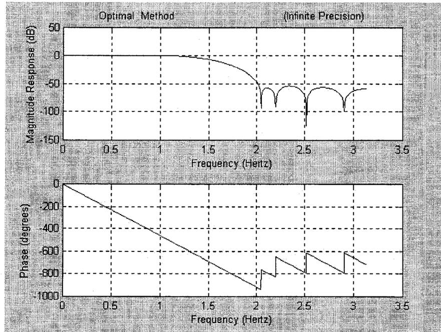
*Fig. 3.5 Response of Optimal Design using IP Coefficients*
