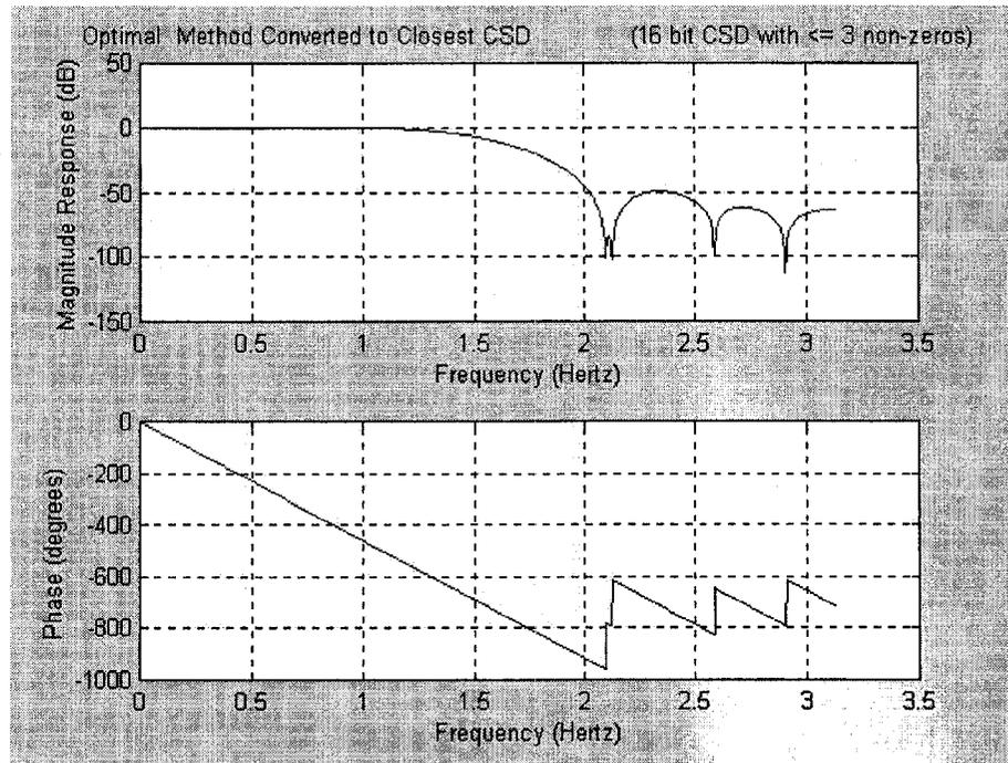
Fig. 3.6 Response of Optimal Design Converted to CSD Coefficients
