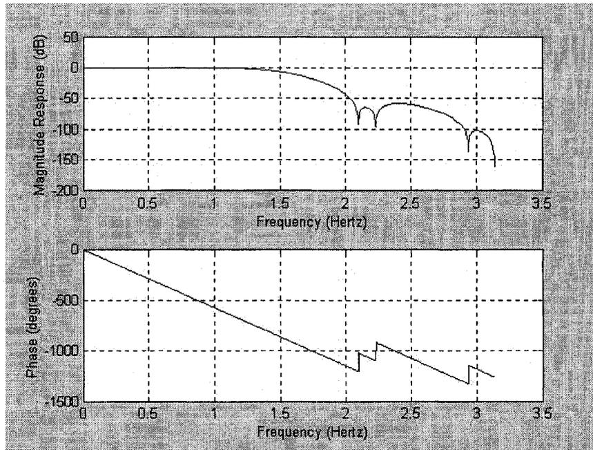
*Fig. 3.17 Response of the Filter with CSD coefficients Designed by GA with a Maximum 3 Non-Zero Digits*
