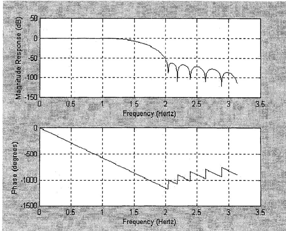
Fig. 3.9 Response using Infinite Precision Coefficients
