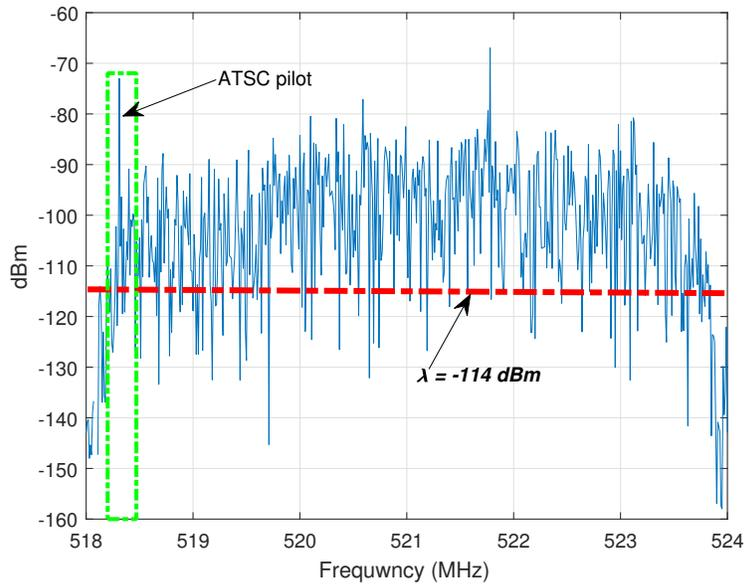
Figure 4.12: Observed pilot-tone for channel 22
