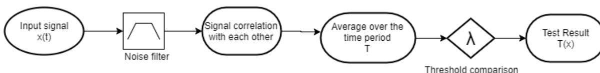
Figure 2.9: Block Diagram of CS detection scheme
