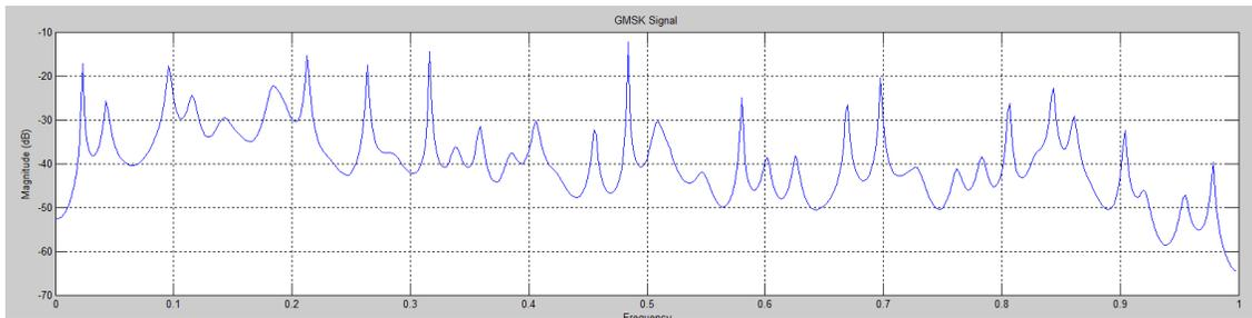
(c) Gaussian Minimum Shift Keying Modulated Signal
