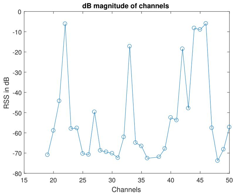
Figure 4.17: Received Signal Strength of Channel 19 to 50
