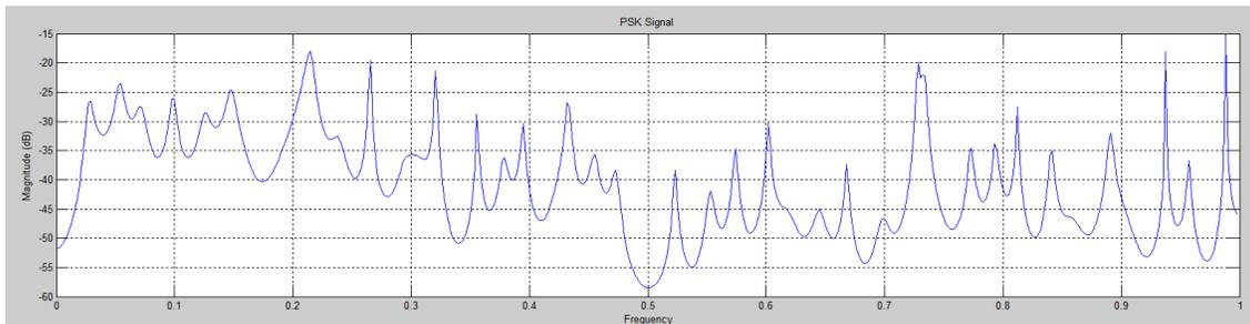
(b) Phase Shift Keying Modulated Signal
