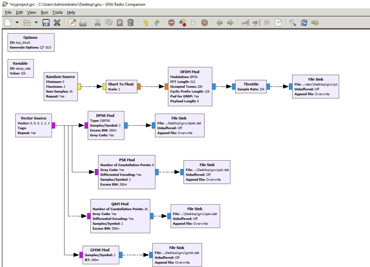
Figure 3.4: GNU Radio Program for data generation
