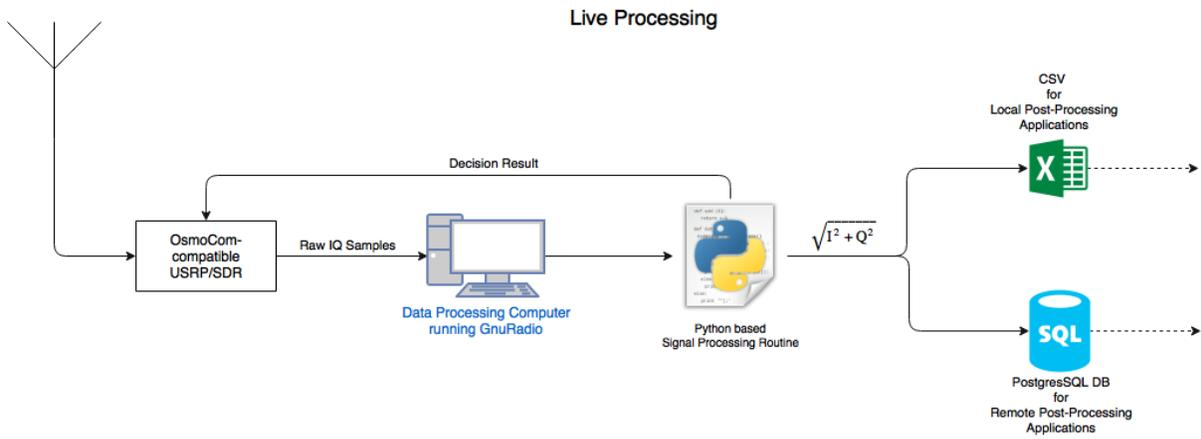
(a) Detected signals pre-processing flowchart
