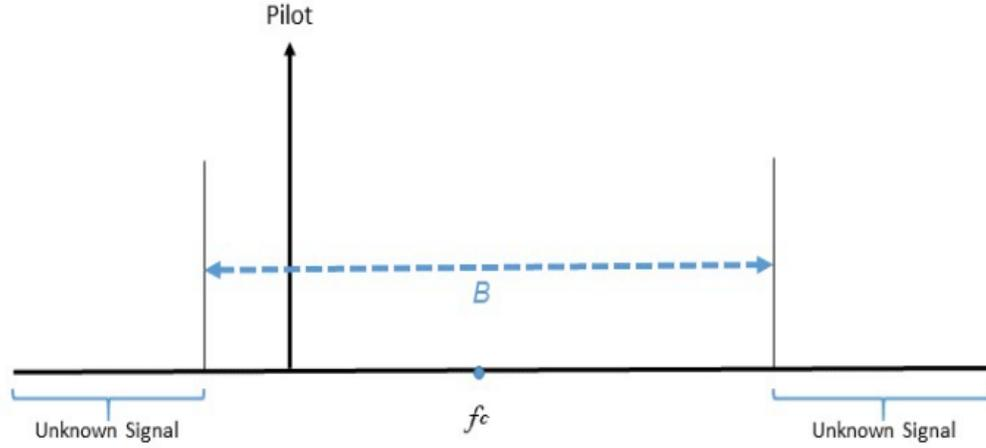
Figure 2.6: Pilot Signal in Spectrum
