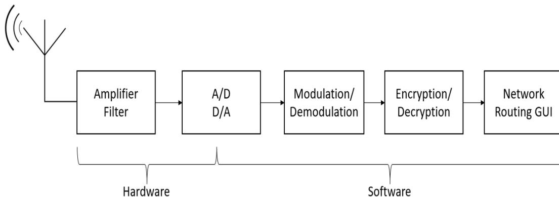
Figure 2.2: A simple Software Defined Radio
