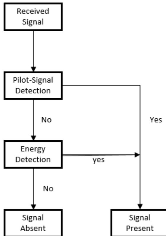
Figure 3.5: Block Diagram of Two step spectrum sensing Technique
