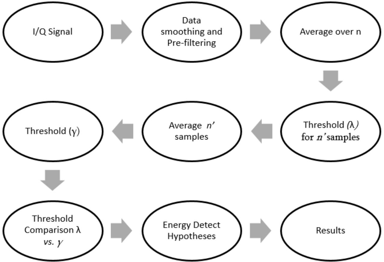
Figure 3.8: Block Diagram of Utilized Sensing Algorithm
