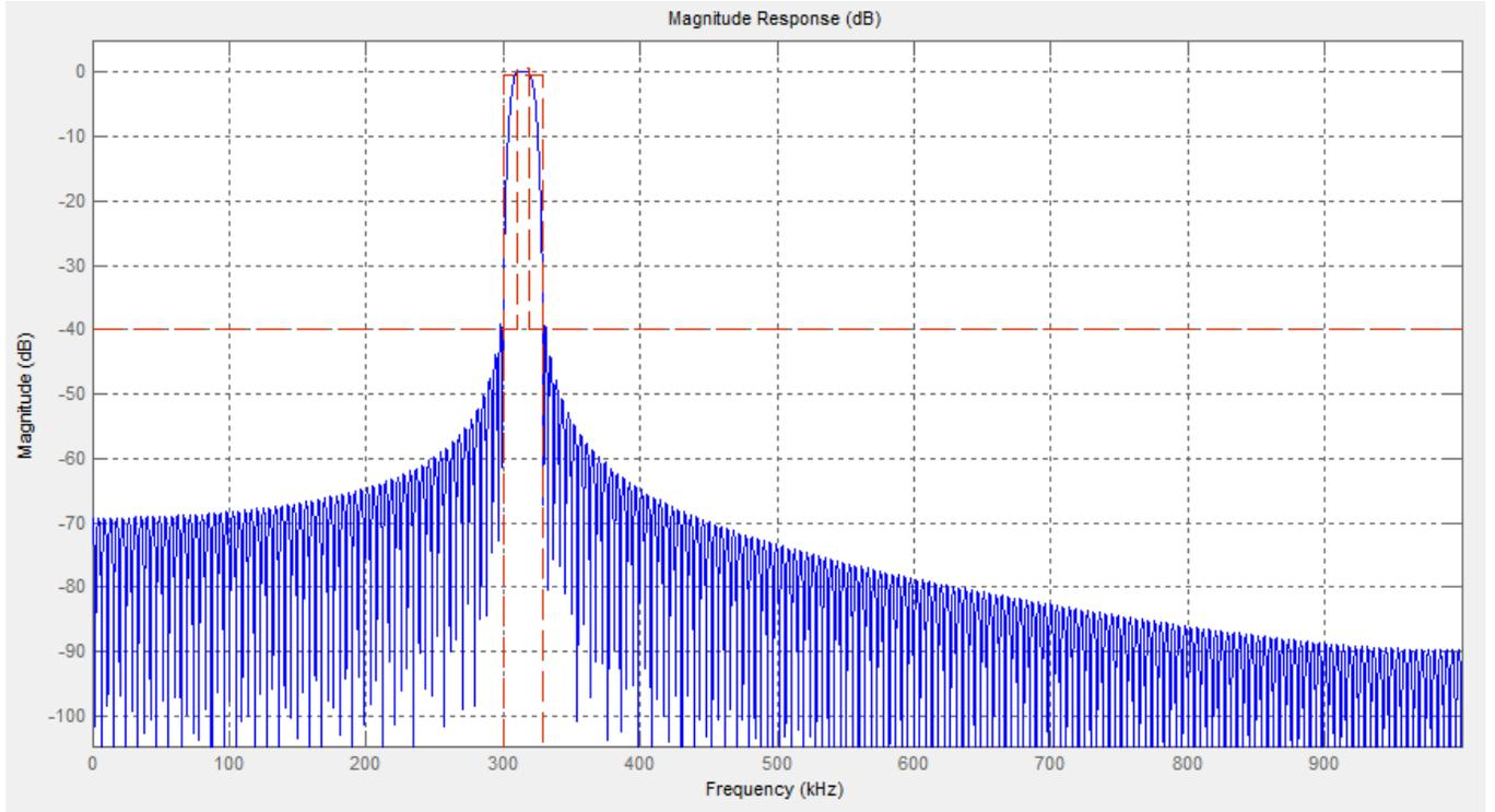
Figure 3.7: Magnitude Response of Band-pass filter
