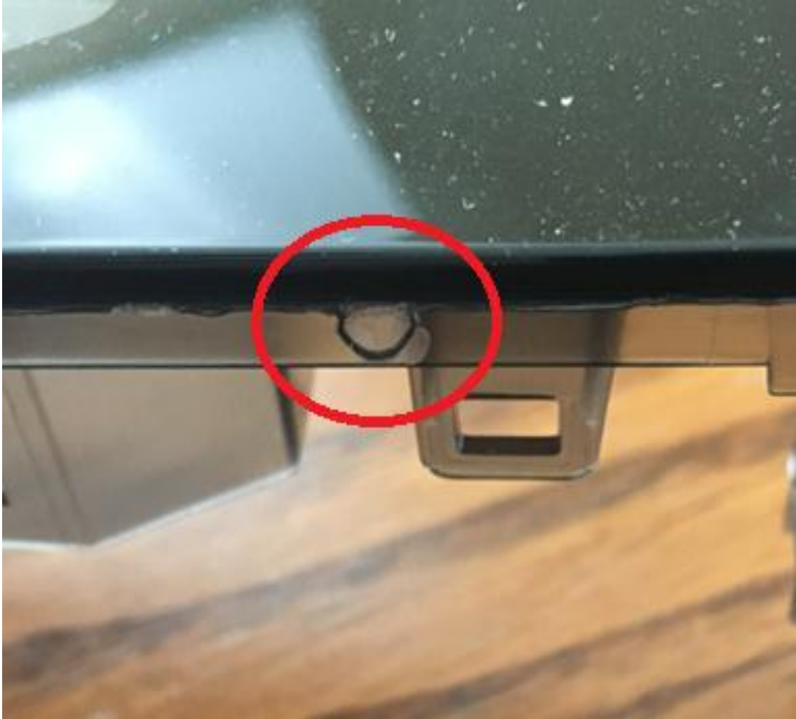
Figure 10: Representation of flash of the resin. Some injected resin flowed out from the edges when it was still hot.
