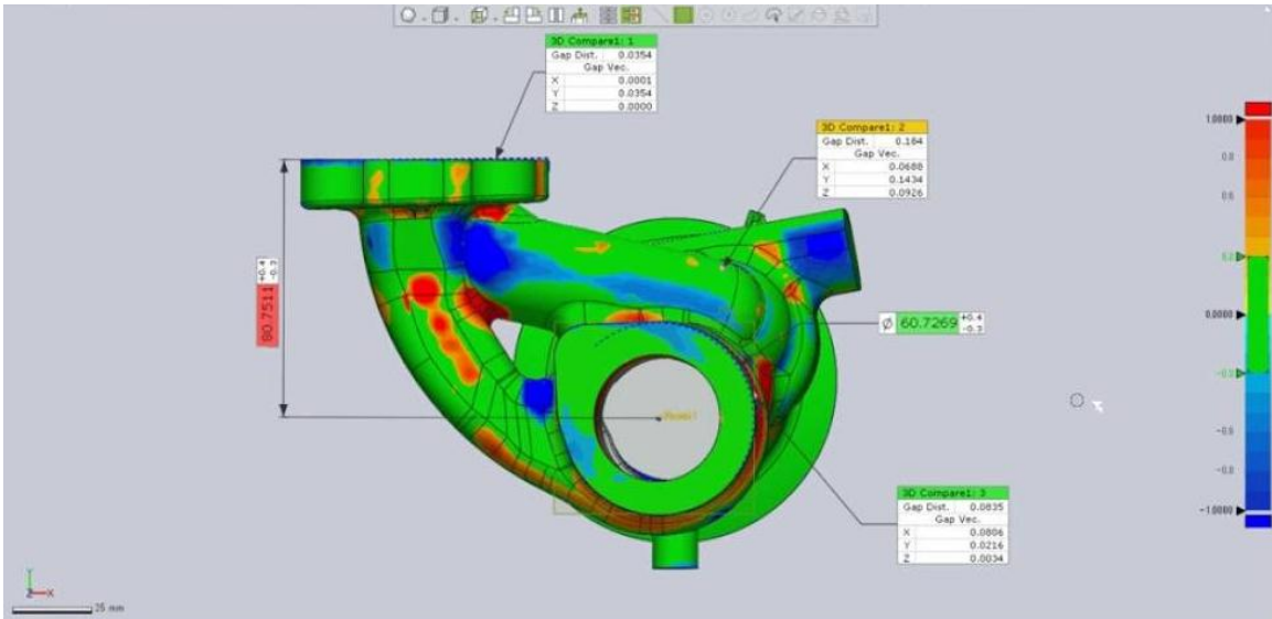
Figure 17: Color map as outcome of the Software Geomagic Control X [41]
