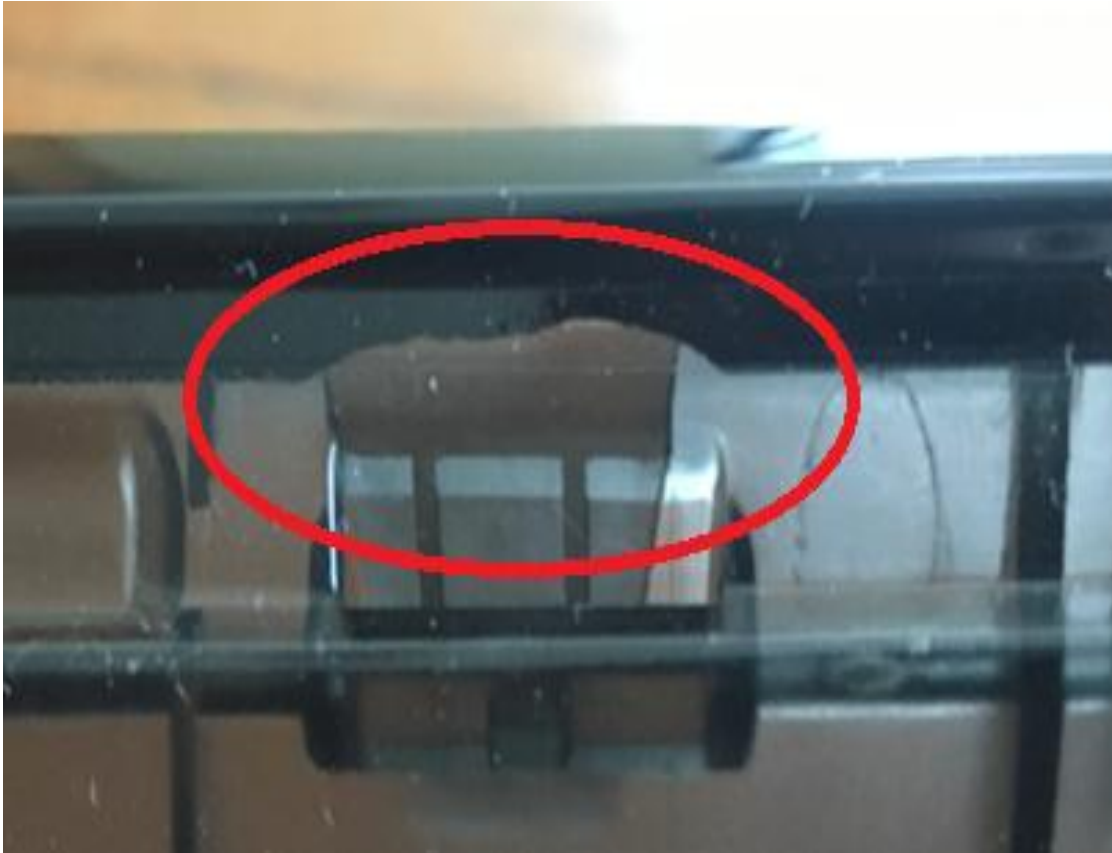
Figure 11: Representation of a ripped edge of the film, showing an improper contour.
