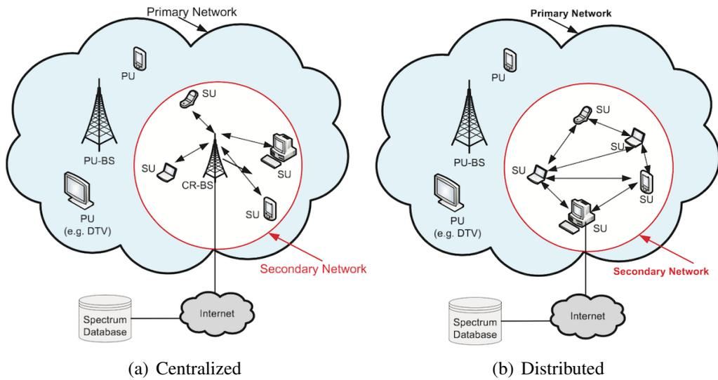
Figure 2.3: Cooperative spectrum sensing topologies.
