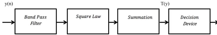
Figure 2.1: Block diagram of Energy detector.
