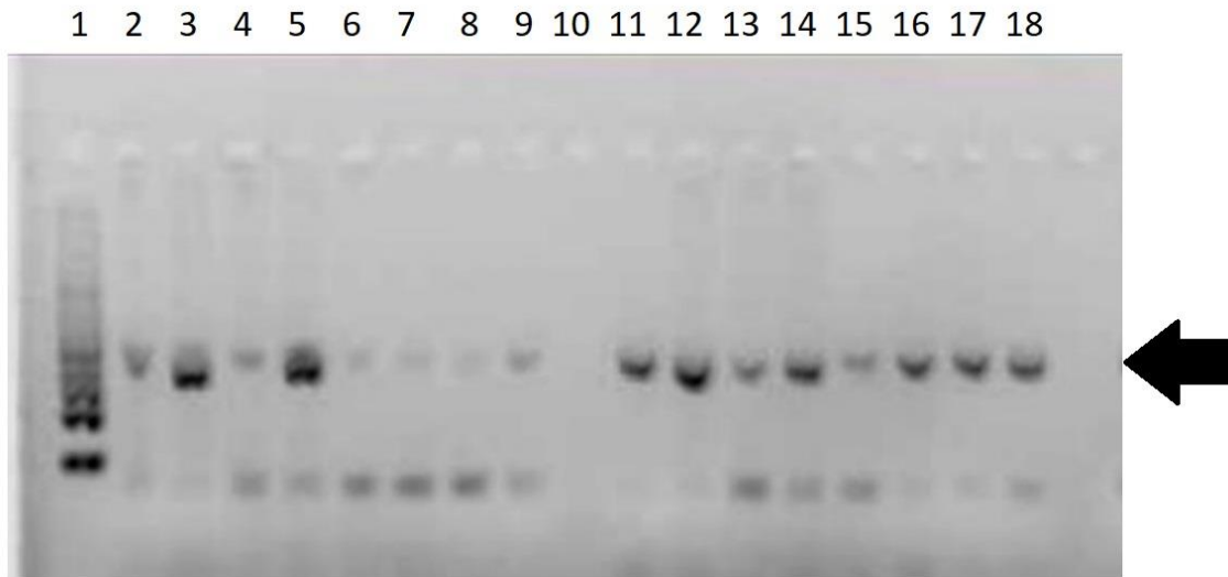
Figure 7: Positive detection of zebra mussel DNA (mtDNA COI amplification) in sensitivity test. Bands on agarose gel are amplified DNA (arrow). Lane 1: Ladder (100bp); Lane 2 to 5: One veliger; Lanes 6 to 9: One veliger + other plankton and particles; Lane 11 to 14: Three veligers; Lanes 15 to 18: Three veligers + other plankton and particles.
