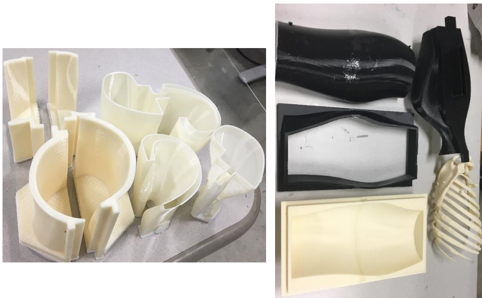
Figure 4.5-7 (a): Split optimized mould set for 2-year old male patient representation, (b): Adhered mould set for 18-year old female patient representation
