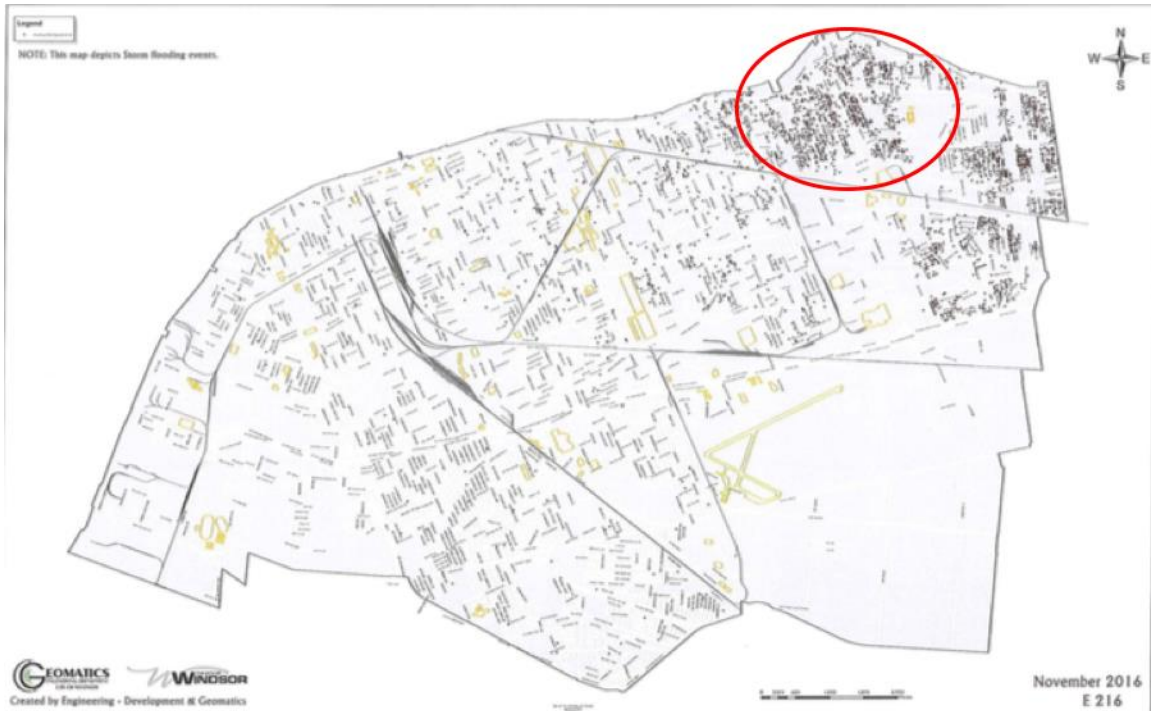
Figure 3-6 Reported basement flooding after storm event in 2016 (The City of Windsor, 2017).
