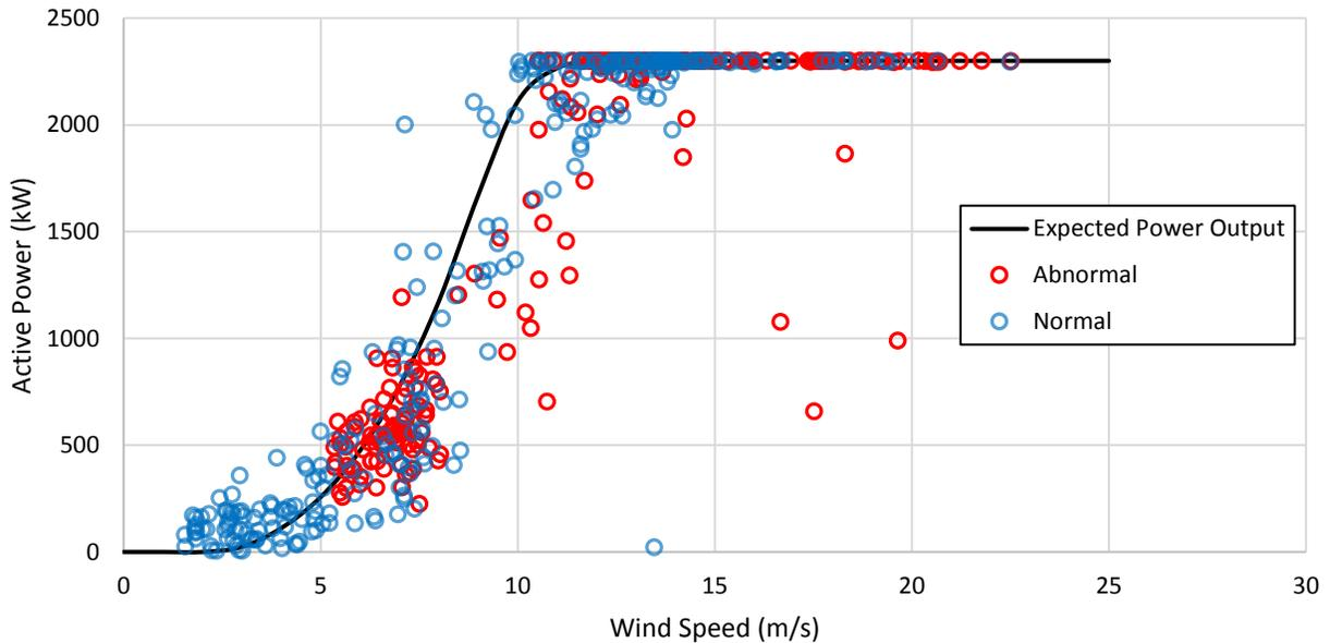
Figure 3. 5: Power curve comparison for wind turbine 1.
