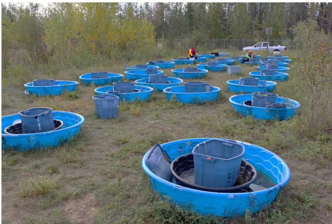
Fig. 2.3: Mesocosms set up at the Experimental Trench Complex showing the 3 x 10 experimental setup, the precipitation mesocosms and the DO calibration mesocosms used in Chapter 3 and additional mesocosms constructed for a parallel study by Boudens et al. (2016).
