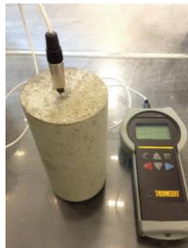
Figure 3.5. Testing procedure for thermal conductivity
