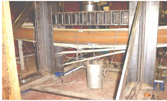
Figure 1.3: Failure mode observed in the rehabilitated beams (El Damatty et al.)
