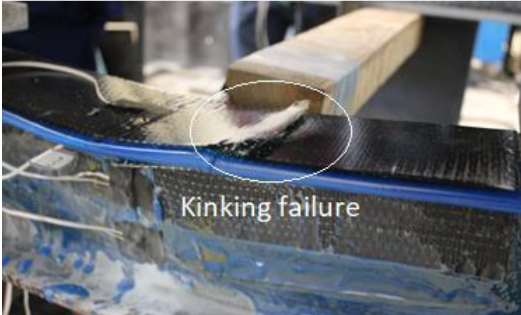
Figure 3.11: Kinking along the stress concentration line
