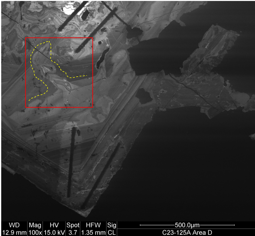
Figure 4.21 Red box denoting a dissolution feature in Sn-related fluorite I that has crosscut earlier growth zones.
