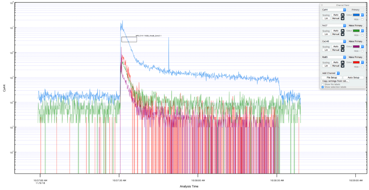
Figure 4.54 Laser ablation spectra of a zone of W-related fluorite with numerous REE-mineral inclusions, illustrating the uniformity of the spectra.
