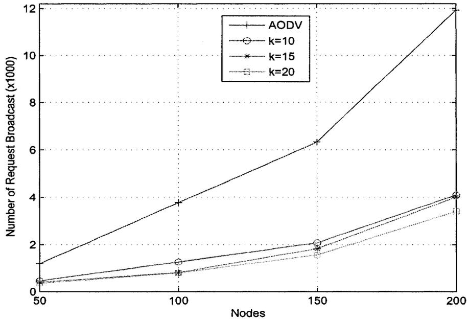
**Figure 3.4: Broadcast reduction with varying values of k**
