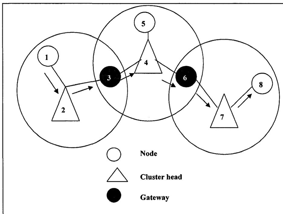
**Fig 2.1: CGSR: routing from node 1 to 8**
