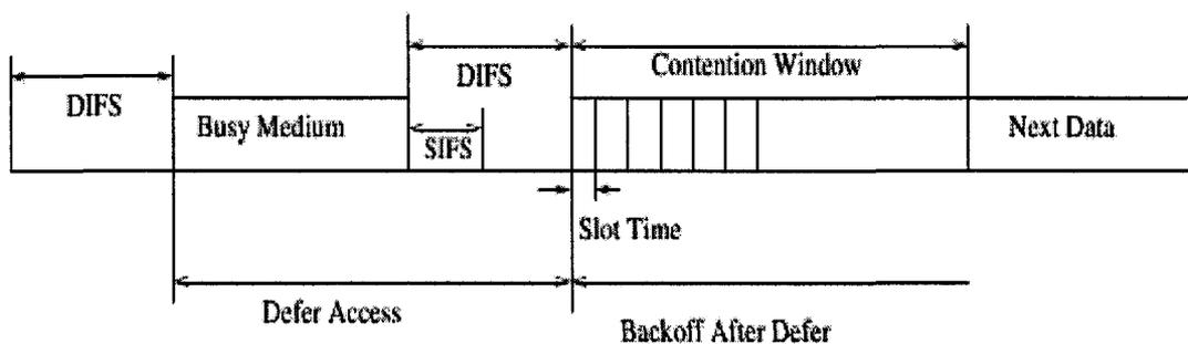
**Figure 3.7: Basic access mechanism in IEEE 802.11**
