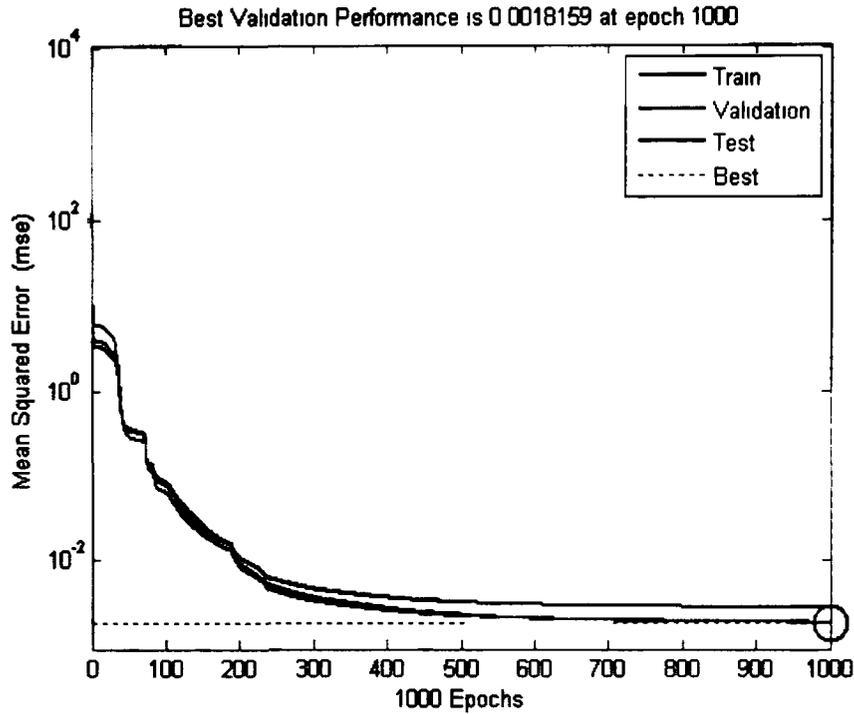
Figure 5.30. Error curve for 100% loss in torque (1 s).
