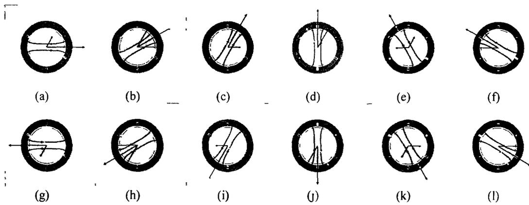
Figure 2.4. Rotating magnetic field of a synchronous machine.
