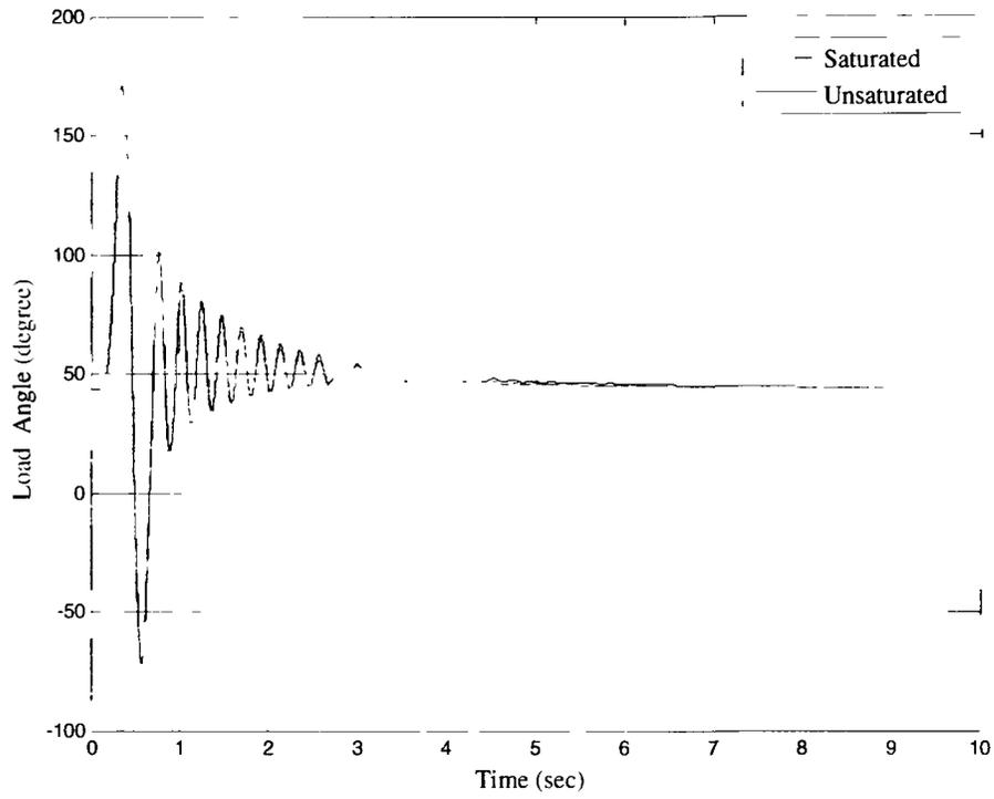
**Figure 4.21. SC for 0.212 s (Marginally Stable).**
