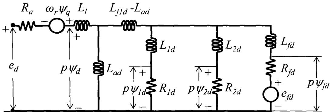
Figure 2.7. d-axis circuit diagram.
