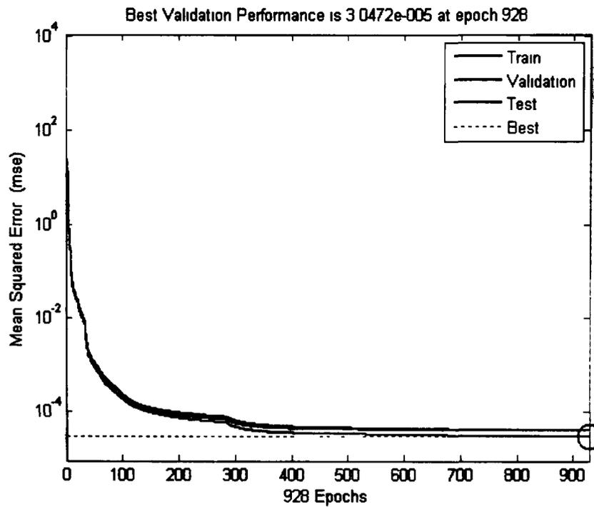
Figure 5.24. Error curve for 100% over-excitation in DIT (0.1 s).
