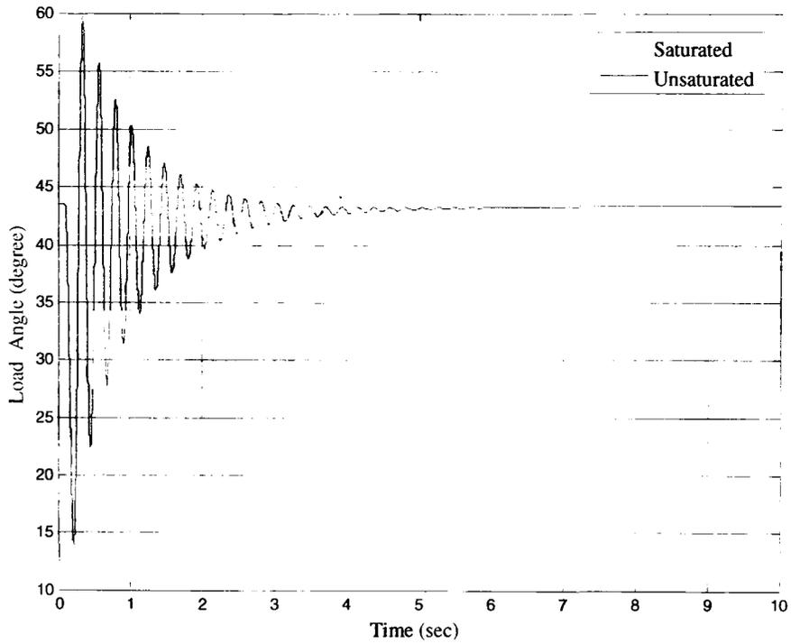
**Figure 4.13. 100% loss of DIT for 0.1 s.**
