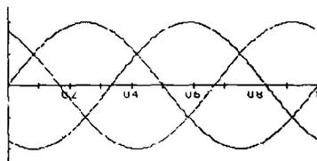
Figure 2.2. Three-phase AC signal.
