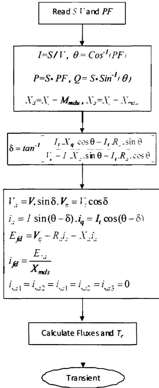
Figure 4.1. Initial value calculation flowchart for unsaturated model.
