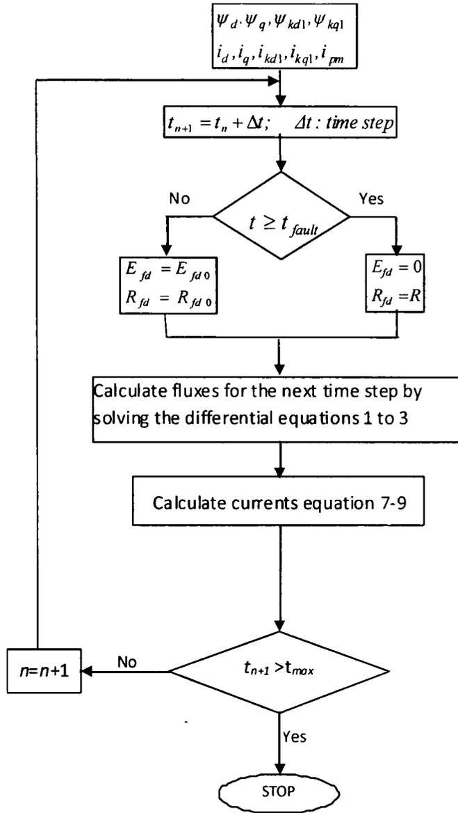
Figure 4.3. Calculation of transient values after LOF fault for unsaturated model.
