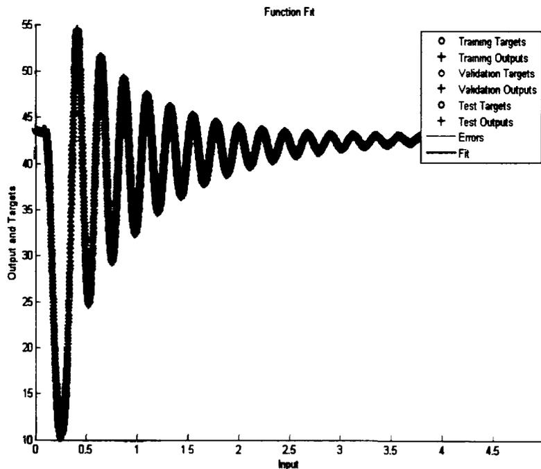
**Figure 5.25. Approximation for 100% loss in torque (0.2 s).**
