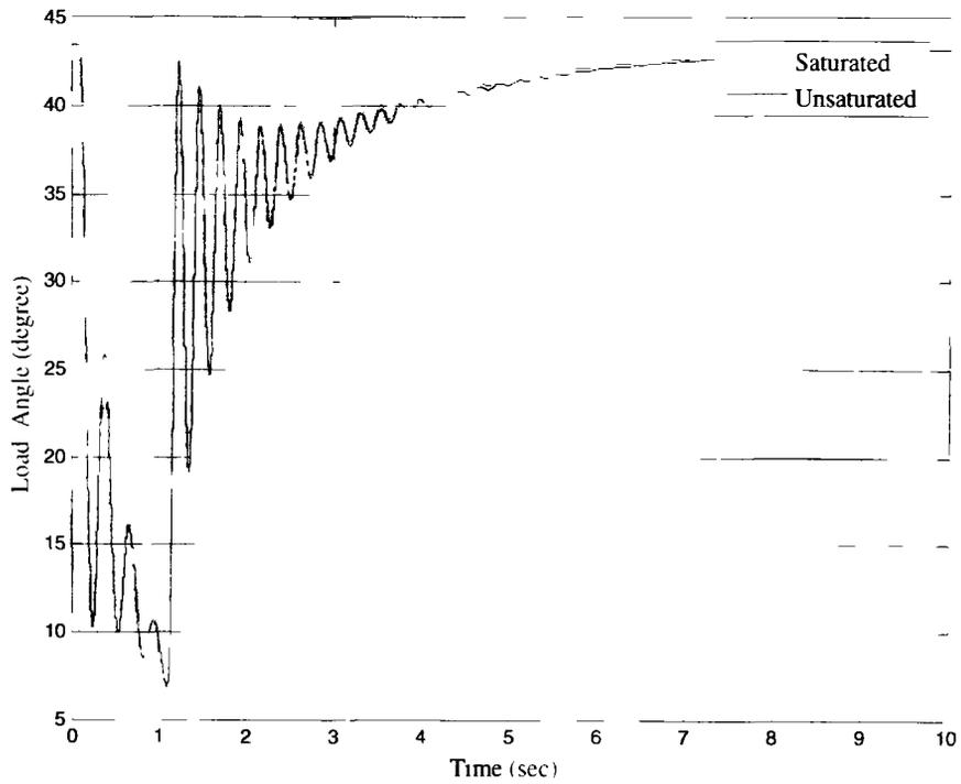
**Figure 4.18. 100% loss of DIT for 1 s.**
