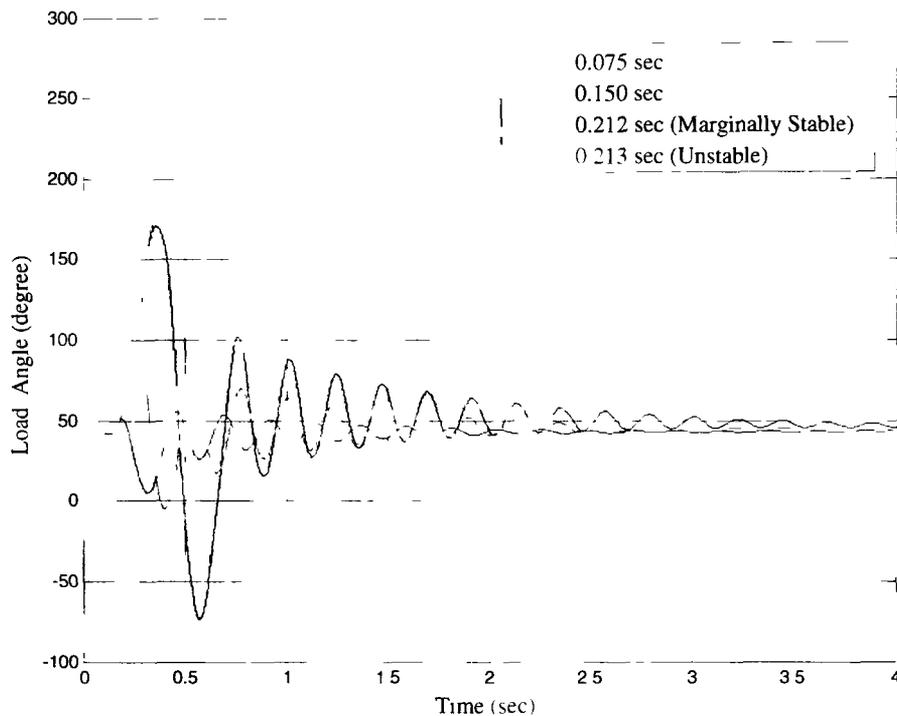
**Figure 4.23. Comparison of SC for 0.075 s, 0.150 s, 0.212 s (marginally stable) & 0.213sec (unstable).**
