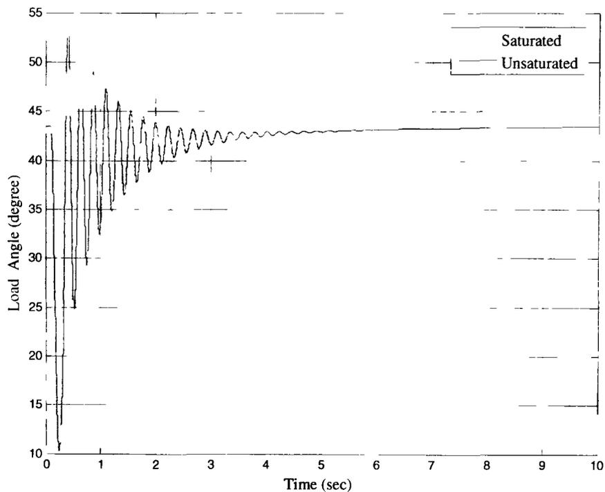
**Figure 4.16. 100% loss of DIT for 0.2 s.**
