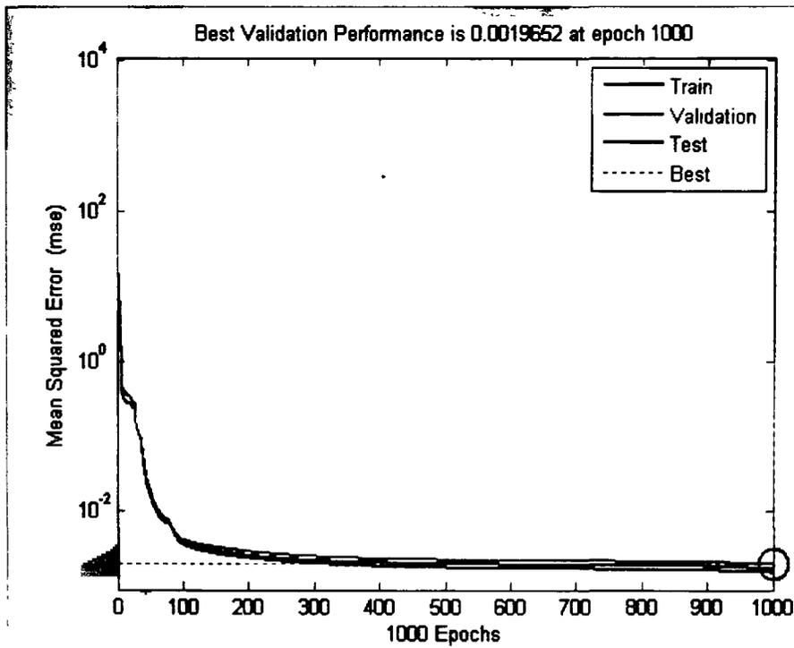
Figure 5.20. Error curve for 100% loss in DIT (0.1 s).
