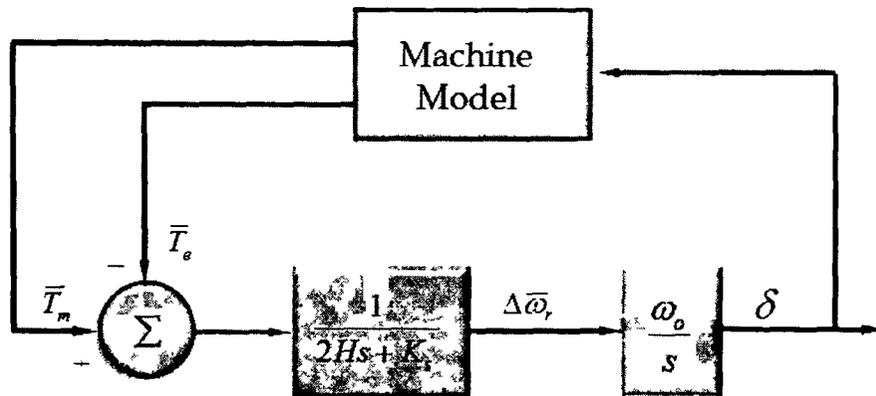
Figure 2.11. Internal control loop.
