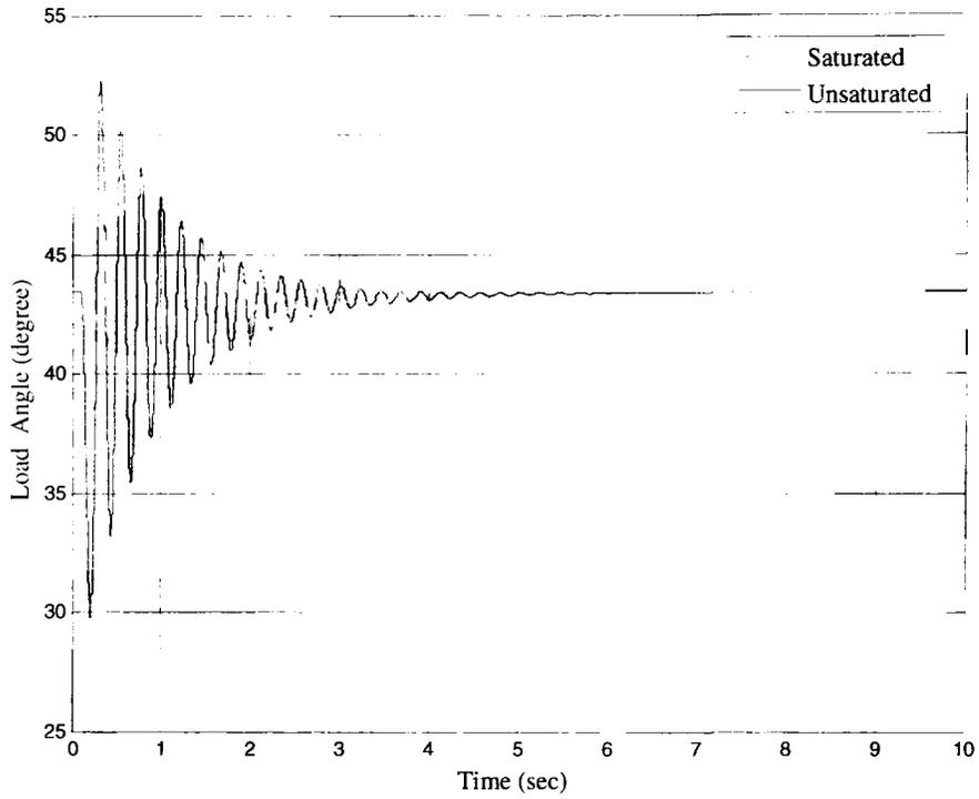
**Figure 4.12. 50% loss of DIT for 0.1 s.**
