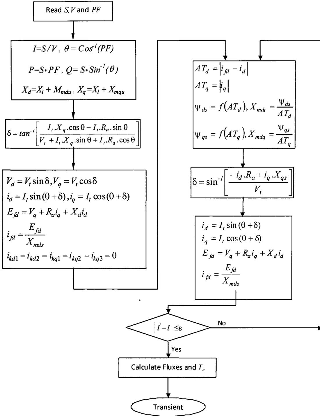
Figure 4.2. Initial value calculation flowchart for saturated model.
