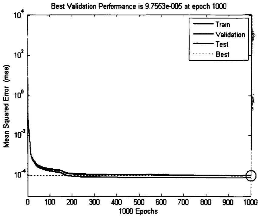
Figure 5.22. Error curve for 50% over-excitation in DIT (0.1 s).
