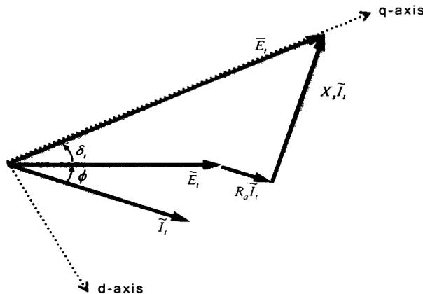
Figure 2.9. Phasor diagram for calculating initial conditions.
