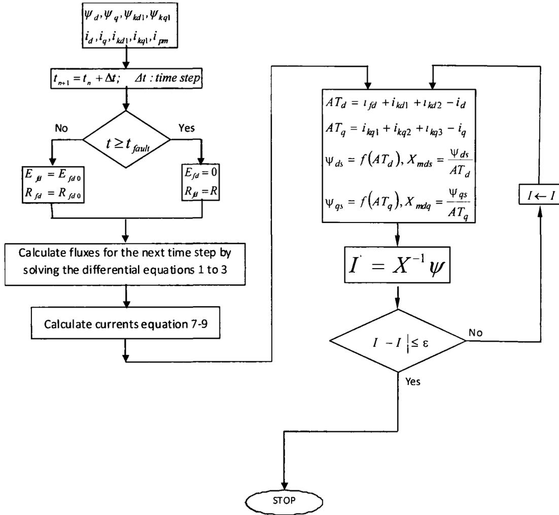
Figure 4.4. Calculation of transient values after LOF fault for saturated model.
