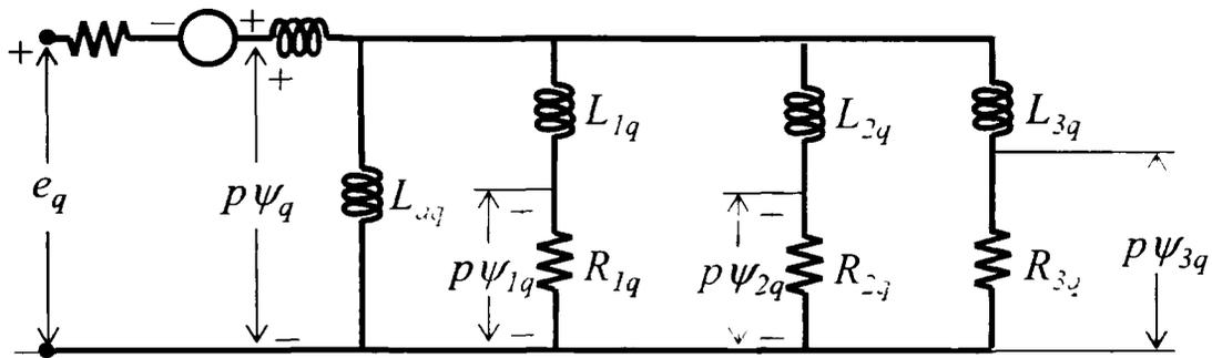
Figure 2.8. q-axis circuit diagram.
