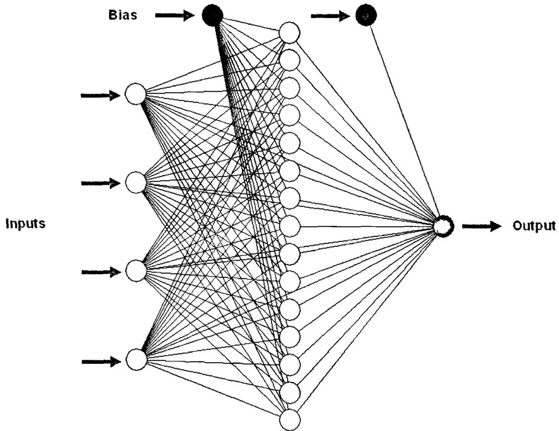
Figure 3.4. Feedforward neural network.
